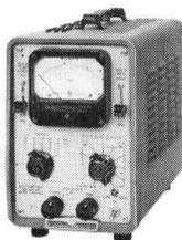
No computations! Provides instantaneous, automatic power readings *direct* in dbm or mw at all frequencies for which there are suitable bolometer mounts. For CW measurements, uses either 1/100 amp. fuse or Sperry 821 barretter. Also measures CW or pulsed power with negative coefficient thermistor. Provides up to 16
