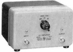
General-purpose transistorized instrument amplifier offering standard gains of 20 and 40 db,  $\pm 0.2$  db at 1000 cps. Distortion less than 1%, 10 cps to 100 KC. Frequency response  $\pm 0.5$  db 10 cps to 1 MC, output 1.5 v rms across 1500 ohms, noise 75  $\mu$ v rms, referred to input; input impedance 1 megohm with 20  $\mu$ mf shunt. Battery powered, 150 hours operation; or ac driven. Weight just 3 lbs. \$150.00. Specify battery or ac operation.
