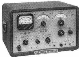
Completely transistorized, advanced instrument provides direct, accurate wave component measurement without calibration or stabilization. 20 cps to 50 KC, hum free, needs no warmup, very sharp acceptance circuits plus AFC. May be battery operated (18 to 28 volts). \$1,800.00△.
