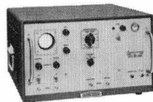
Stability of  $5/10^8$  is satisfactory in most applications formerly requiring primary standard. Multiple outputs include 6 sine and 4 pulse signals, plus timing comb. Includes
