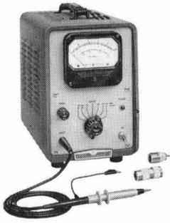
Millivolt sensitivity and two easy-reading linear voltage scales in 1-to-3 ratio make the all-new hp 411A perhaps the most widely useful voltmeter you have ever seen. Measure 10 mv to 10 v full scale, 500 KC to 1 KMC; get usable indications to 4 KMC! Db scale gives readings from -42 to +33 db for convenient gain measurements. Five probe tips
