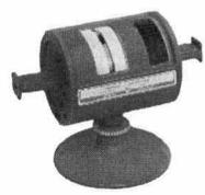
Previously offered for frequencies 3.95 through 18.0 KMC, popular hp 382A series precision attenuators are now available in "K" and "R" bands, 18.0 to 40.0 KMC. "K," "R" band attenuators are of new, space-saving design (see photo). Direct reading, one control tuning, high power handling capacity. Attenuation 0 to 50 db full range, independent of frequency. Phase shift constant with attenuation. For prices G, C, J, H, X, M and P382A, see table above. hp K382A, \$475.00. hp R382A, \$500.00.
