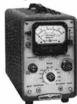
Directly measures frequency of voltages 3 cps to 100 KC; expanded scale allows any 10% or 30% of range to be measured full scale. Sensitivity 0.2 v rms, 1 v peak for pulses. Input impedance 1 megohm with 40 pf shunt. 500A calibrated in cps, 500C calibrated in rpm.
