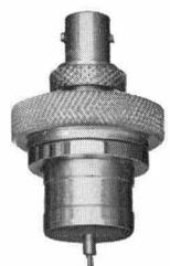
hp 444A is modified crystal (1N76 or 1N26) plus small antenna in convenient housing. Probe penetration easily variable; may be locked in position. No tuning needed; sensitivity superior to most elaborate single or double tuned probes. Range 3.0 to 18 KMC; fits 3/4" bore. New hp 446B, for hp 814 Probe Carriage, similar but covers K and R bands, 18.0 to 40.0 KMC. hp 444A, \$40.00. hp 446B, \$145.00.
