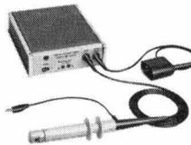
Permits measurement of current on indicating meters such as hp 400D, 400H, 400L (below) or hp oscilloscopes. New hp "current" probe clamps around wire under test, needs no physical connection, does not load circuit. Range 1 ma to 2 amps peak, accuracy  $\pm$  1% at 1 KC, response  $\pm$  2%, 100 cps to 3 MC,  $\pm$  5%, 60 cps to 4 MC, -3 db at greater than 20 MC. \$190.00.
