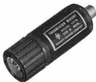
For frequency range 10 MC to 10 KMC. SWR less than 1.5. Thermistor element is 200 ohm negative. No tuning required; not susceptible to burnout. \$75.00 (including thermistor).
