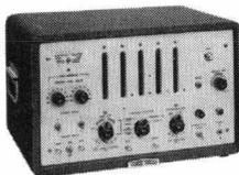
Compact, low cost, versatile instrument for frequency, period or time measurements. Measures frequency 10 cps to 120 KC, time interval 10  $\mu$ sec to  $10^6$  sec. Reads direct in cps, KC, seconds or milliseconds. Count automatically reset, action repetitive. Stability of time base  $1/100,000$ /week. \$915.00 △.
