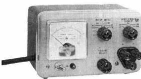
New, completely transistorized, compact, regulated supply. Output 0 to 30 v, continuously variable. 150 ma maximum output, output impedance less than 0.2 ohms. Regulation, no load to full load, 0.3% or 30 mv whichever is greater. Line voltage change of  $\pm 10\%$  causes output change of less than 0.3% or  $\pm 15$  mv, whichever is greater. Front panel switch limits maximum output current preventing damage to transistors, etc., from accidental overload. Reads ma, v direct. \$145.00.
