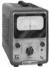
High sensitivity, high stability microvolt meter reading end scale voltages of 10  $\mu$ v to 1 v in 11 ranges. Also reads currents of 10  $\mu$ a to 3 ma in 18 steps, 1-3-10 sequence. Accuracy  $\pm$  3% on all ranges. Drift is less than 4  $\mu$ v per day referred to input terminals. Input impedance 1 megohm  $\pm$  3% on all voltage
