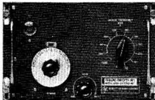
**-hp- 526A Video Amplifier.** This equipment increases the Counter's 10 cps-to-10 MC sensitivity to 10 millivolts for frequency measurement at low power levels. A special probe assembly simplifies remote pickup at high impedance levels. An oscilloscope output terminal enables monitoring at the input waveform visually.
