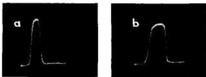
**Figure 1.** (a) 0.01  $\mu$ sec pulse through *-hp- 460B* Amplifier. (b) 0.02  $\mu$ sec pulse through 3 amplifiers in cascade.
