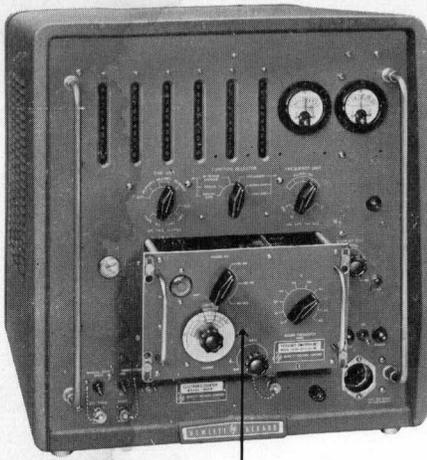
**-hp- 524B COUNTER WITH -hp- 525A FREQUENCY CONVERTER**
