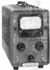
No computations! Provides instantaneous, automatic power readings *direct* in dbm or mw at all frequencies for which there are suitable bolometer mounts. For CW measurements, uses either 1/100 amp. fuse or Sperry 821 barretter. Also measures CW or pulsed power with negative coefficient thermistor. Provides up to 16 ma bias current. Operates with all mounts in adjacent table. \$250.00.
