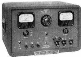
This new **-hp-** instrument features high regulation of 0.01%, 0.1 millisecond transient response, internal impedance 0.1 ohms in series with 25  $\mu$ H; full-load maximum hum less than 500  $\mu$ v, sealed transformers, chokes and condensers. 0 to 500 v, 200 ma supply and fixed —300 v tap providing a 50 ma, 300 to 800 v variable supply for klystron operation. \$365.00 $\Delta$ .
