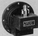
For fast, accurate waveguide power measurements. Each mount covers full range of its waveguide frequency. No tuning required, SWR less than 1.5. Rugged construction, high temperature coefficient permanent thermistors virtually eliminate delays due to detector element burn-out.
