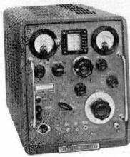
10 to 420 mc. Highest stability. No incidental fm or frequency drift. Calibrated output 0.1  $\mu$ v to 0.5 v throughout range. Built-in crystal calibrator provides frequency check accurate within 0.01% each 5 mc. Master-oscillator, intermediate and output amplifier circuit design. Premium quality
