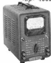
Best *-hp-* voltmeter ever built! Covers all frequencies 10 cps to 4 mc. Extremely sensitive, wide range, accurate within 2% to 1 mc, measures 0.1 mv to 300 v. Direct reading in dbm. 10 meg-ohm input impedance insures negligible loading on circuits under test. New amplifier circuit with 56 db mid-range feedback assures utmost stability, freedom from change due to external conditions. \$225.00.
