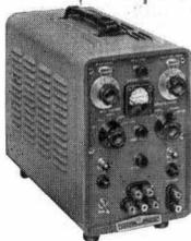
**-hp- 715A** is a versatile source of regulated beam and reflector voltage for operating most test bench klystron tubes. Beam voltage 250 to 400 v; reflector voltage 0 to 900 v; 6.3 v filament. Internal, 1,000 cps square wave modulation, also 60 cps fm modulation, both on reflector voltage. \$300.00.
