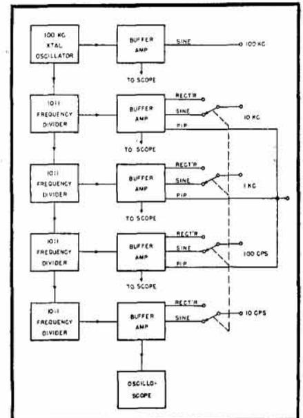
Fig. 1. Block diagram of circuit, Model 100D.
