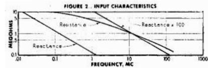
**Input Impedance:** Input capacity is 1.3  $\mu\text{f}$ d; input resistance is 10 megohms at low frequencies. At high frequencies resistance drops off due to dielectric losses. (See Fig. 3.) Dc input resistance is 100 megohms for all ranges.
