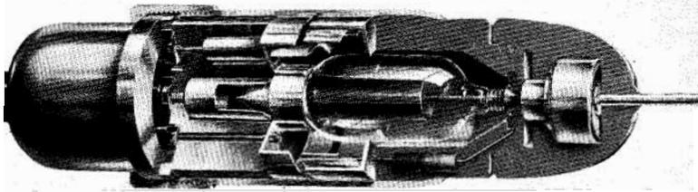
Figure 1. Construction details of new *-hp-* diode probe
