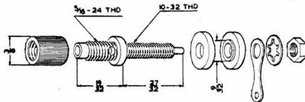
of the post, a feature which eliminates excessive contact resistance. The cross-hole for permanent connection can be used even when the "Banana" plug is inserted. The screw thread will not damage the thread. The long, axially-knurled ferrule is 10-32 and the tip is undercut so that a soldered connection provides a wide surface for ease of handling.
