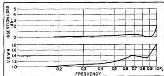
Fig. 2. Typical band pass characteristics.
