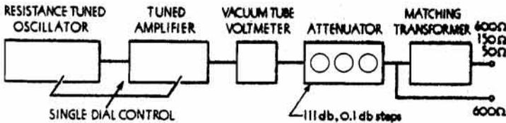
A single ended 600 ohm output is provided which bypasses the line-matching transformer. This output connection results in superior distortion and frequency response characteristics.
