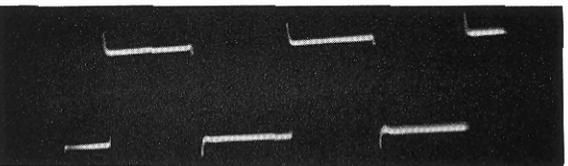
Attenuator leakage at high frequencies shows up in this oscillogram.
