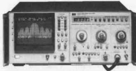
There is a potential personnel and equipment shock hazard in Analyzers with serial numbers 2128A00340 and below. When a new CRT (5083-6176) is installed in these units, approximately 2500 volts is applied via CRT pin 13 (deleted on older CRT's) through the CRT cable assembly and the
