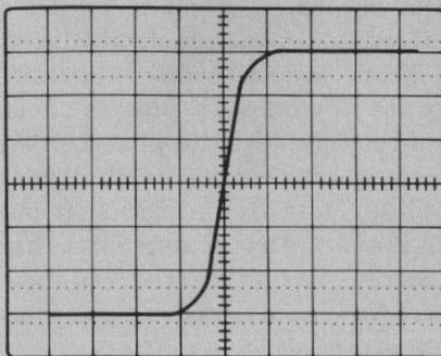
Use DELAY control to center leading edge of pulse over center horizontal graticule.
