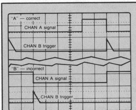
**Figure 3. Trigger example showing time relationship between signal connected to CHAN A and its trigger connected to CHAN B.**
