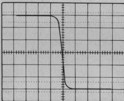
Use DELAY control to center trailing edge of pulse over center horizontal graticule.
