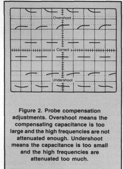
**Figure 2. Probe compensation adjustments. Overshoot means the compensating capacitance is too large and the high frequencies are not attenuated enough. Undershoot means the capacitance is too small and the high frequencies are attenuated too much.**
