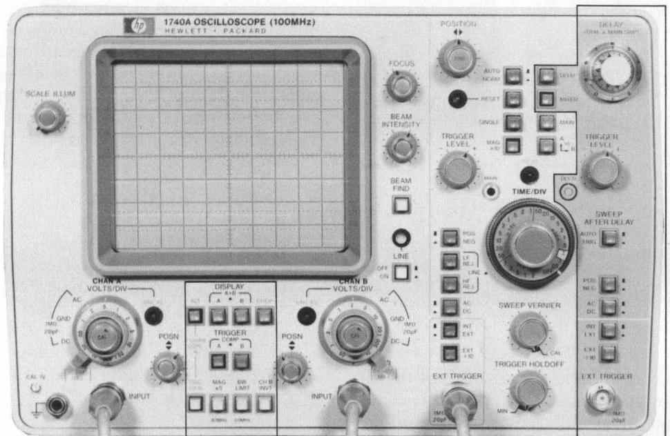
Main display and trigger controls. These pushbuttons determine which channel will be displayed, A, B, or both; Alternate or Chop mode, and which input will trigger the sweep.
