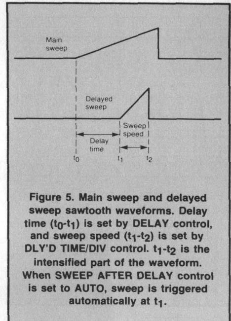
other mode, the delayed sweep is armed at the end of the delay period and requires a trigger signal (either internal or external) to start the delayed sweep. Since there is no way to know when the trigger signal will occur, the delay time is uncalibrated.
