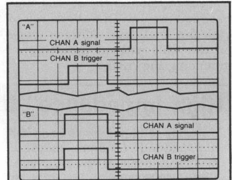
**Figure 4. Composite trigger example showing how to compare two asynchronous signals connected to CHAN A and CHAN B.**
