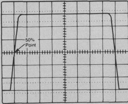
Figure 6. Pulse width measurement using the delayed sweep controls.
