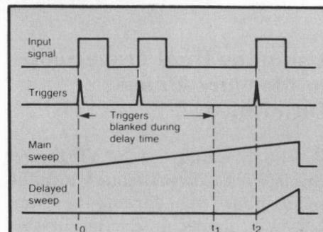
**Figure 8. Delayed sweep delayed trigger example.** The main sweep is started by the first trigger pulse at  $t_0$ . The second trigger pulse "arms" the delayed sweep at  $t_1$ . The next trigger pulse to arrive after the delay time ends starts the delayed sweep sawtooth at  $t_2$ . The time between  $t_1$  and  $t_2$  is unknown which makes the delayed sweep uncalibrated.
