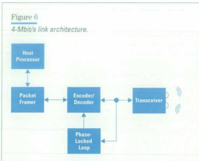
framer, ENDEC, and phase-locked loop are more complex than the UART and ENDEC in the 2400-to-115,200 bit/s link. However, this added complexity need not be expensive. The components are specified in a hardware description language and can be added quickly and inexpensively to one of the host system's ASICs. PC chipsets including the 4-Mbit/s hardware are already available from leading semiconductor manufacturers.
