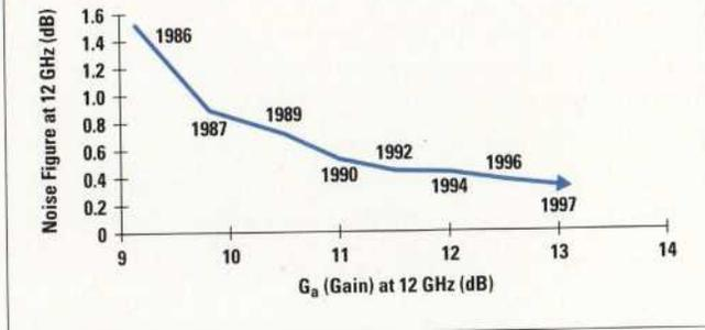
the noise figure improves the carrier-to-noise ratio for a given size of dish antenna, while still maintaining the signal quality. Therefore, the history of developing low-noise block downconverters is the same as improving the noise figure of GaAs transistors.
