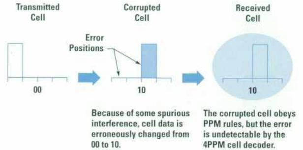
the same way that a sufficient number of carefully positioned errors can produce a correct-looking CRC for a corrupted packet, there are some error patterns that a 4PPM decoder cannot detect. An example is shown in **Figure 10**.
