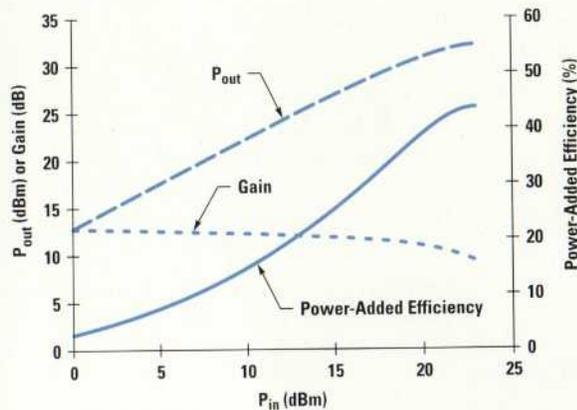
these measurements were the same as for the preceding gain, power, and efficiency tests. A 0.8-dB correction has been applied to account for the measured output circuit matching loss.
