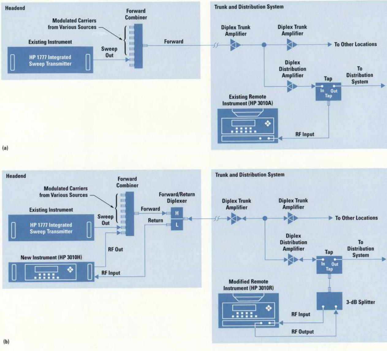
At the beginning of the project, the required hardware changes to the original HP 3010A block diagram (see Figure 6) were not readily obvious. We considered several schemes for the sweep source portion of the new remote unit. We finally settled on an approach that is based upon a tracking generator concept used in most spectrum analyzers. In a spectrum analyzer, a tracking generator is implemented by operating the RF conversion in reverse. That is, instead of converting a broad input
