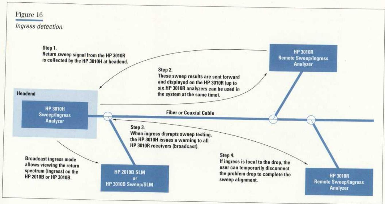
The forward pilot is a frequency that is set aside in the cable spectrum for communication. The HP 3010R uses a forward and return pilot to complete the communication loop.
