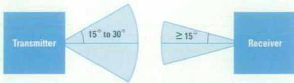
range of up to one meter with a viewing half-angle of between 15 and 30 degrees (see **Figure 1**). More recently, IrDA has extended the physical layer specification to allow data communications at transfer rates up to 4 Mbits/s.
