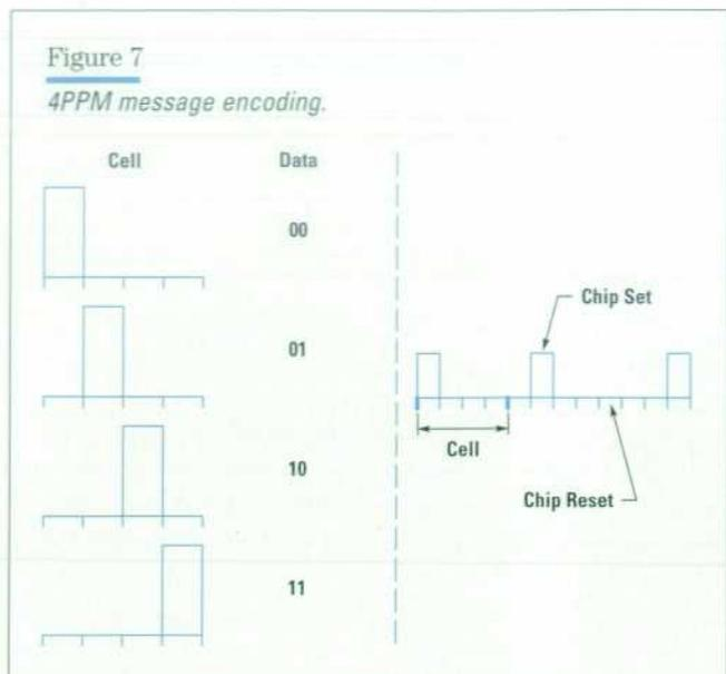
format that has very little dc content and can be high-pass filtered at 100 kHz, avoiding interference generated by fluorescent lighting without adversely affecting the receiver's eye diagram. A particularly interesting feature of PPM—one that had important ramifications in the choice of end delimiters—is its ability to detect line code errors.
