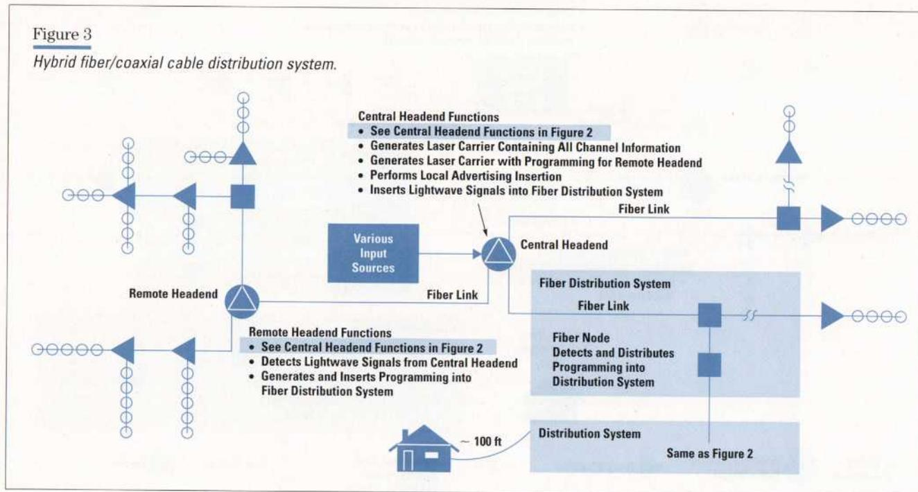
The advantages of using hybrid fiber/coaxial systems include significantly lower vulnerability to amplifier outages, reduced bandwidth restrictions, lower noise buildup (because fewer amplifiers are in series), and greatly reduced ingress. The greatly reduced ingress makes a two-way system practical. Another major benefit of the fiber backbone approach is that implementation cost is relatively low.
