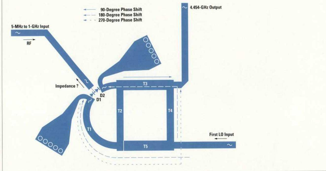
This multiplication performed in the time domain results in a translation in the frequency domain and the net result is the sum and difference of the RF and first LO frequencies. More specifically, if the input frequency is  $f_{rf}$  and the first LO frequency is  $f_{lo}$ , mixing produces two new frequencies:  $f_{hi} = (f_{lo} + f_{rf})$  and  $f_{low} = (f_{lo} - f_{rf})$ . In our case we are interested in the  $f_{hi}$  so we simply filter the  $f_{low}$  with the first IF bandpass filter.
