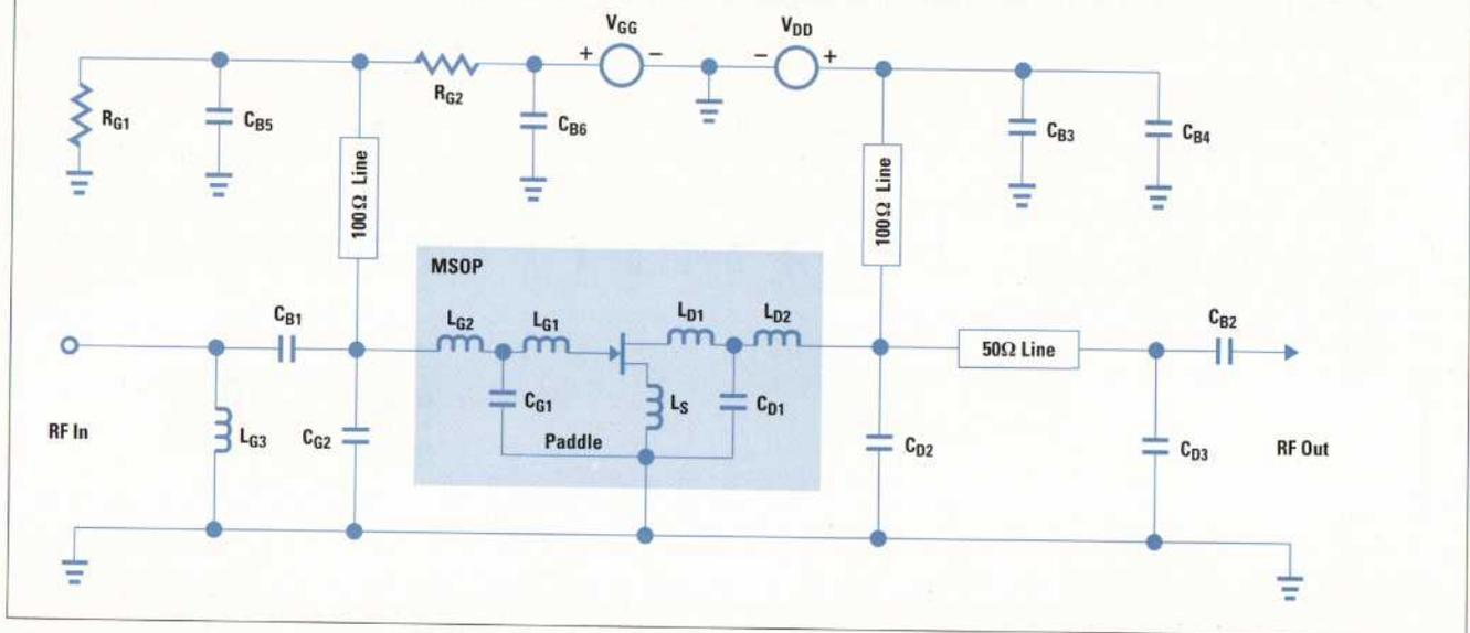
(see Figure 14) provides pi-section matching networks on both the input and output to achieve these goals, along with quarter-wavelength transmission line networks for gate and drain biasing.
