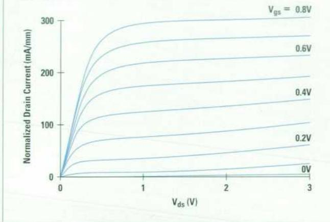
2 mA/mm, is 0 volts. The knee voltage, defined as the drain-source bias when the drain-source current density becomes 200 mA/mm with  $V_{gs}$  equal to 0.8 volt, is 0.3 volt. The on-resistance, measured at  $V_{gs} = 0.8$  volt, is 1.5 ohms-mm.
