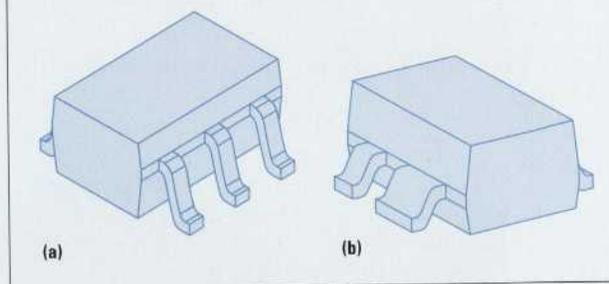
This package is used for a wide range of RF products. The SOT-343 package was developed specifically for high-frequency, low-noise transistors. The leadframe design, lead-forming profile, and molding-compound selection were optimized to improve the high-frequency performance of the package. The noise contribution of the SOT-343 package at 12 GHz is only half that of the SOT-363 package.
