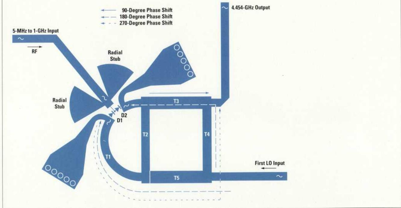
changes other than scaling the line widths and lengths. However, because the second LO is loaded by the second mixer and dielectric resonator, the line lengths become critical (see **Figure 12**).
