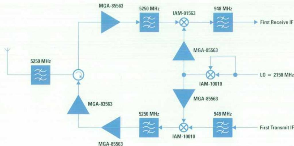
a number of highly integrated GSM receiver RFICs available, and these could be leveraged to minimize design effort. Also, a variety of transmit solutions are possible, including, for example, the HPMX-2007 vector modulator and upconverter.
