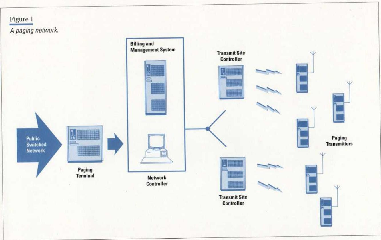
then transmit the batch of pages at the same time on the same frequency using a simulcast technique. Simulcast means that two or more transmitters are used to transmit identical information at the same time. This allows the system to provide seamless coverage on a single frequency.
