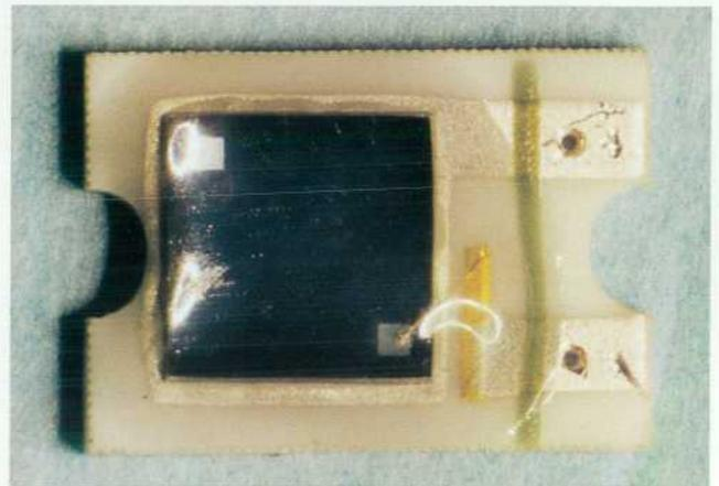
**Fig. 19.** Photodiode receiver.
