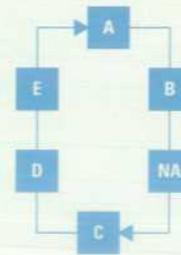
Fig. 5. The primary ring of an FDDI network.
