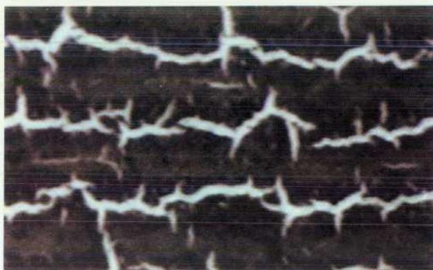
**Fig. 7.** Imaged film with cracked coating in the print area.
