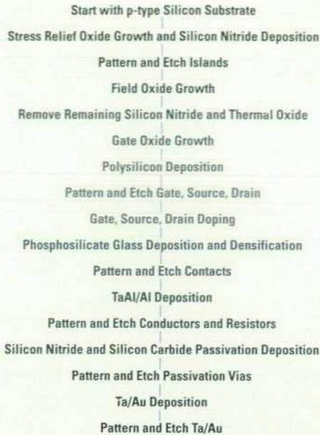
Fig. 5. Integrated driver printhead process flow.
