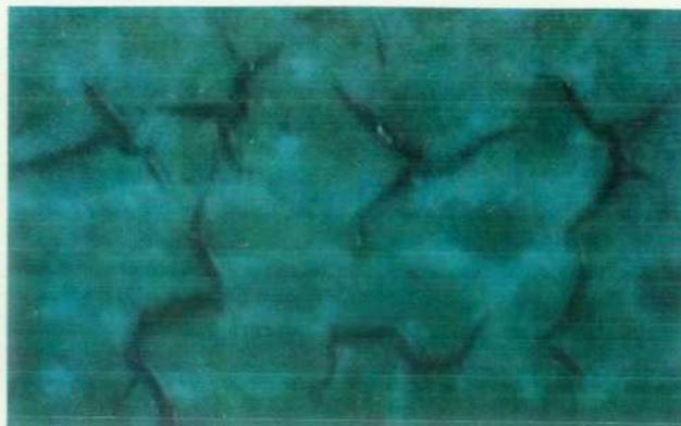
**Fig. 6.** Imaged film with wrinkles in the print area.
