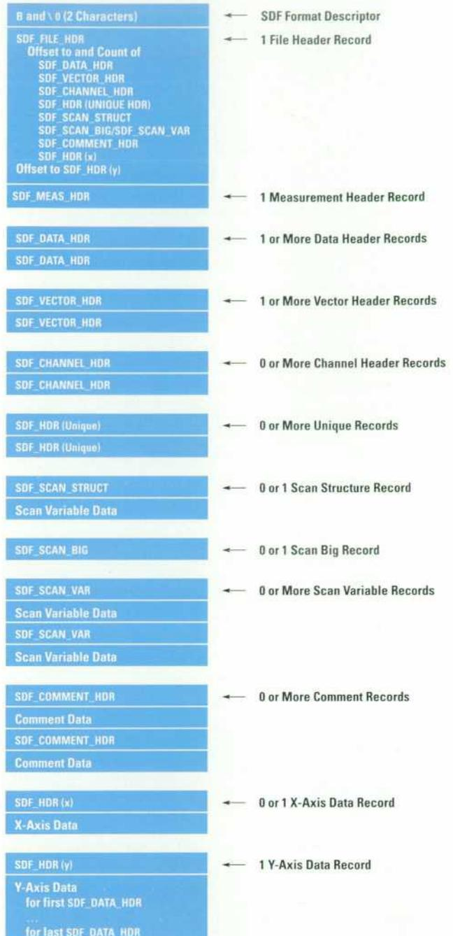
Fig. 3. Standard Data Format file structure.
