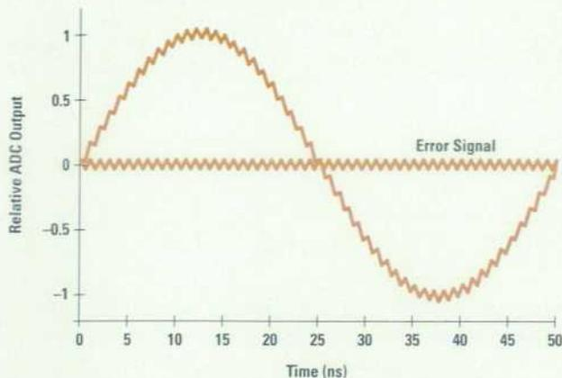
**Fig. 2.** The output produced by a system of two interleaved ADCs with an offset error between them is the original signal plus an error signal at the individual ADC sampling frequency, or half the interleaved sampling frequency.
