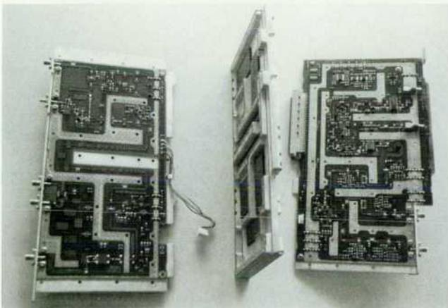
**Fig. 12.** Two RF circuit boards and the molded aluminum block.
