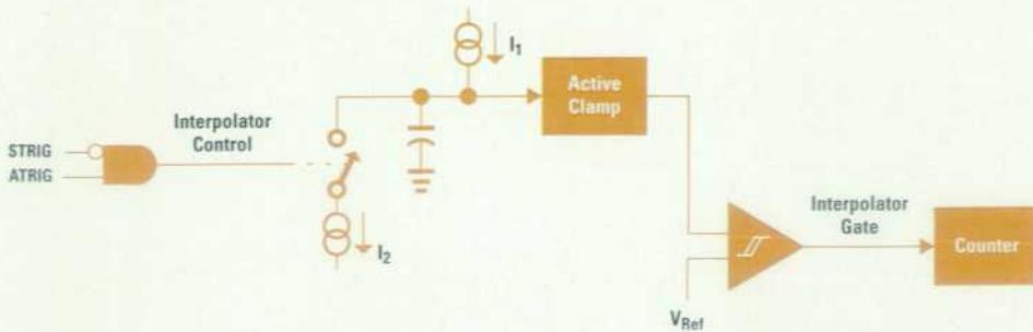
Fig. 7. Functional block diagram of the dual-slope trigger interpolator.
