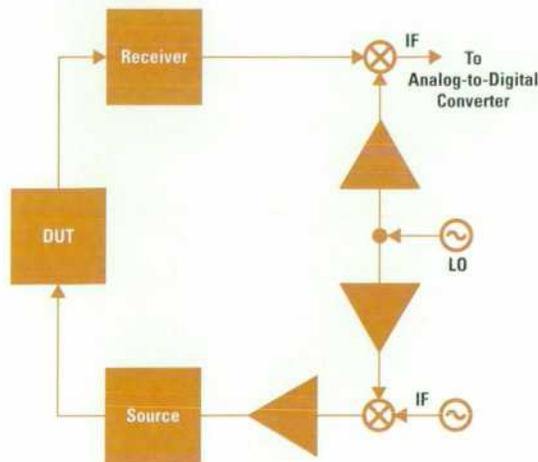
**Fig. 1.** A measurement setup in which the source to the DUT and the receiver are in the same network analyzer. The receiver of the network analyzer is easily tuned to the same frequency as the source.
