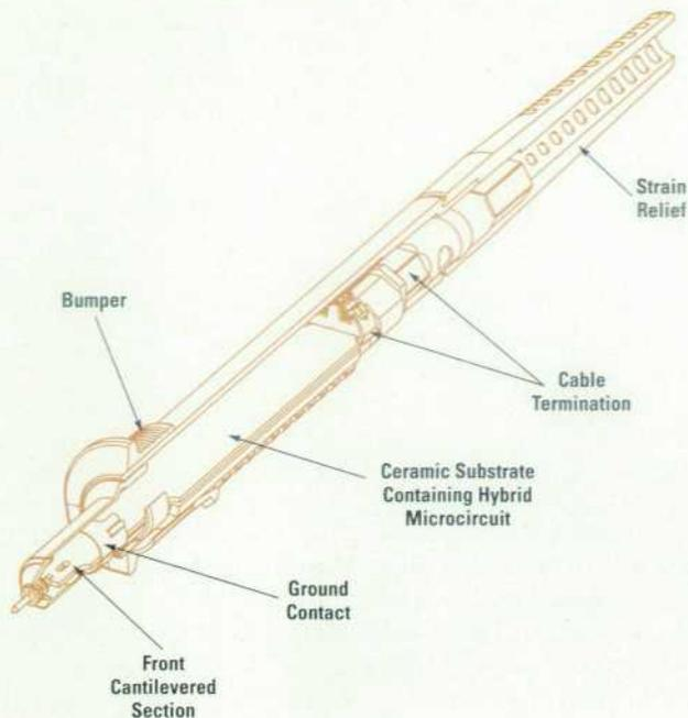
Fig. 3. Cutaway view of the active probe.
