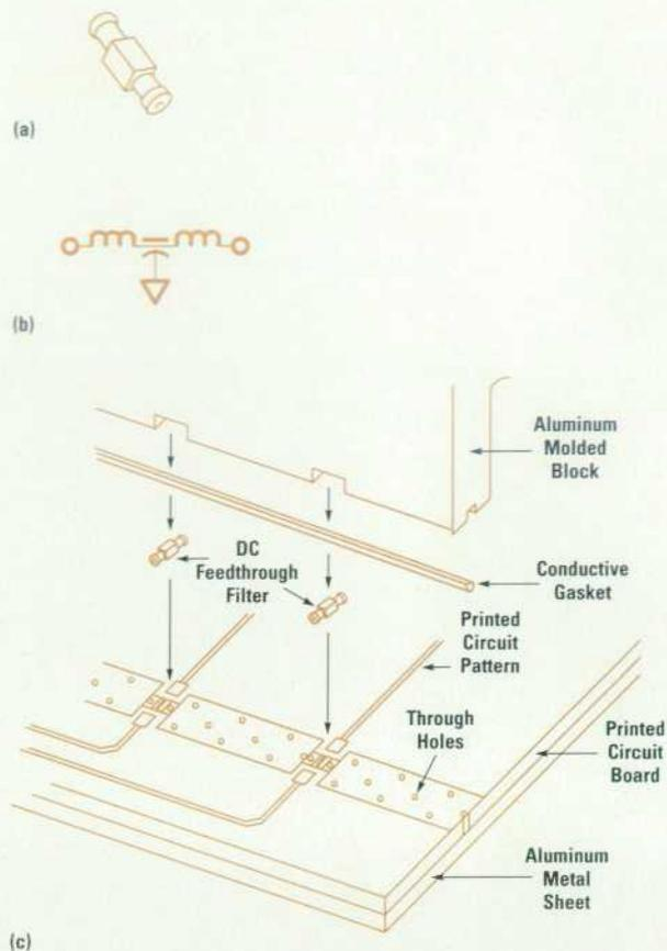
**Fig. 13.** Dc feedthrough on an HP 4396A RF module uses a surface mount dc feedthrough filter. This method contributes to cost reduction, productivity, and serviceability without degrading the shielding performance. (a) Feedthrough component. (b) Equivalent circuit. (c) Implementation.
