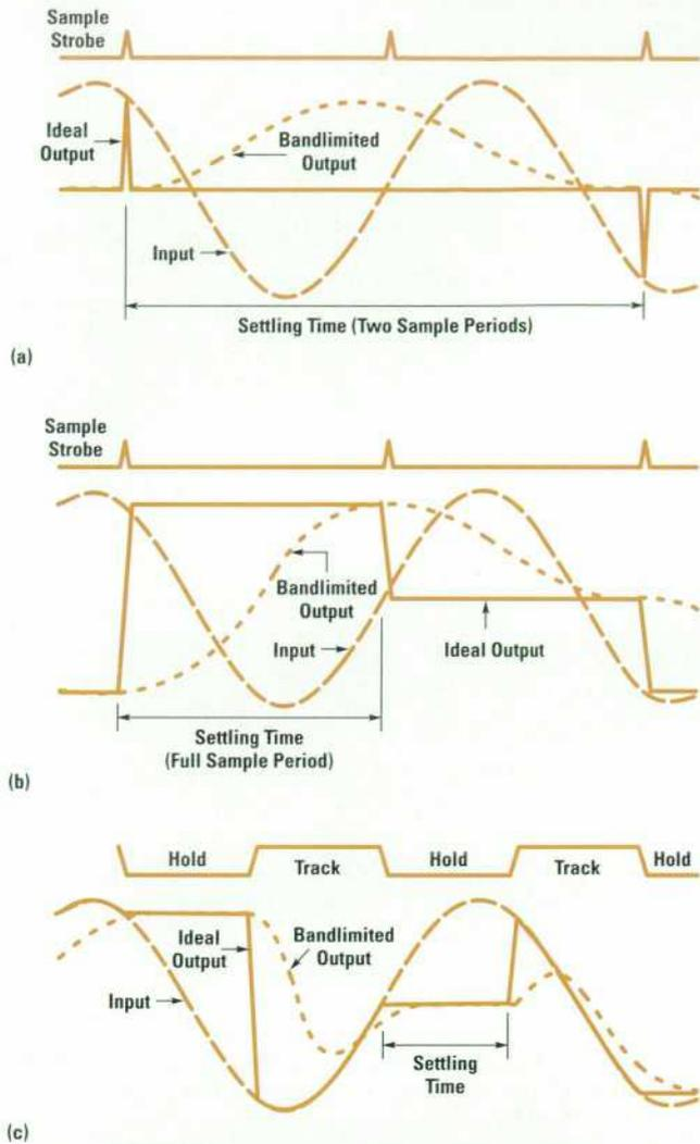
**Fig. 11.** The sample-and-filter technique compared with sample-and-hold and track-and-hold, showing IF bandwidth and settling time comparisons. (a) Sample-and-filter. Required bandwidth =  $\frac{1}{2}$  sample rate. (b) Sample-and-hold. Required BW = sample rate. (c) Track-and-hold. Required BW =  $2 \times$  sample rate.
