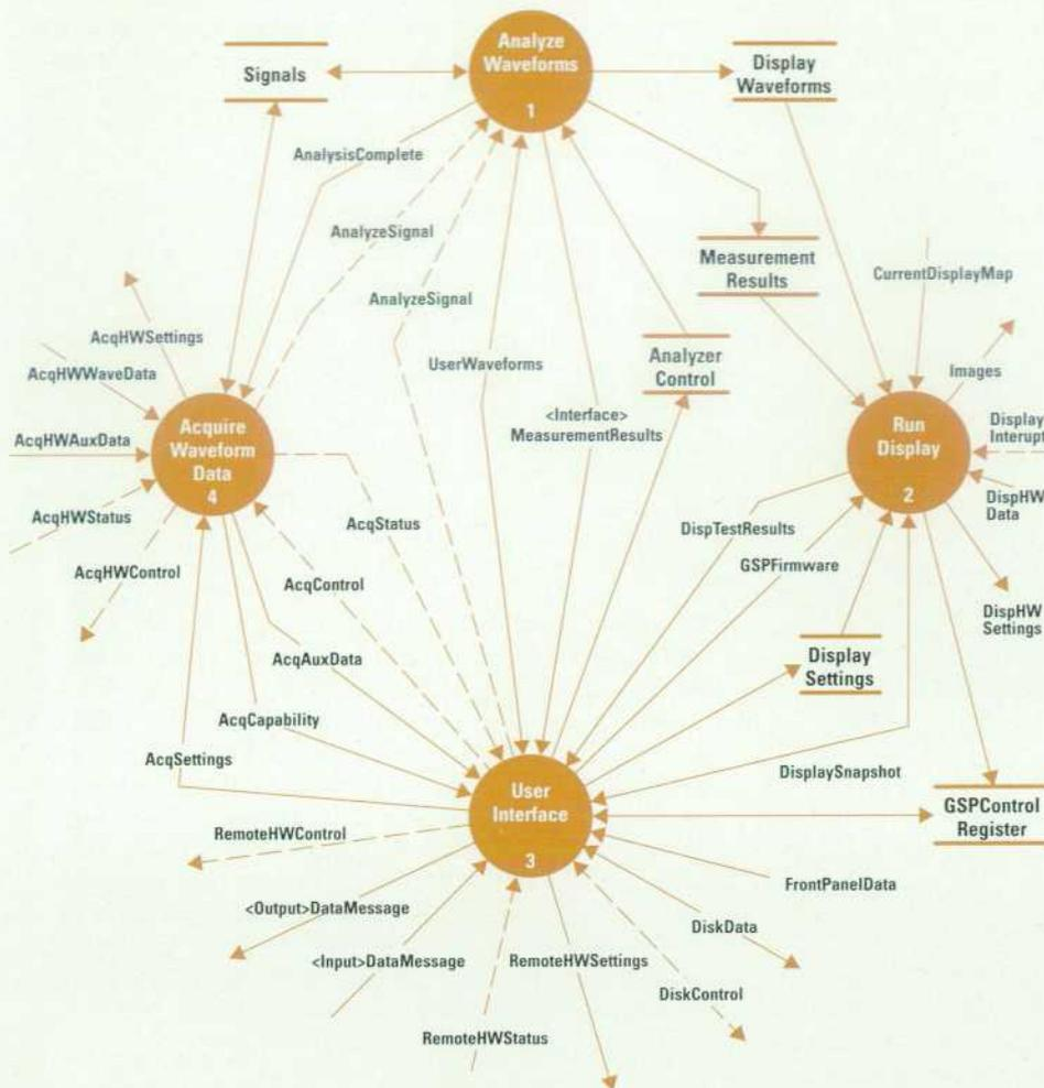
Fig. 1. Top-level data flow diagram for the HP 54720/10.
