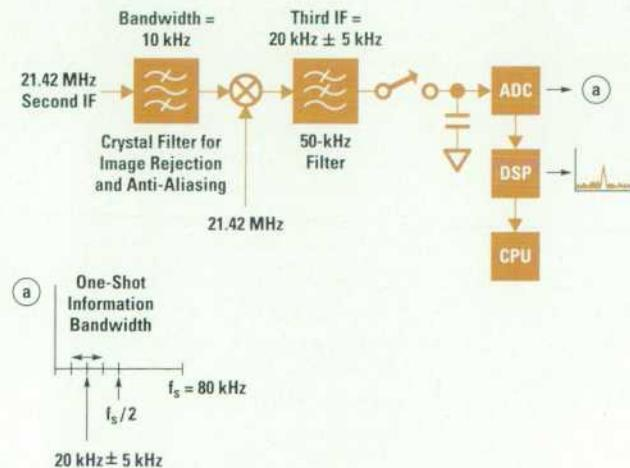
**Fig. 8.** Components involved in providing the FFT mode for spectrum analysis with narrower RBWs. The effective information bandwidth in this mode is 15 to 25 kHz. The DSP chip does the decimation and the FFT calculation.
