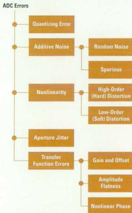
Fig. 1. Outline of analog-to-digital converter (ADC) errors.
