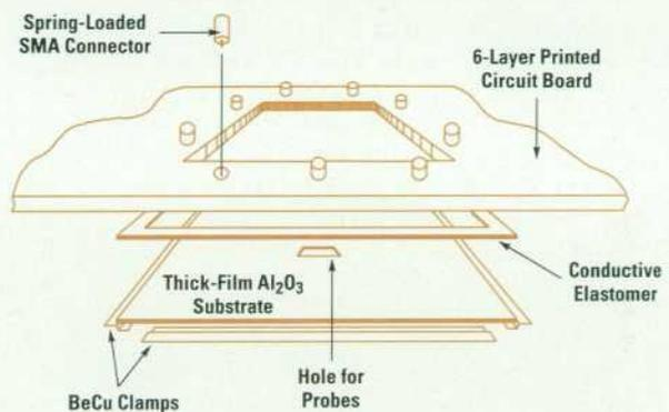
Fig. 1. Simplified perspective view of the new probe fixture.
