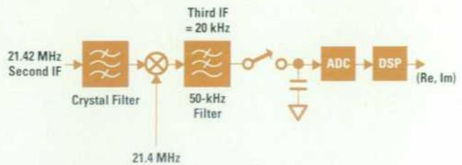
**Fig. 9.** Components involved in providing the ac sampling mode for network analysis. The 20-kHz IF is sampled and held at 80 kHz. The vector information is generated by the DSP chip, and the CPU receives the real and imaginary components of the IF signal.
