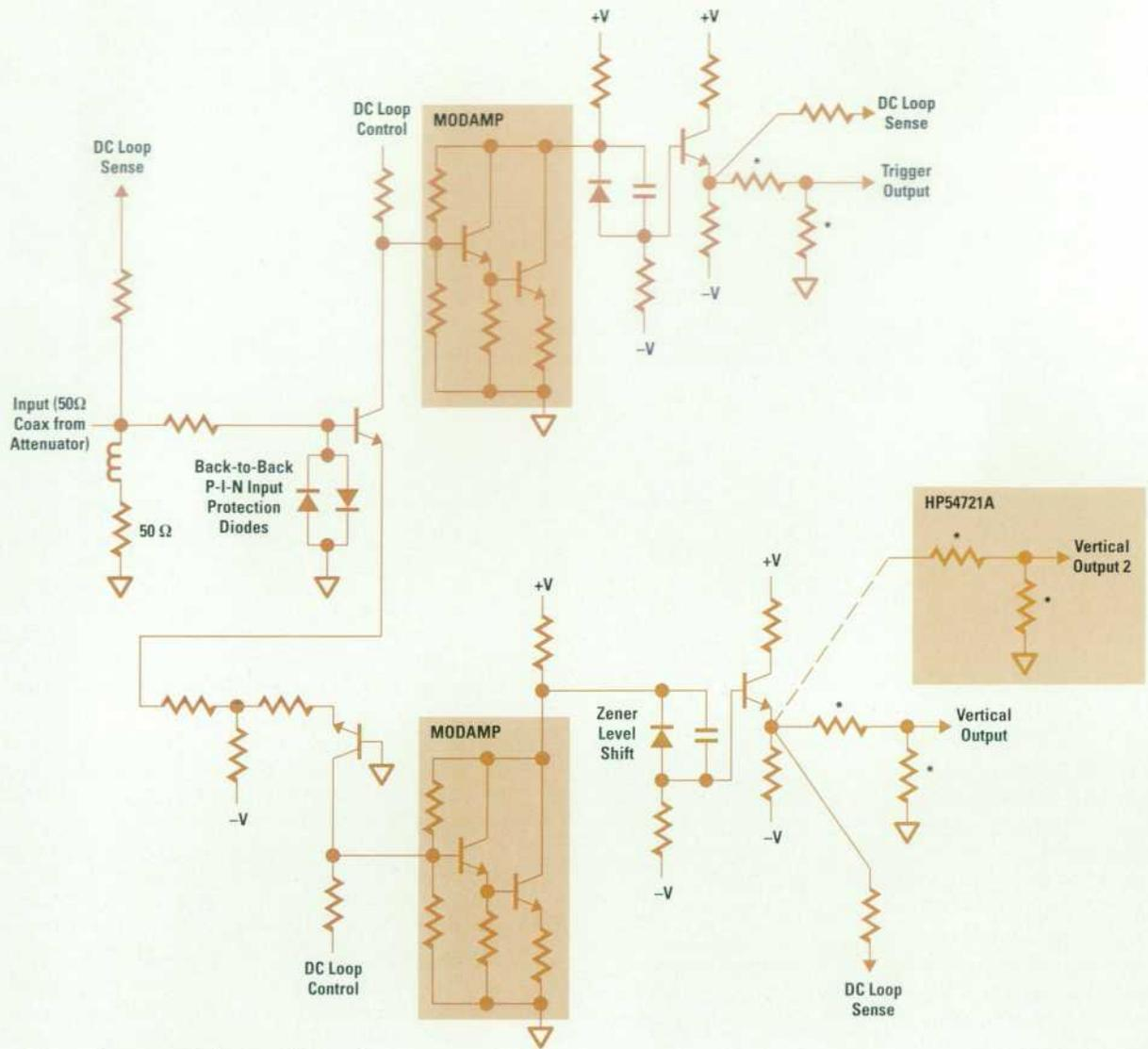
\* These resistors are actively trimmed (by lasers) to set the gain and source terminations.
