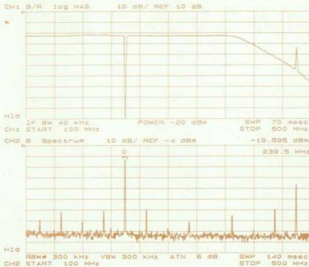
**Fig. 2.** The upper channel shows a network measurement in which the gain of an amplifier is being measured. The lower channel shows the spectrum of the signal being monitored at the output of the same amplifier. Without changing any connections, spurious signals that corrupt the amplifier gain measurement can be found by means of the spectrum monitor.
