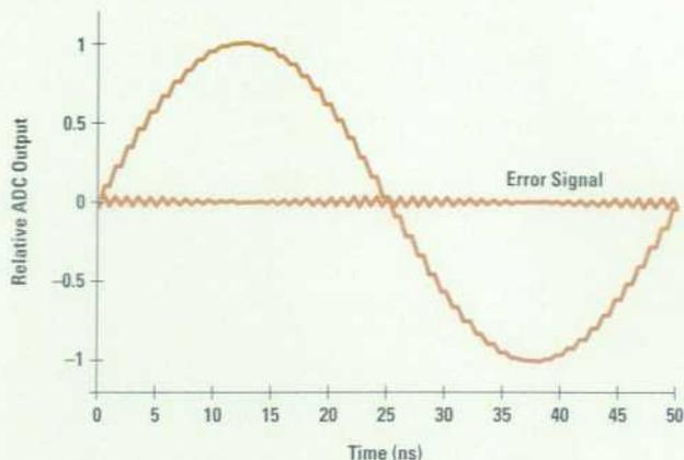
**Fig. 4.** Output from a system of two interleaved ADCs with a timing offset between them includes an error signal at the individual ADC sampling frequency, or one half the combined sampling frequency. The carrier is amplitude modulated by the derivative of the original signal. The error is maximum on the slewing portion of the waveform.
