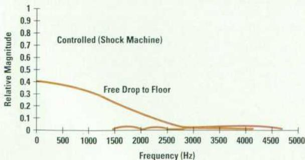
Fig. 7. Spectra of controlled and estimated uncontrolled shocks.
