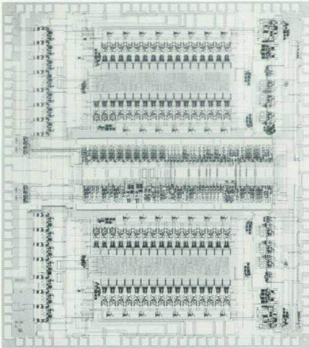
Fig. 6. Dual 500-MSa/s 8-bit bipolar flash ADC chip.
