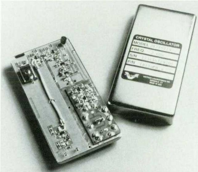
Fig. 13. Clock oscillator.
