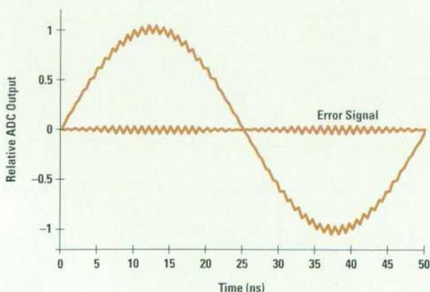
**Fig. 3.** A system of two interleaved ADCs with a gain error between them introduces an error signal that consists of a carrier at the individual sampling frequency that is amplitude modulated by the original signal.
