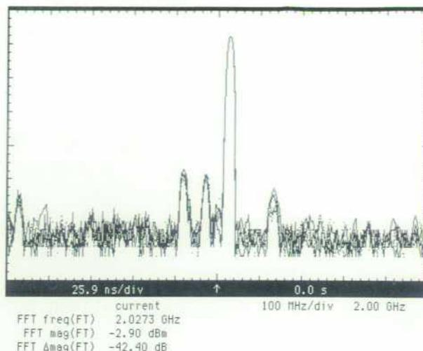
Fig. 24. FFT of the 2-GHz reconstructed sine wave of Fig. 20, showing sidebands down 42 dB from the fundamental.
