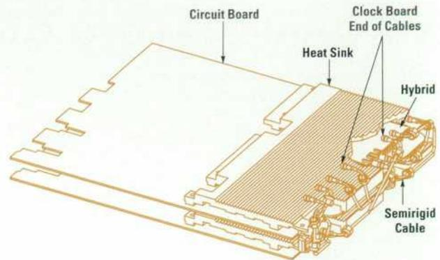
**Fig. 8.** Acquisition assembly with one heat sink partially cut away to show the thick-film hybrid circuit. Semirigid cables attach directly to the hybrids.
