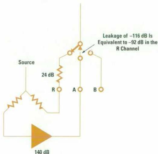
**Fig. 9.** Measurement of a high-gain amplifier (140 dB). The leakage through the A channel is 48 dB larger than the desired R-channel signal. Thus, the amplifier cannot be measured correctly because of the extra pad at the R channel.
