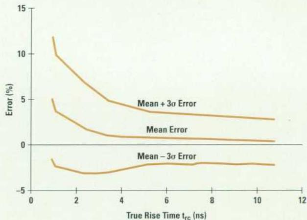
**Fig. 1.** HP 54720A oscilloscope single-shot step rise time error at 4 GSa/s. For the first time bias and variation in indicated 10%-to-90% rise time measurements made by faster real-time oscilloscopes like the HP 54720A can be measured. ( $t_{rc}$  is the true rise time as measured by an HP 54124T.)
