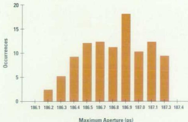
Fig. 6. Sample maximum aperture measurement repeatability histogram.
