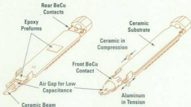
Fig. 9. Method of prestressing the substrate using epoxy.
