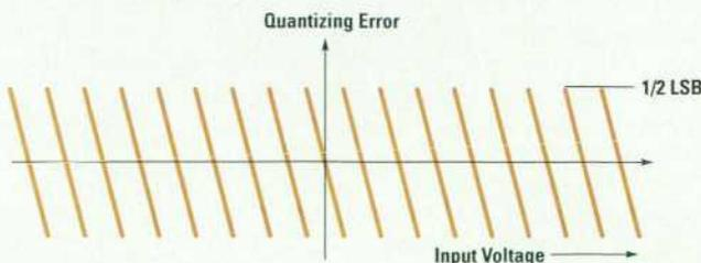
Fig. 8. Quantizing error for an ideal ADC.
