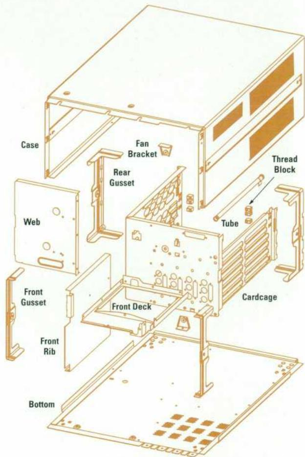
**Fig. 4.** Nineteen parts are welded by the supplier to complete a cabinet ready to accept circuit boards and other components. The vertical plane of sheet metal at the center of the drawing is the bulkhead, which establishes the z location of the plug-ins.
