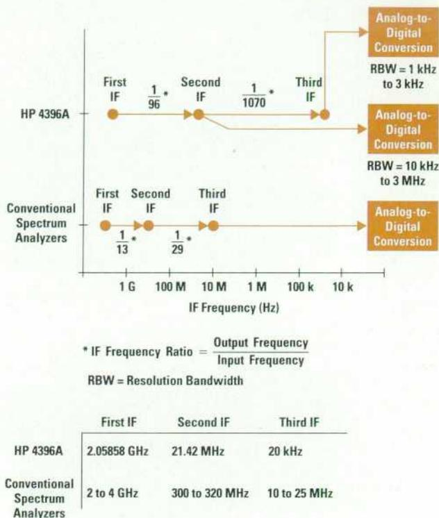
Fig. 10. IF frequency ratios of the HP 4396A compared to conventional spectrum analyzers.
