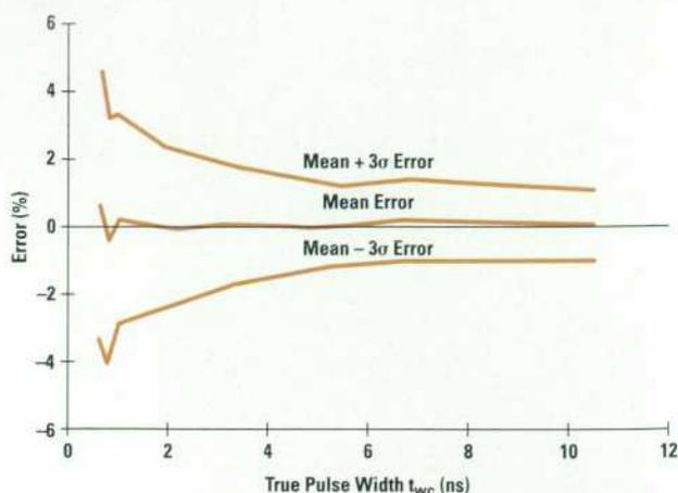
**Fig. 4.** HP 54720A bias-corrected impulse width error at 4 GSa/s. Bias correction equations using exponential terms can correct the HP 54720A's Gaussian pulse mean measurement accuracy to better than 0.5% and  $3\sigma$  accuracy to better than 4% for most pulses.
