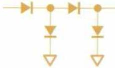
**Fig. 6.** Series-shunt type diode switch. This circuit provides less isolation efficiency.
