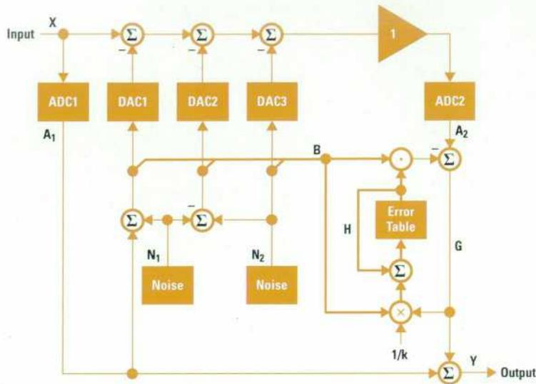
Fig. 14. DAC calibrator block diagram.
