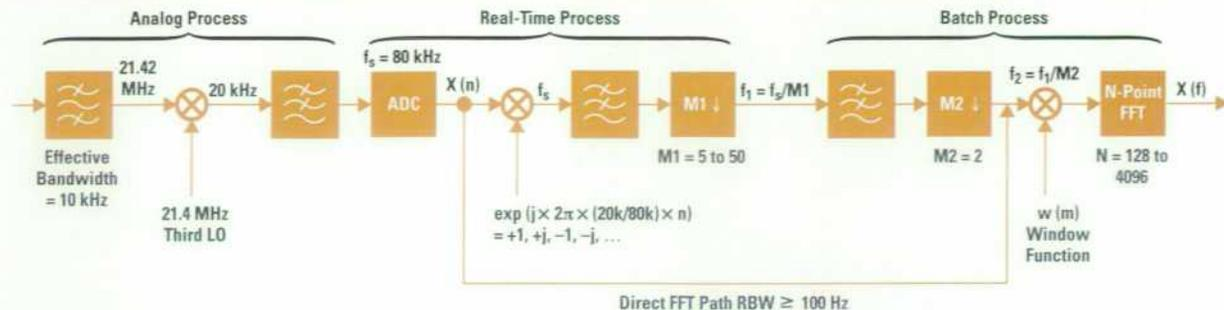
Fig. 2. HP 4396A signal processing block diagram.
