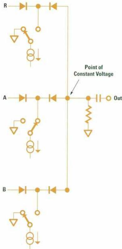
**Fig. 11.** The p-i-n diode switches of the multiplexer are driven by switched current sources. All the switches have been designed to switch simultaneously to reduce switching transients. Remember that there are six diodes per channel. Therefore, each diode in the schematic represents three diodes.
