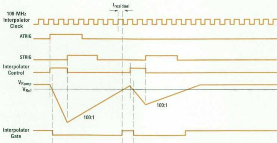
Fig. 10. Waveforms in the residual dual-slope interpolator.
