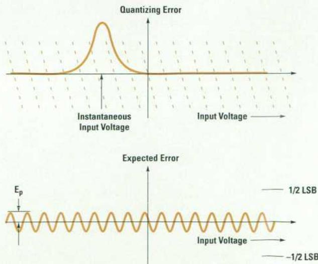
Fig. 10. Adding noise to reduce nonlinearity error.
