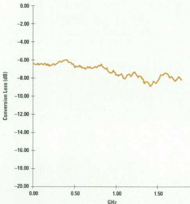
Fig. 2. Conversion loss of the double-balanced first mixer and the input low-pass filter. The double-balanced mixer design reduces the conversion loss and consequently increases the sensitivity (lowers the noise floor) of the HP 4396A.
