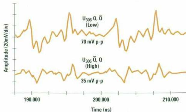
Fig. 5. Clock-to-output coupling on nonswitching outputs is higher on low outputs (top trace) than on high outputs.
