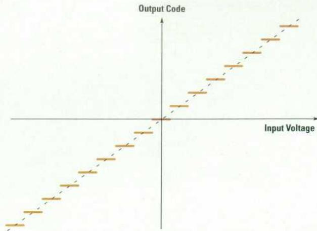
Fig. 7. Ideal quantizer transfer function.
