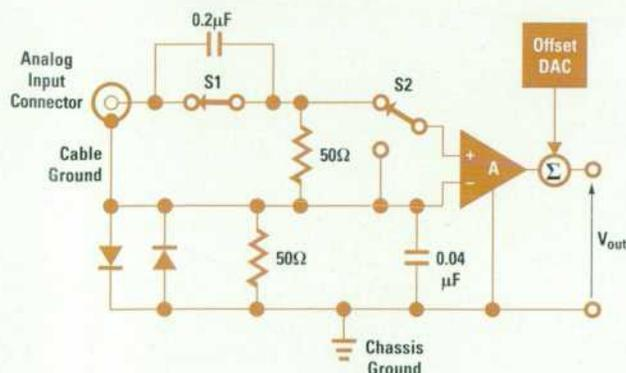
Fig. 3. Analog signal conditioning equivalent circuit.
