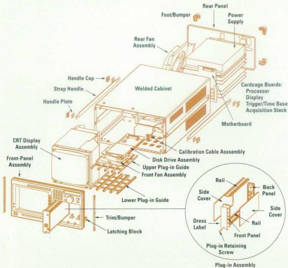
**Fig. 5.** Modularity of components is required for assembly into the cabinet and contributes to overall simplicity and organization of the production flow. This drawing shows the chamfered protrusions in the front panel that define the plug-in slots and the top and bottom guide rails for the plug-ins.
