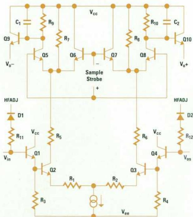
**Fig. 13.** Bipolar differential current-mode sampler schematic diagram.
