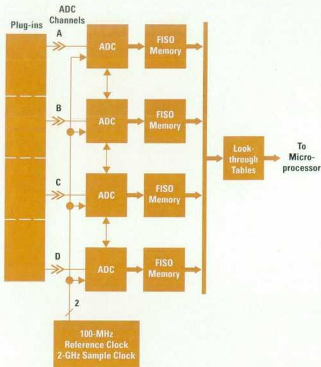
Fig. 4. Block diagram of the HP 54720 acquisition system.
