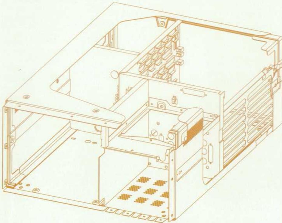
**Fig. 1.** View of the oscilloscope cabinet from the front. Internal compartment elements and the external cosmetic shell are welded into a single structure. Clockwise from the left front are compartments for the display, the fan, the cardcage, and the plug-ins. The compartment at the right front above the plug-ins houses the plug-in fan and disk drive.
