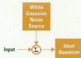
Fig. 9. Adding noise to randomize quantizing error.
