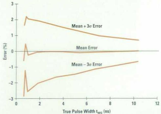
**Fig. 6.** HP 54720A bias-corrected pulse height error at 4 GSa/s. Bias corrections for Gaussian pulse amplitude measurements reduce the HP 54720A's bias to less than 0.5% for most of the range and to less than 0.1% for wider pulses.
