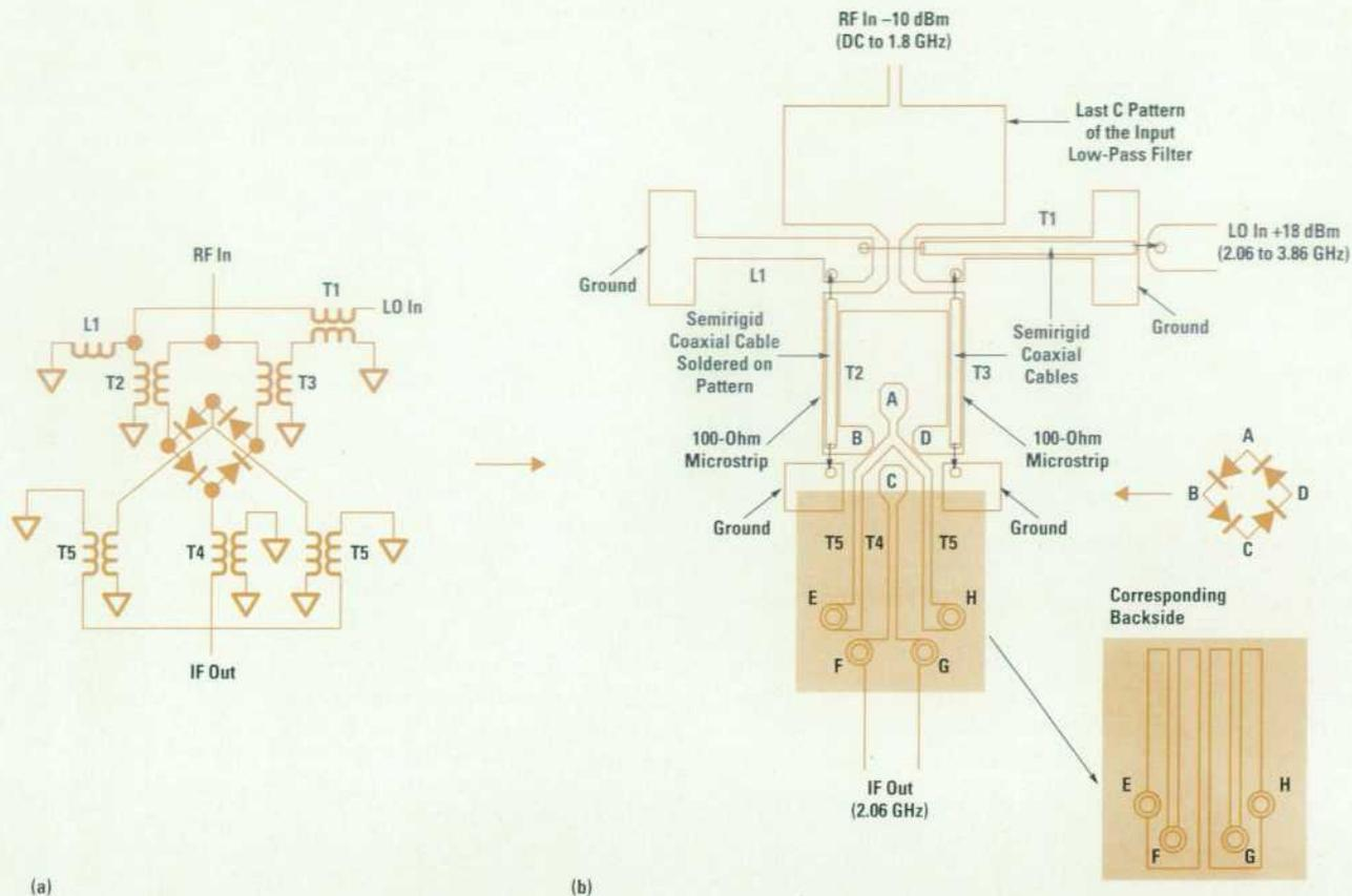
**Fig. 4.** (a) The layout of the first mixer based on the schematic shown in Fig. 3 and (b) the physical layout of the first mixer. The double balanced mixer is implemented on the printed circuit board in such a way that its layout has complete symmetry.
