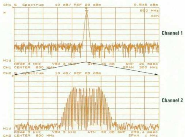
**Fig. 8.** An example of the cross-channel marker zoom function. In this case channel 1 is used for tracking a signal with a wide frequency span and channel 2 is used for zooming in to measure sidebands of the signal. Zoomed-in sidebands can be measured without missing a signal that is frequency hopping.
