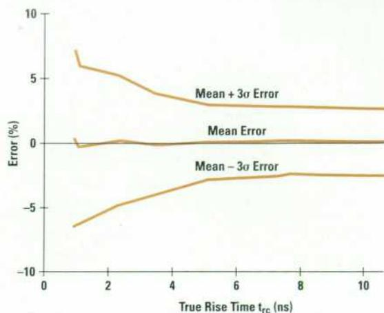
**Fig. 2.** HP 54720A bias-corrected rise time error at 4 GSa/s. Rise time measurement bias in the HP 54720A can be greatly reduced by correcting the readings for gain and offset. ( $t_{rc}$  is the true rise time as measured by the HP 54124T.)
