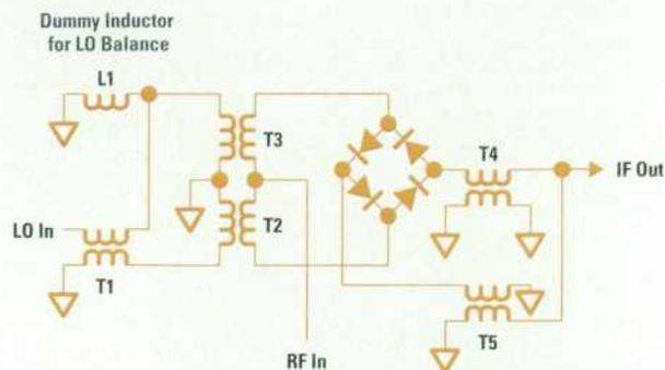
Fig. 3. Schematic diagram of the first mixer.
