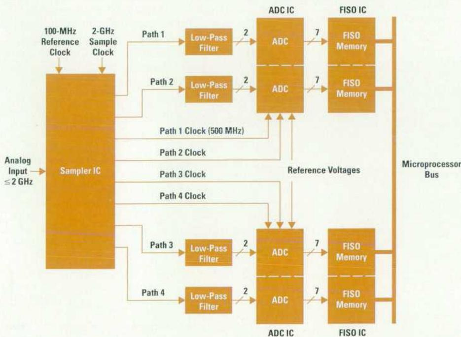
Fig. 7. Acquisition hybrid block diagram. There are four sampler channels on each hybrid.
