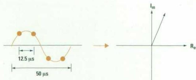
**Fig. 10.** Four data points are collected in the ac sampling mode to determine the real and imaginary parts of the 20-kHz signal. The sample rate is based on the 80-kHz (12.5-μs) ADC.
