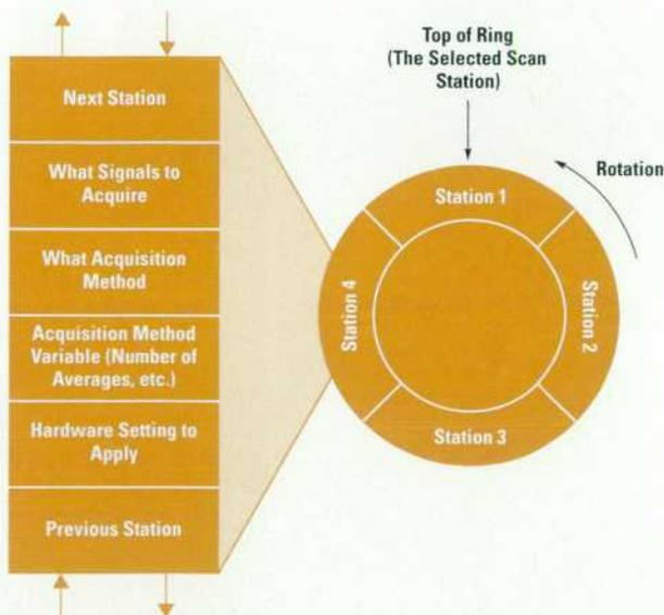
Fig. 5. The ring is a circularly linked list. It provides a good abstraction of the repetitive acquisition schedule of the oscilloscope.
