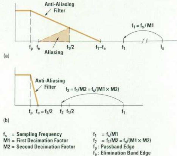
**Fig. 1.** Signal processing and filter specification for two-stage decimation. (a) First-stage decimation. (b) Second-stage decimation.
