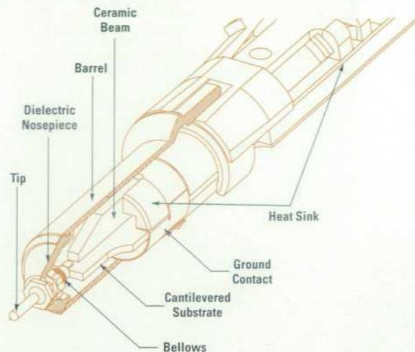
Fig. 4. Cutaway view of the probe tip.
