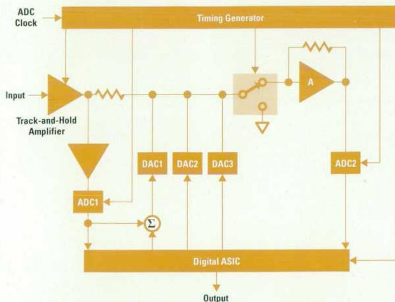
Fig. 15. Hardware block diagram of the 10-MHz ADC.
