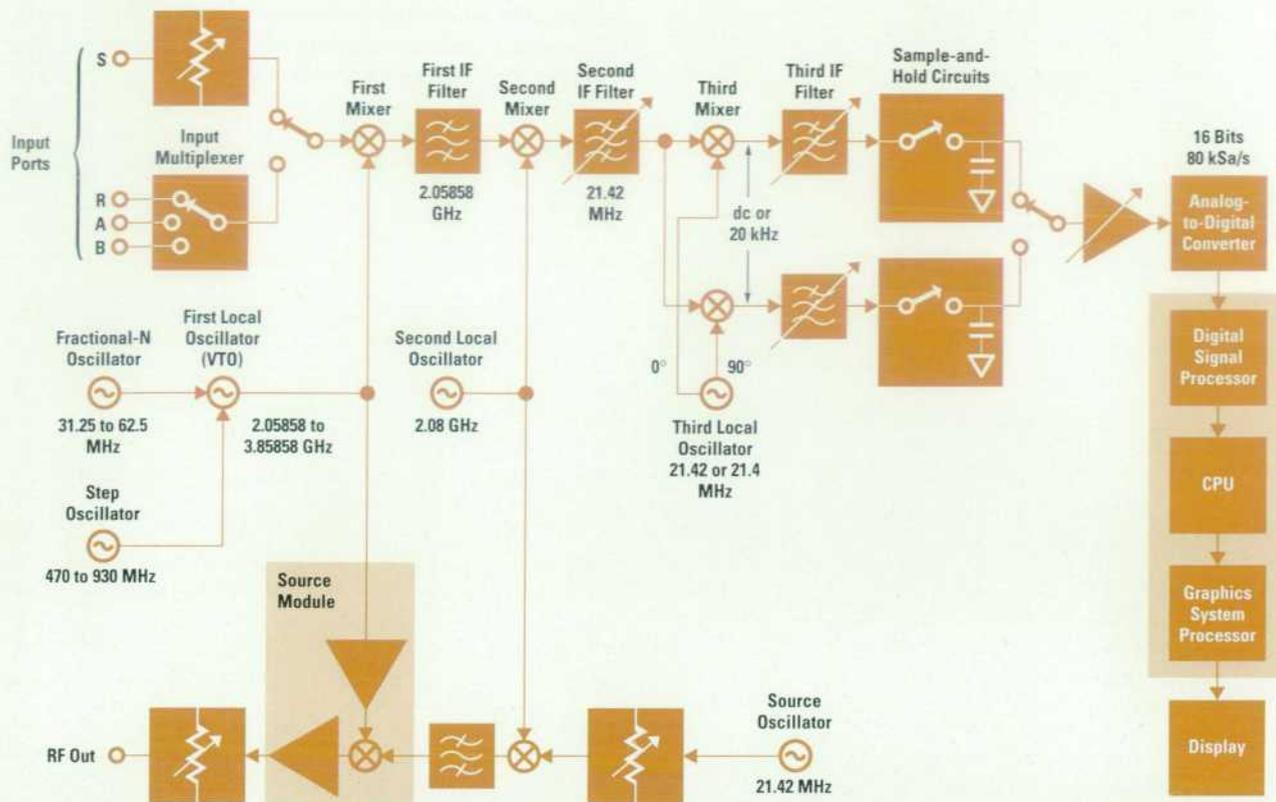
Fig. 9. Simplified block diagram of the HP 4396A.
