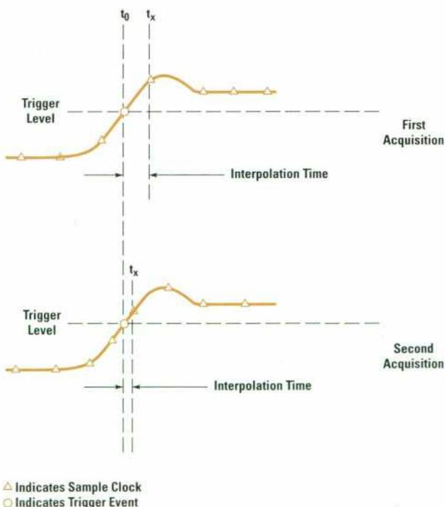
Fig. 6. The interpolator measures the time between the trigger ( $t_0$ ) and the next sample clock ( $t_x$ ).
