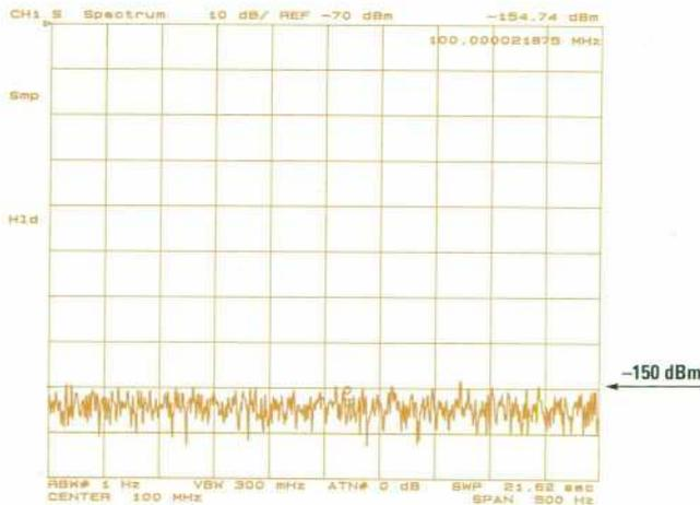
Fig. 11. The system noise floor for the HP 4396A is about  $-155$  dBm/Hz at 100 MHz.
