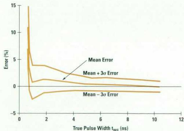
**Fig. 3.** HP 54720A single-shot impulse width measurement error at 4 GSa/s. Measurements of narrow Gaussian pulse widths on an HP 54720A show a dip and an abrupt increase in error below one nanosecond. ( $t_{wc}$  is the true pulse width as measured by an HP 54124T.)
