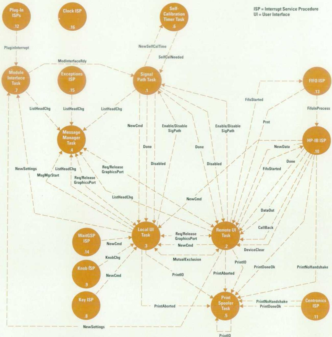
Fig. 4. Host processor tasks in the HP 54720/10 oscilloscope.
