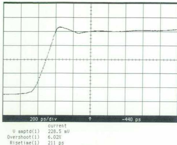
Fig. 22. Step response of an 8-GSa/s HP 54720 system.
