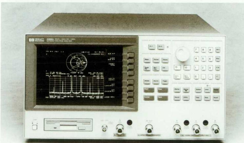
**Fig. 1.** The HP 4396A high-performance vector network and spectrum analyzer provides the capabilities of both types of analysis without compromising the performance of either. Options include burst-signal analysis and HP Instrument BASIC programming.
