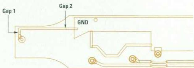
Fig. 2. Dual-cut spark gap for electrostatic discharge protection.
