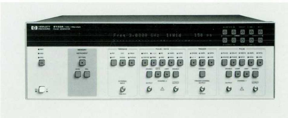
**Fig. 1.** The HP 8133A pulse generator provides pulses with repetition rates up to 3 GHz. All pulse parameters are accurately programmable. An optional second channel can be either a pulse channel or a pulse/data channel capable of generating a 32-bit data word or a pseudorandom binary sequence.
