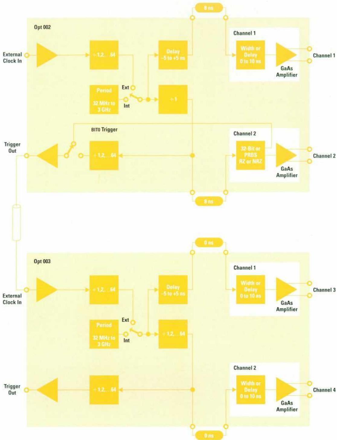
**Fig. 3.** Two two-channel HP 8133A pulse generators in a four-channel master-slave configuration. In the lower instrument channel 2 is a pulse channel like channel 1, while in the upper instrument channel 2 is a pulse/data channel. External delay lines compensate for timing skew between the output channels of the two instruments.
