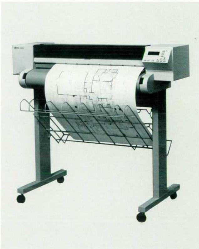
**Fig. 1.** The HP DesignJet plotter uses thermal inkjet technology to produce large-format plots on commonly available drafting media. A roll-feed mode allows unattended plotting with automatic cutting and stacking of completed plots. Resolution is 300 dots per inch and plot time for a D-size plot is about three minutes.
