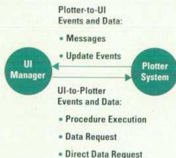
**Fig. 10.** Interaction between the plotter system and the user interface manager. The user interface can request the plotter system to schedule the execution of a particular function or procedure. The user interface manager can also send a request for data maintained by the plotter system. The plotter system interacts with the user interface manager by means of messages and update events.
