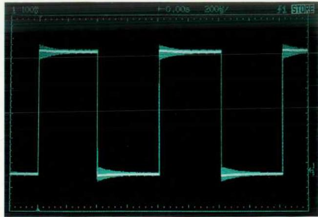
**Fig. 2.** Minimizing overshoot by adjusting a circuit so that the current live trace at full intensity is always within the autostored historical traces at half intensity.
