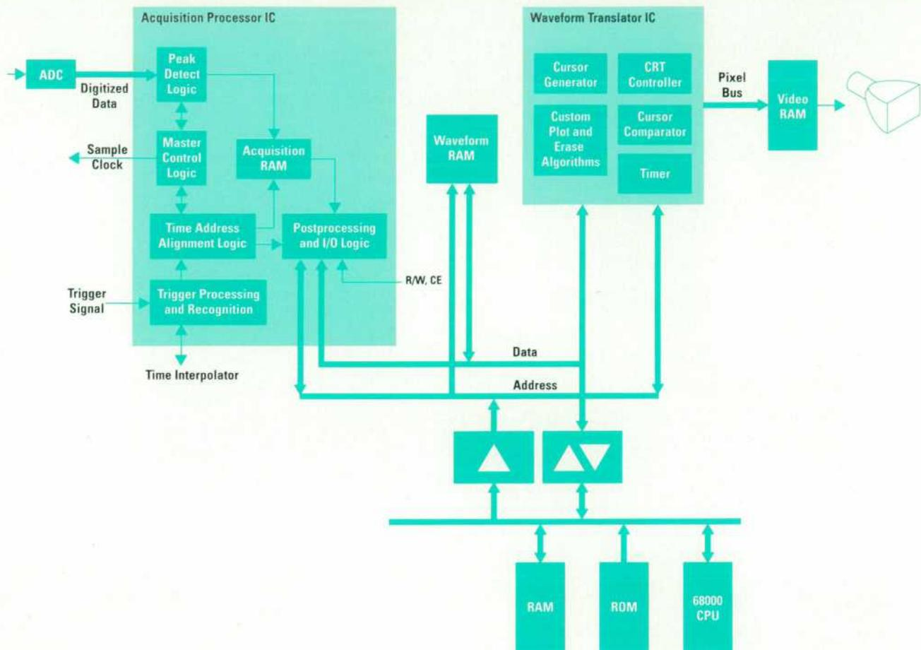
Fig. 3. New raster digital oscilloscope architecture.
