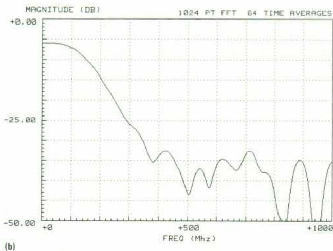
**Fig. 4.** Noise in the frequency response of an HP 54600A. (a) No averages. (b) 64 averages.
