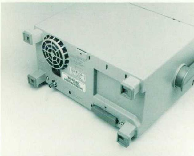
Fig. 3. Two screws allow removal of the chassis assembly from the cabinet. For ruggedness, the rear feet are integrated into the cabinet and have four load-bearing walls.
