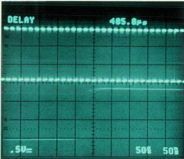
Fig. 3. Analog oscilloscope delayed sweep display.
