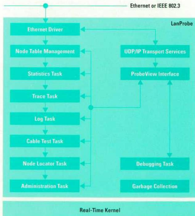
Fig. 8. HP LanProbe internals and tasks.
