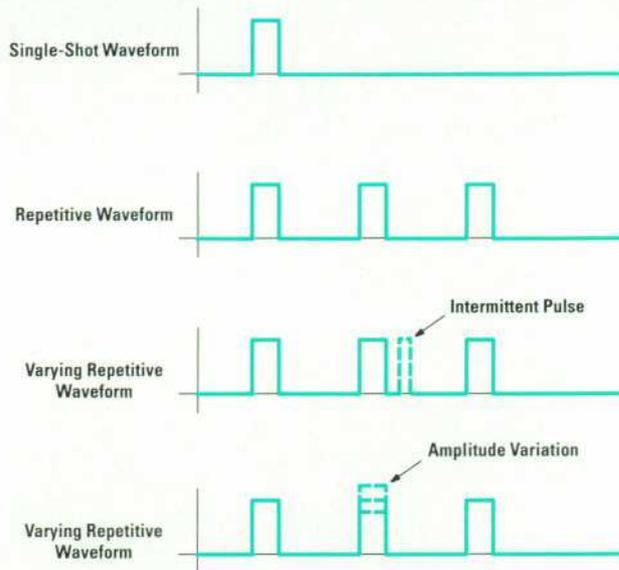
Fig. 2. Waveform types.
