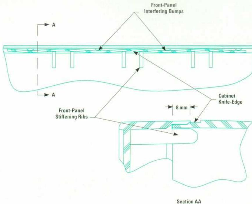
**Fig. 7.** Details of the contact method used to mate the front panel to the cabinet. The amount of deformation in the cabinet knife-edge is exaggerated for clarity. Some deformation also occurs in the wall of the front panel. Also see Fig. 1 on page 41.
