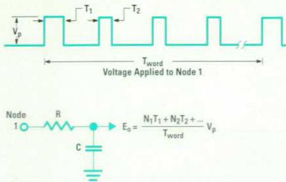
Fig. 2. Filter section input waveform and output voltage.
