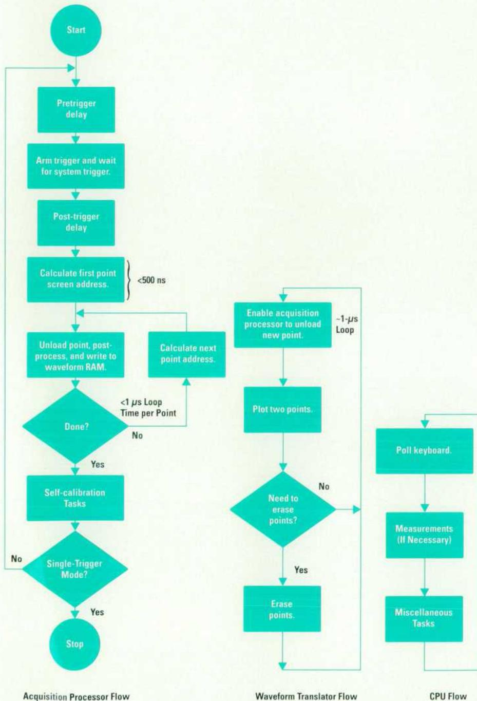
Fig. 4. Simplified task flows in the new raster digital oscilloscope architecture.
