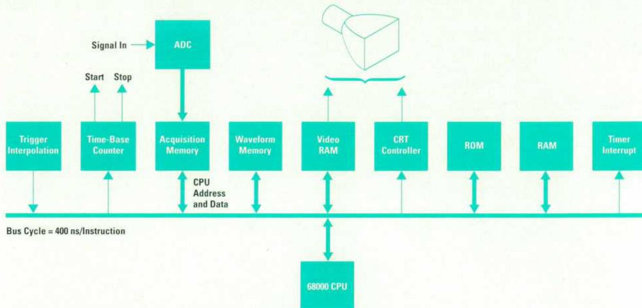
Fig. 1. Previous raster digital oscilloscope architecture, simplified.
