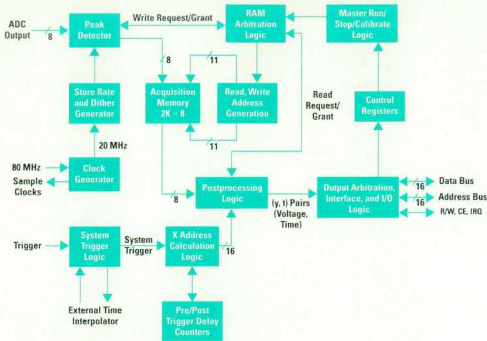
Fig. 5. Logical block diagram of the acquisition processor.
