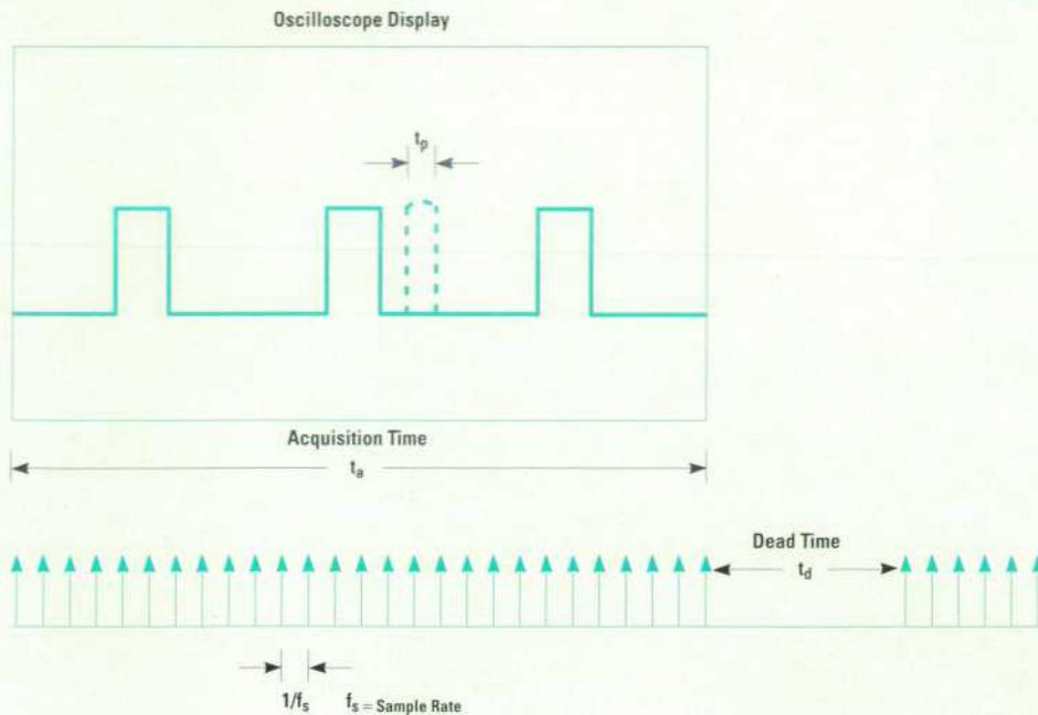
Fig. 3. Acquisition time, sample rate, and dead time.
