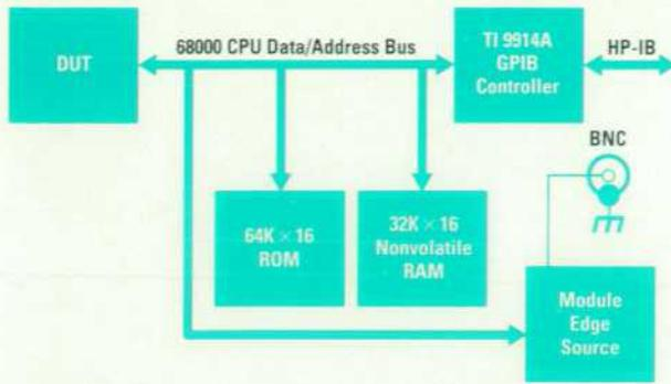
Fig. 2. Block diagram of the production calibration module.
