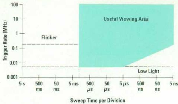
Fig. 1. Analog oscilloscope operating area.
