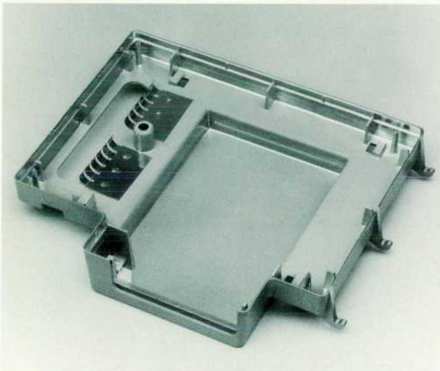
**Fig. 4.** A finger stock strip is used to reduce the radiated emissions from the option module. The fingers contact the module connector ground shell.
