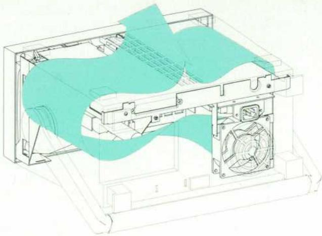
**Fig. 5.** Airflow in the HP 54600 Series.
