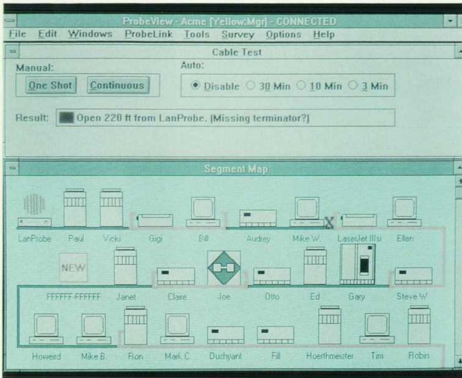
**Fig. 6.** The cable test tool can be used on a one-shot basis or set to run continuously to capture intermittent faults. The test is non-disruptive and shows the location and nature of a cable problem.
