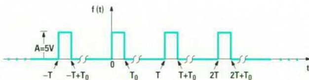
Fig. 12. A generic filter input voltage.
