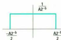
Fig. 1. Probability density function assumed for quantization noise of an ADC with  $b$  bits and a range of  $A$ .
