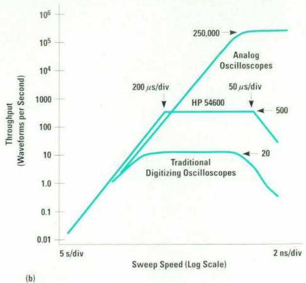
**Fig. 8.** (a) HP 54600 screen update rate. (b) HP 54600 throughput compared to analog oscilloscopes and traditional digitizing oscilloscopes.
