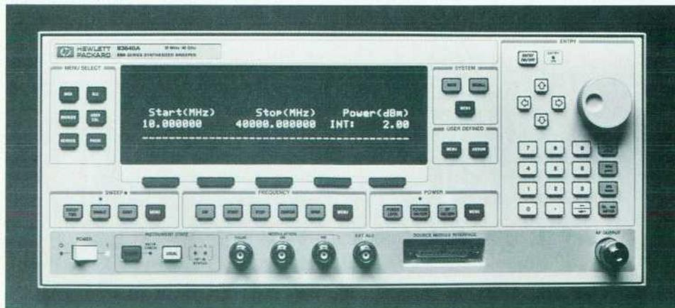
**Fig. 1.** HP 8360 synthesized sweep oscillators include eleven models that cover the frequency range from 10 MHz to 50 GHz. Millimeter heads extend the frequency range to 110 GHz (Model 83640A shown). High-power models provide 17 dBm at 20 GHz. Analyzer models have special network analyzer synchronization features.
