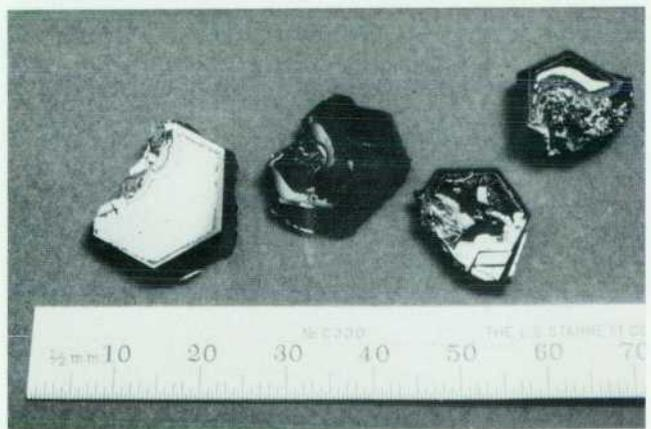
Fig. 2. Hexagonal ferrite crystals.
