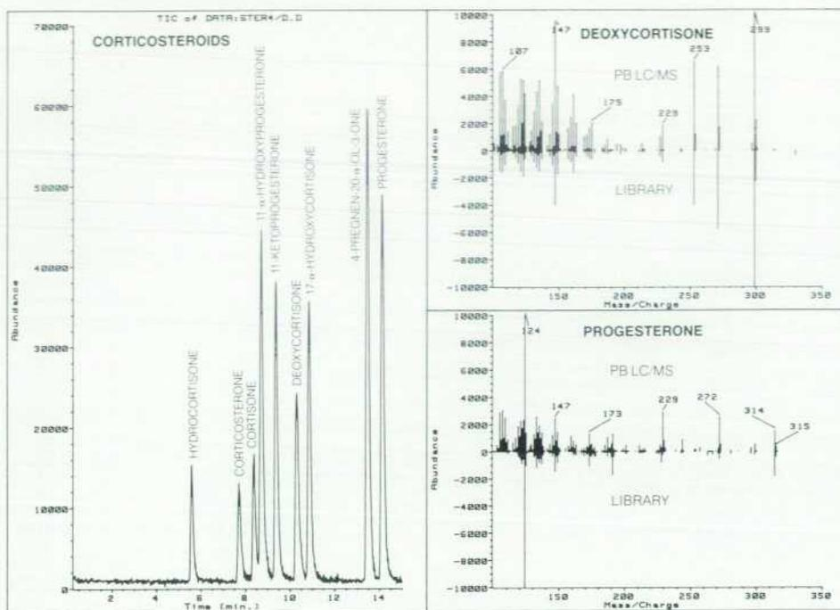
Fig. 12. Separation of corticosteroids by particle beam LC/MS.
