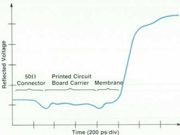
Fig. 8. Time-domain reflectometry profile and characteristic impedance.
