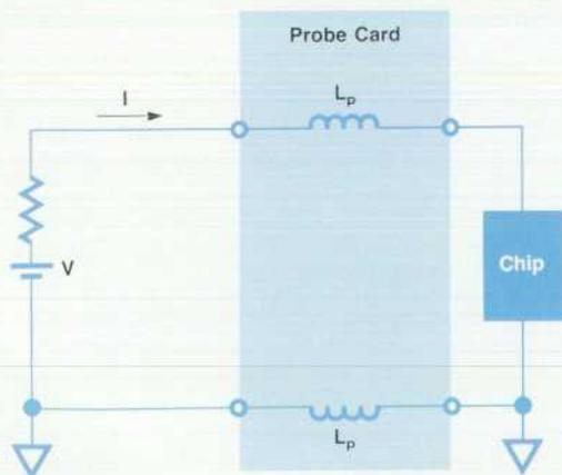
Fig. 4. A power line in a conventional probe.
