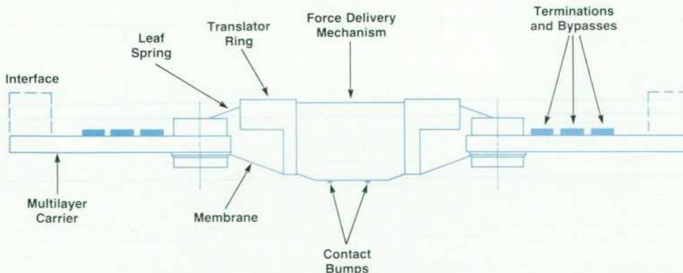
Fig. 6. Architecture of the membrane probe card.
