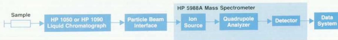
**Fig. 1.** For particle beam liquid chromatography/mass spectrometry (LC/MS), a special interface is mounted between the LC and MS systems. The data system can be either an HP 59970C ChemStation for single-instrument operation or an HP 1000 computer system for multiinstrument, multitasking, multiuser operation.
