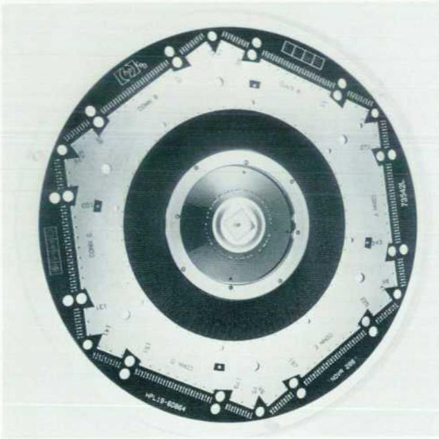
Fig. 16. The membrane probe for microprocessor testing.
