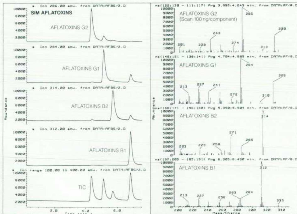
Fig. 13. Separation of aflatoxins by particle beam LC/MS.
