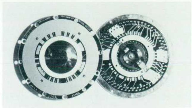
Fig. 14. The membrane probe for DAC testing.
