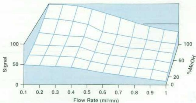
Fig. 7. Effects on sensitivity of mobile phase flow rate and composition.
