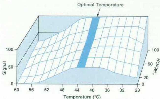
Fig. 5. Effects on sensitivity of desolvation chamber temperature and mobile phase composition.
