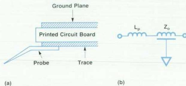
Fig. 1. Conventional wafer probe. (a) Structure. (b) Equivalent circuit.
