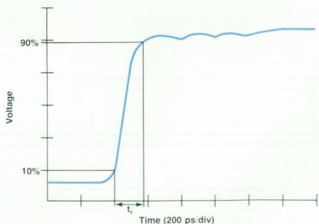
Fig. 9. Transmission response and rise time.
