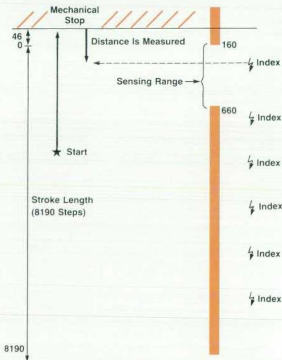
Fig. 10. Determination of an absolute reference position.
