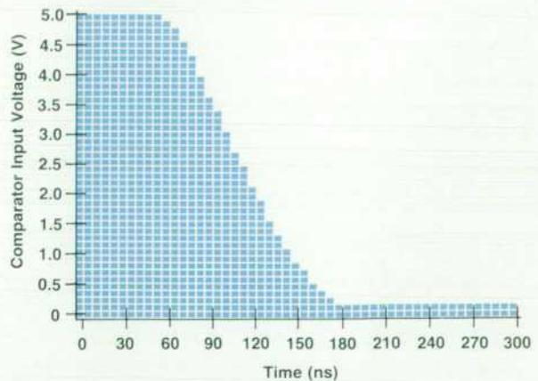
**Fig. 4.** CMOS MC14000 family output signal ( $V_{oh} = 2.5V$  at  $I_{oh} = 2.1$  mA,  $V_{ol} = 0.4V$  at  $I_{ol} = 0.44$  mA) with open-ended transmission line ( $t_{pd} = 3$  ns), comparator in high-Z mode (lumped capacitance = 23 pF, resulting in a load of 50 pF total).
