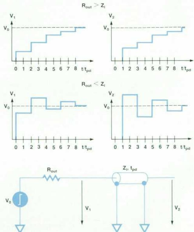
Fig. 4. Underterminated model.
