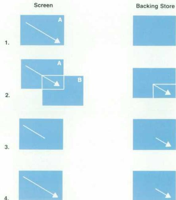
**Fig. 11.** Views of a window and its backing store. In frame 1 window A is completely visible and backing store is empty, in frame 2 window A is partially obscured by window B. In frame 3 window A is unobscured and part of the screen picture is missing, and in frame 4 the missing part of the picture is copied from backing store to window A without intervention by the client.
