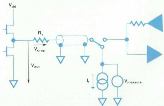
Fig. 17. Dc measurement path using the resistive divider.
