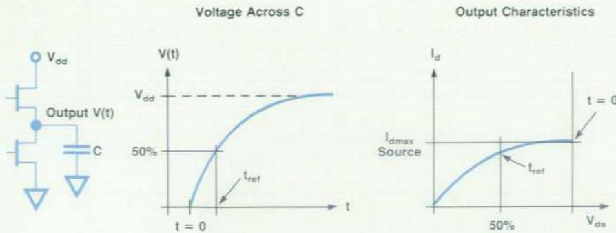
Fig. 9. CMOS output driving a capacitive load.
