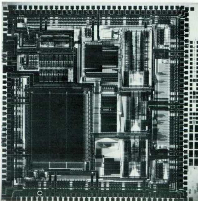
Fig. 4. TREIS (TTransform Engine In Silicon) chip.
