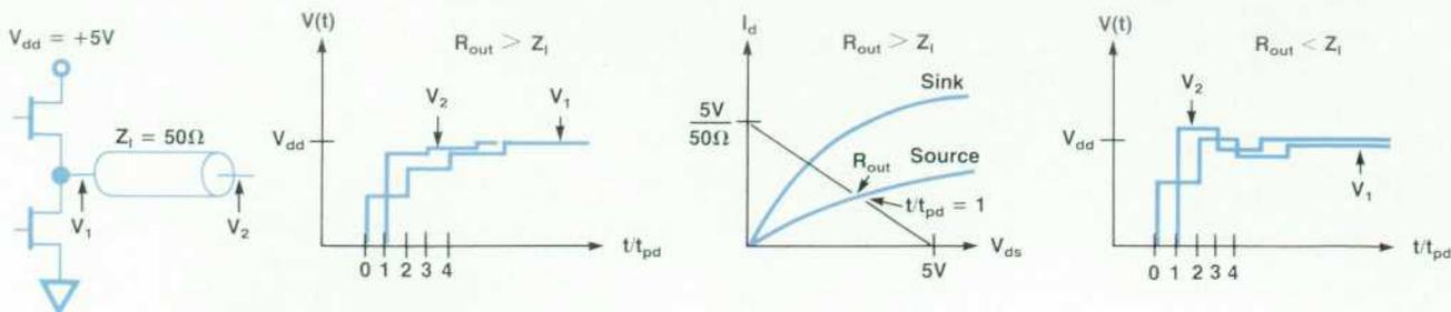
Fig. 11. CMOS output driving an open-ended transmission line.
