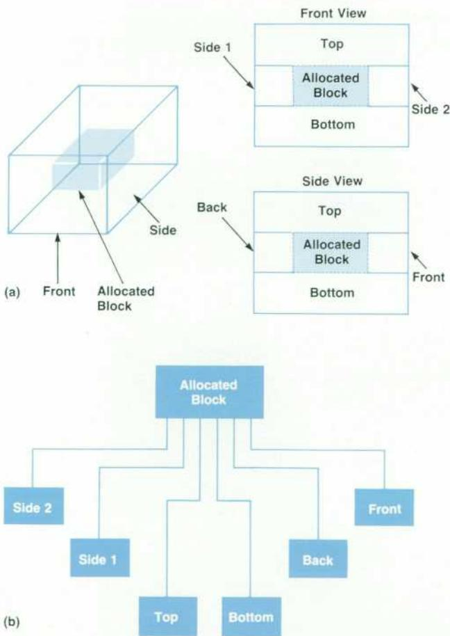
**Fig. 8.** (a) Two-dimensional views of an allocated block with front and back added. (b) Data structure representation of an allocated block with the six free blocks from the original block of memory.
