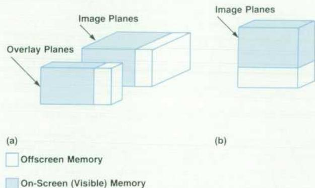
**Fig. 2.** The organization of the image planes in the frame buffer. (a) A display system containing both image and overlay planes (e.g., the HP 98550A Color Graphics Board). (b) A display system with only image planes in the frame buffer (e.g., the HP 98547A).
