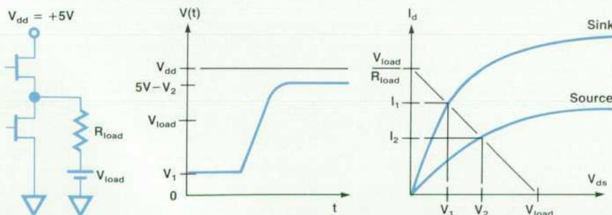
Fig. 10. CMOS output driving a resistive load.
