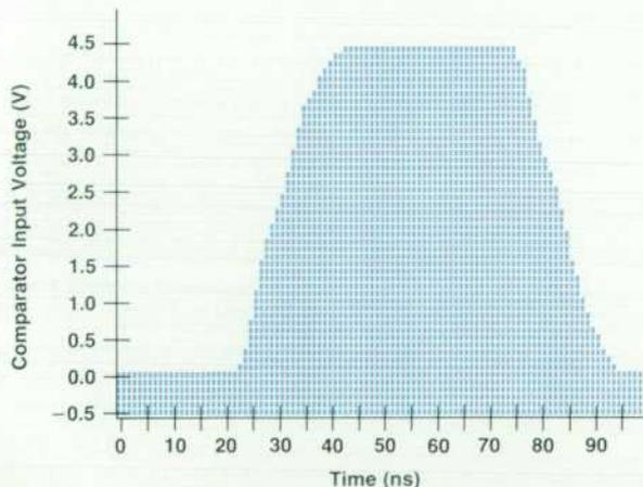
**Fig. 2.** Shmoo plot of comparator input signal from an HCMOS output buffer with 4-mA source/sink capability, loaded by an open-ended transmission line ( $t_{pd} = 3$  ns) with the comparator in high-Z mode (lumped capacitance = 23 pF).
