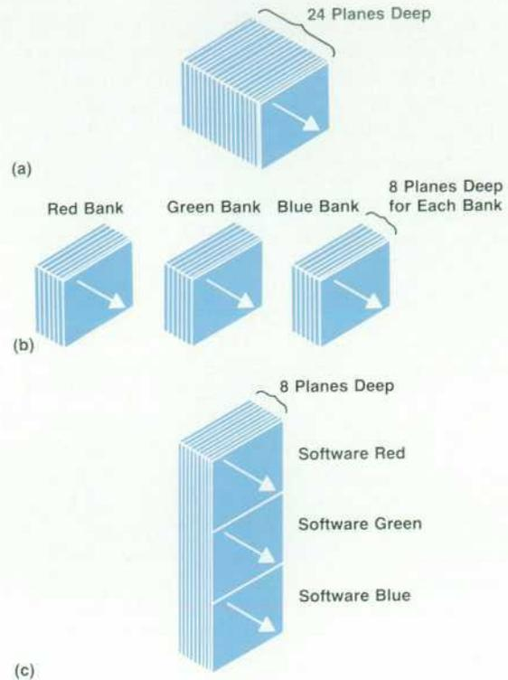
**Fig. 12.** (a) A 24-plane-deep window on the screen. Of course the physical depth of display memory is not seen by the user. (b) 24-plane-deep backing store in offscreen frame buffer memory organized in three hardware banks of 8 planes each. The picture on the display is replicated on the three banks. (c) 24-plane-deep backing store in virtual memory. This is a contiguous piece of memory organized in three compartments. Each compartment is a software bank mirroring the hardware banks.
