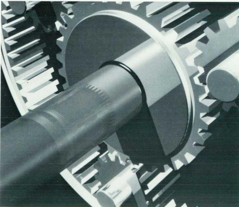
**Fig. 1.** These gears were generated on the HP ME Series 30 modeling, design, and drafting system. The ray traced image was rendered using nonuniform rational B-splines. It is a polygonal representation with 3084 polygons and 12 partial polygons.
