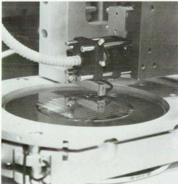
**Fig. 3.** Inkjet printheads being removed from the low-tack mounting tape in the head attach machine.
