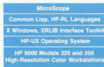
Fig. 5. Microscope's platform.
