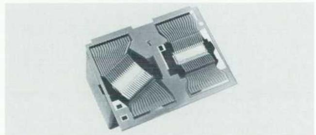
Fig. 7. A leadframe in contact with print cartridges.
