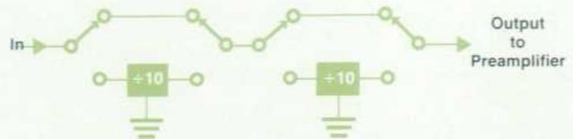
Fig. 2. Input attenuator with  $\div 10$  sections and straight-through  $\div 1$  path.
