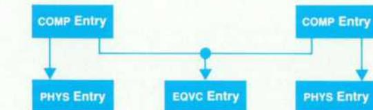
Fig. 1. The composition of a component definition allows sharing of entries to reduce data redundancy.
