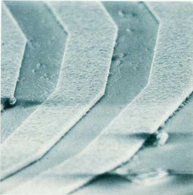
**Fig. 2.** 420 $\times$  magnified photograph of spiral inductor traces on the preamp hybrid. The traces are 50  $\mu\text{m}$  wide on a 100- $\mu\text{m}$  pitch and are 10  $\mu\text{m}$  thick. Pattern plating gives the advantages of thin-film technology with a factor of 20 improvement in trace conductivity.
