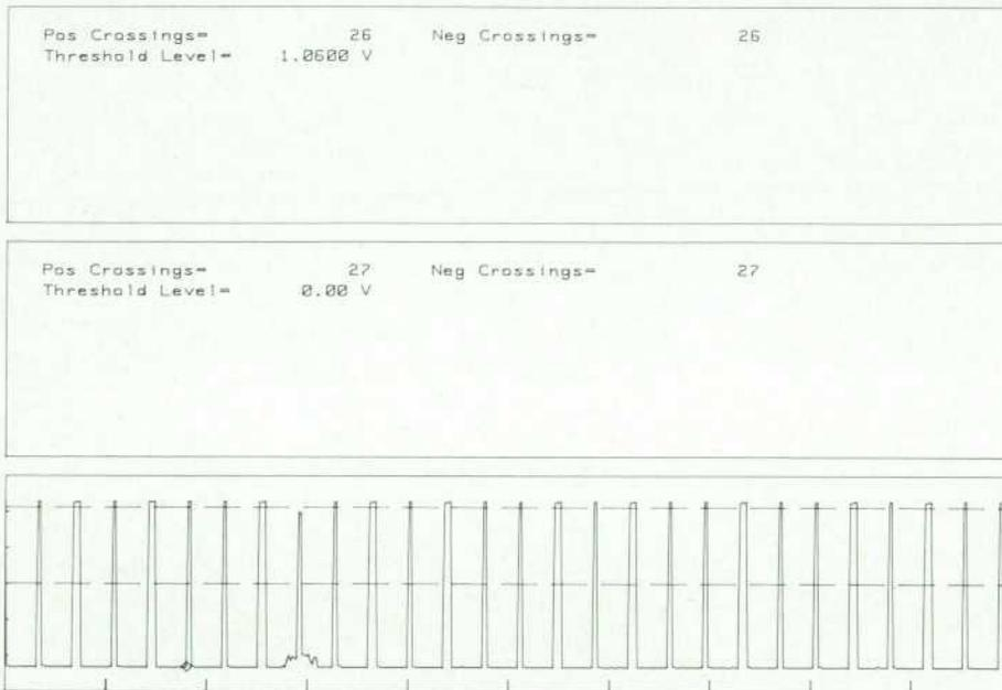
**Fig. 15.** Using the event crossing function at different threshold levels, a single marginal pulse can be detected automatically.
