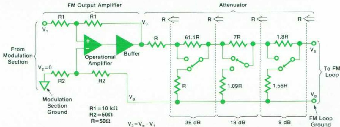
Fig. 2. FM output attenuator with floating ground.
