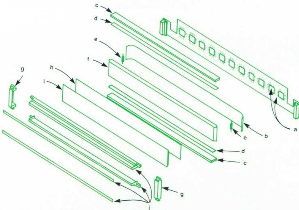
**Fig. 4.** LCD display construction. (a) LCD printed circuit board. (b) Main reflector. (c) Conductive elastomer connectors. (d) Spacers/reflectors. (e) Light bulbs. (f) Backlight. (g) Locators. (h) Diffuser. (i) LCD. (j) Retaining hardware.
