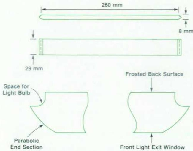
Fig. 5. Backlight detail.
