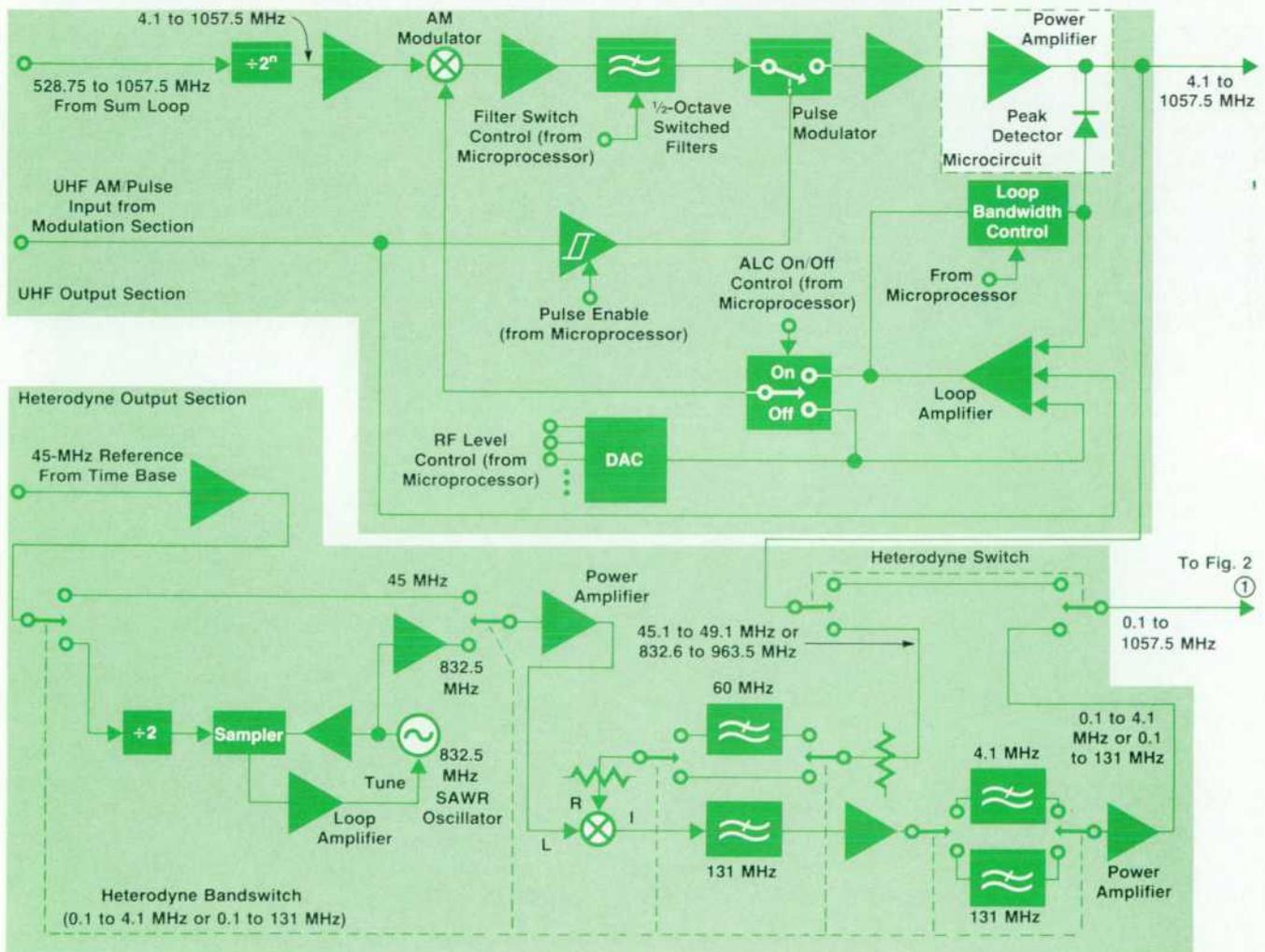
Fig. 1. HP 8642A/B Signal Generator UHF and heterodyne output sections.
