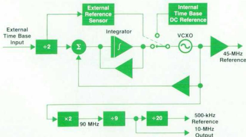
Fig. 2. Time base loop block diagram.
