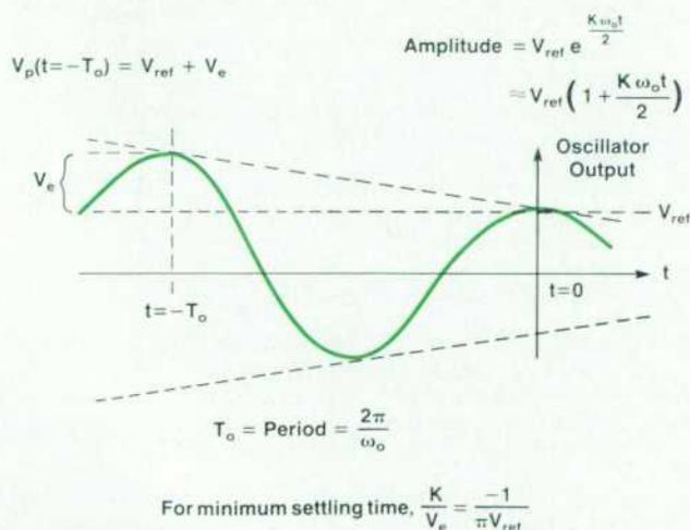
Fig. 7. Optimization of ALC loop gain.
