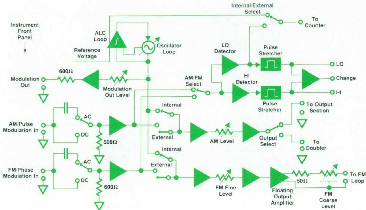
Fig. 1. HP 8642A/B modulation section block diagram.
