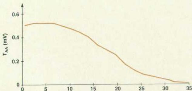
Fig. 3. Track average amplitude  $T_{AA}$  versus transition density along the recording track.
