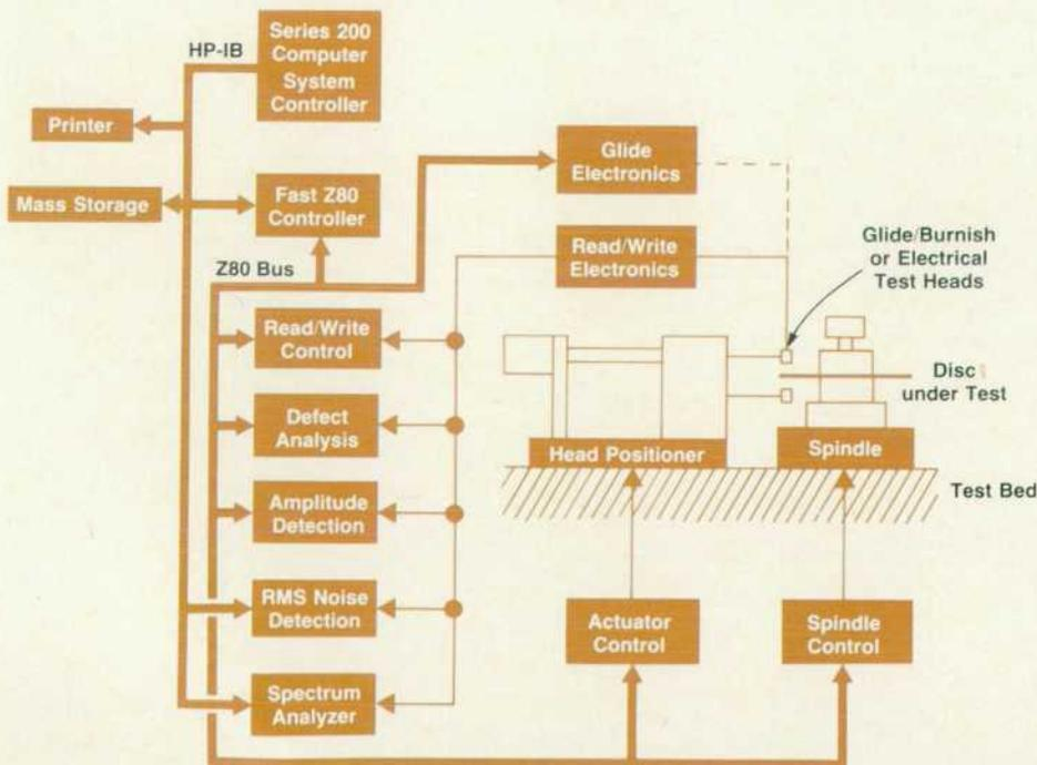
Fig. 1. Test system block diagram.
