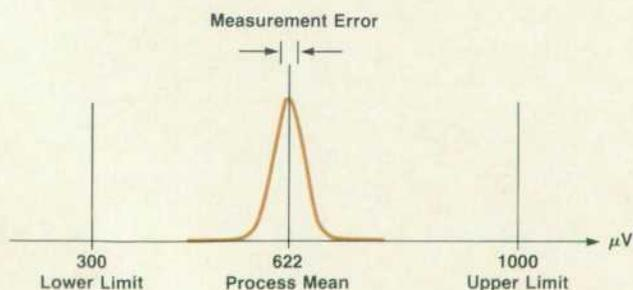
Fig. 3. A high-yield parameter example (track average amplitude at the disc outer diameter). Process standard deviation = 24.8  $\mu\text{V}$ . Yield = 100%.
