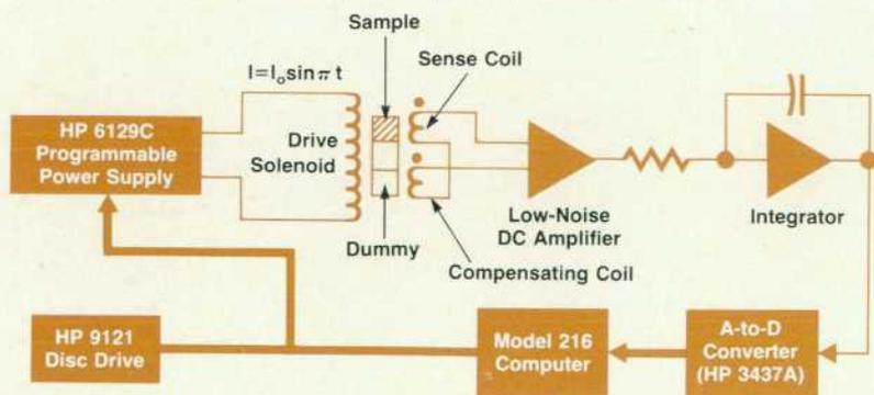
**Fig. 1.** Block diagram of M-H loop measurement system. The sample and dummy are magnetized by the field of the drive solenoid, which is fed with a sinusoidal current by the programmable power supply. The voltage signal resulting from the rate of change of the sample magnetization is amplified, integrated, and digitized. The computer calculates and displays the M-H loop and stores the results of all measurements.
