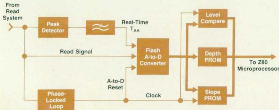
Fig. 12. Block diagram of defect analysis system.
