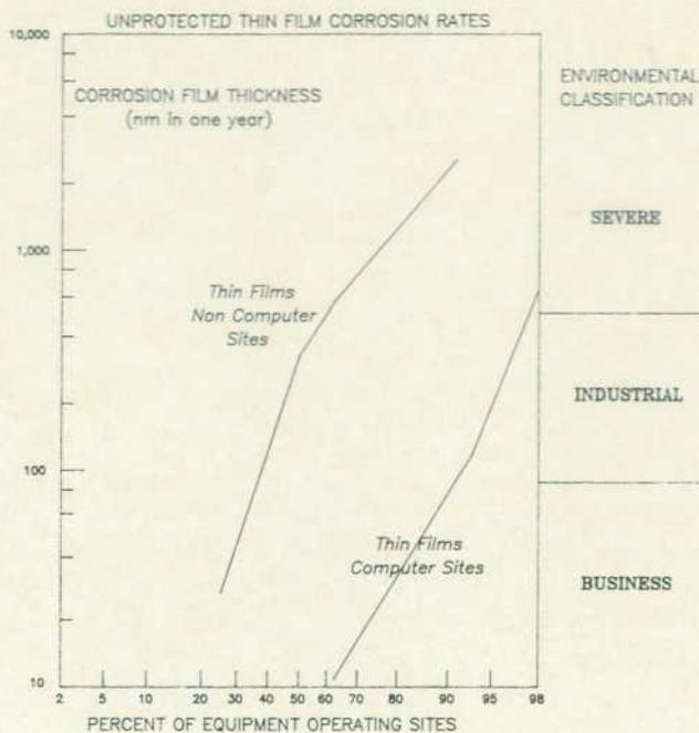
**Fig. 8.** Corrosion results from field tests conducted using sample boards illustrated in Fig. 6 and 7. These results are for samples located in chamber 1 of the sample boards. Samples in chamber 2 were protected below the detection level.
