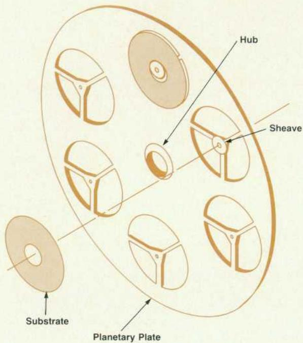
**Fig. 3.** Deposition uniformity across the surface of a thin-film magnetic disc is assured by using a planetary carrier with each disc mounted on a sheave that allows free disc rotation as the carrier is rotated.
