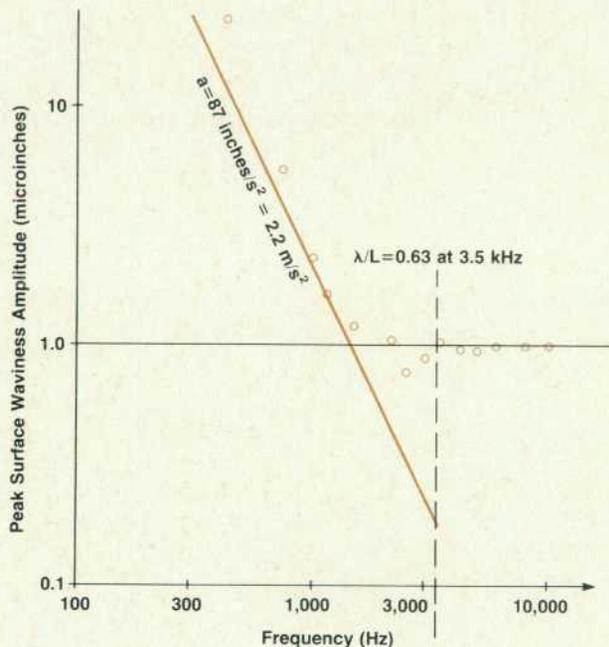
**Fig. 8.** Plot of peak surface waviness amplitude versus frequency for innermost track of HP 97501A Disc Drive. Surface velocity = 0.75 inches/s, radius = 1.0 inch, and variation in flying height =  $\pm 1.0 \text{ microinch}$ .
