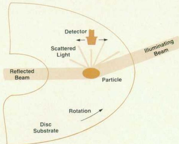
**Fig. 1.** The laser particle scanner detects particles by measuring light scattered by the particles. The disc surface is scanned in a spiral pattern by rotating the disc and moving the detector along a disc radius illuminated by the laser beam.
