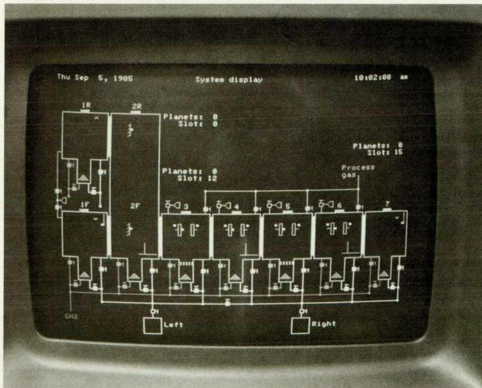
**Fig. 4.** Display showing status of in-line deposition system.
