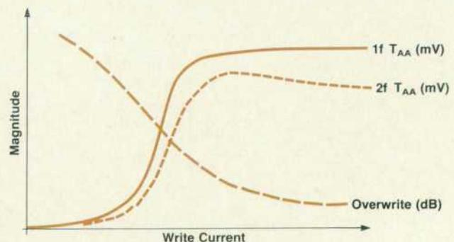
Fig. 4. Typical saturation plots showing  $1f T_{AA}$ ,  $2f T_{AA}$ , and overwrite versus write current.
