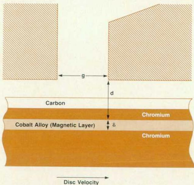
Fig. 1. Head-to-medium geometry for magnetic disc memory.
