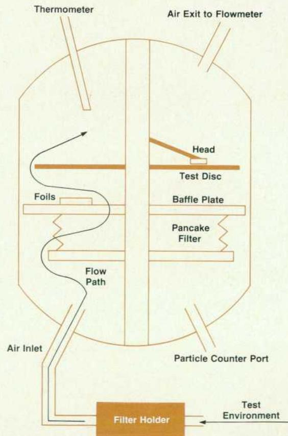
Fig. 4. Cross section of test chamber for evaluating environmental corrosion effects.
