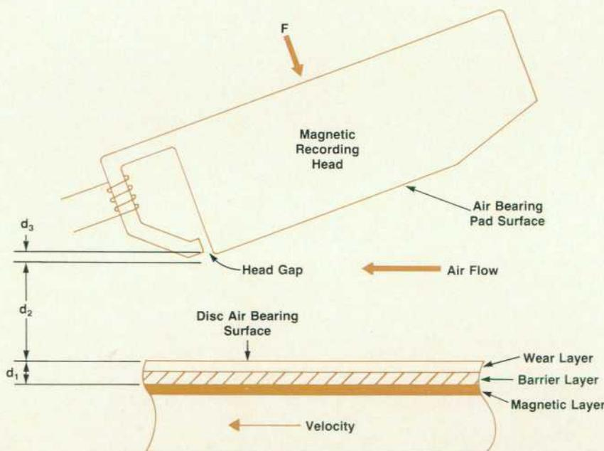
**Fig. 5.** Head-to-disc spacing components of a recording head flying over a disc moving at a velocity  $V$ . Spacing components  $d_1$ ,  $d_2$ , and  $d_3$  are the thickness of the barrier and wear layers, the flying height, and the magnetic pole recession in the head, respectively. The air flow created by the moving disc surface forms a wedge that lifts the head against the spring force  $F$ .
