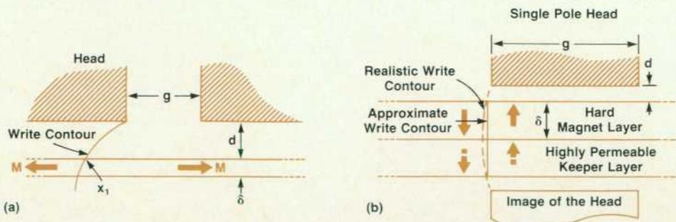
Fig. 6. (a) Longitudinal and (b) perpendicular recording formats.
