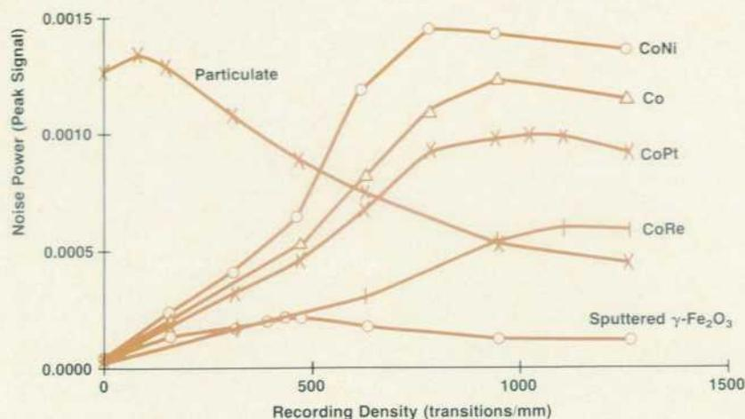
Fig. 2. Total normalized medium noise power versus recording density for various disc memory material systems.
