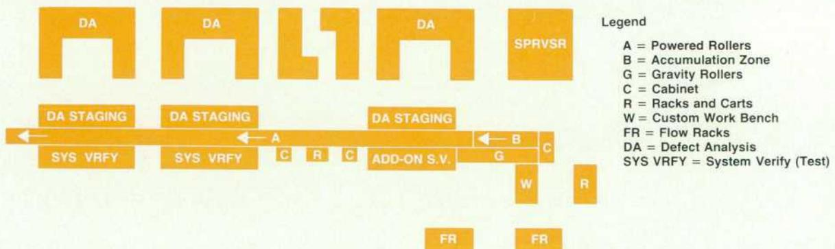
Fig. 1. HP 3000 Series 37 build-test production line.
