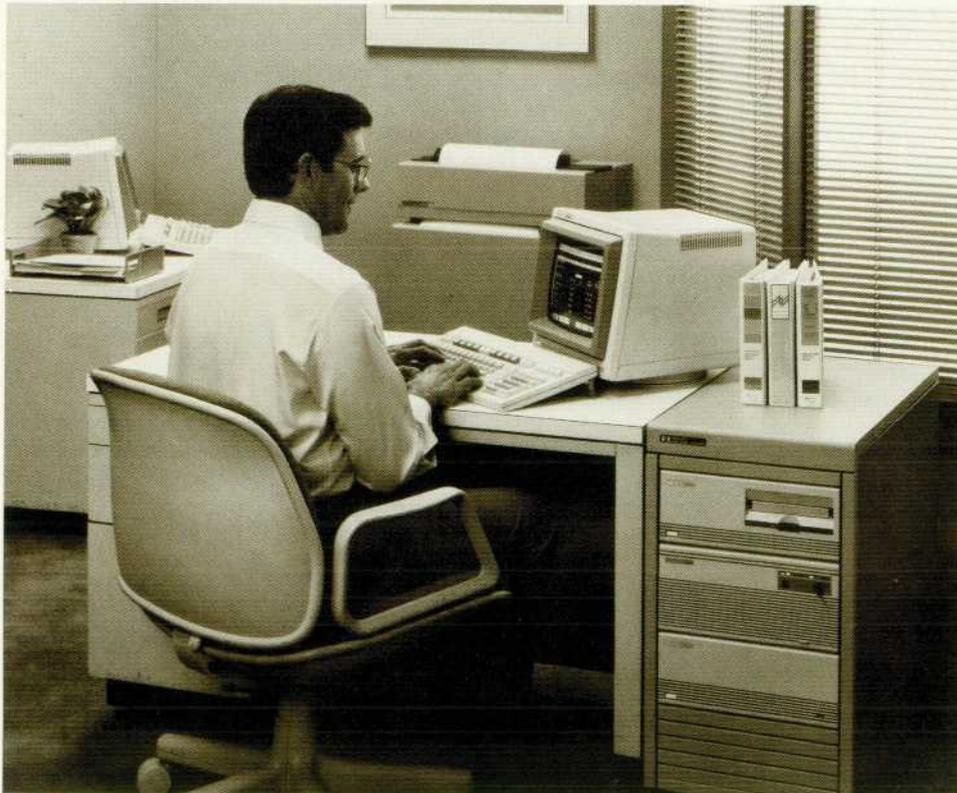
**Fig. 1.** The HP 3000 Series 37 Computer runs the same software as other HP 3000s, supports up to 28 terminals, and fits easily into an office environment. The Series 37 system processing unit is the second unit from the top in the cabinet at right.
