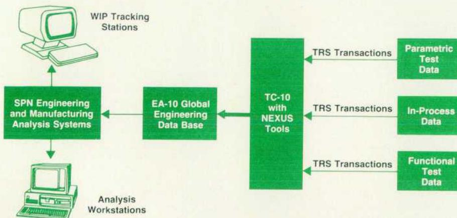
**Fig. 2.** The TC-10 Tester Collection System for SPN couples data from test equipment and process monitors into the EA-10 global data base for access by other SPN modules. The NEXUS software tools included with TC-10 simplify the task of connecting and programming new equipment to communicate with SPN. TRS is the SPN Test Result Standard.
