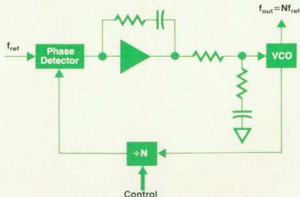
Fig. 4. Conventional +N phase-locked loop block diagram.
