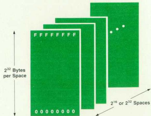
Fig. 1. The new HP architecture provides for up to  $2^{32}$  distinct virtual address spaces, each up to  $2^{32}$  bytes long. Implementations may limit the number of virtual spaces to zero (real addressing only),  $2^{16}$ , or the full  $2^{32}$ .
