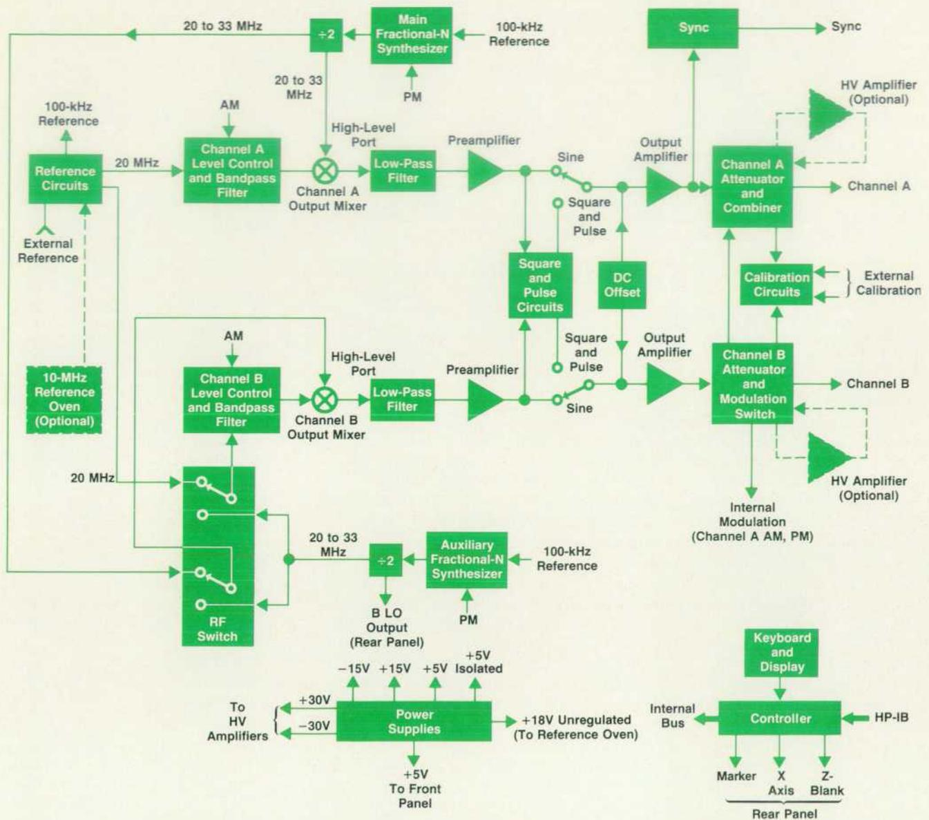
Fig. 2. Simplified HP 3326A block diagram. The functional blocks of a mix-down synthesized signal source appear twice. Fractional-N synthesis provides high-accuracy phase control.
