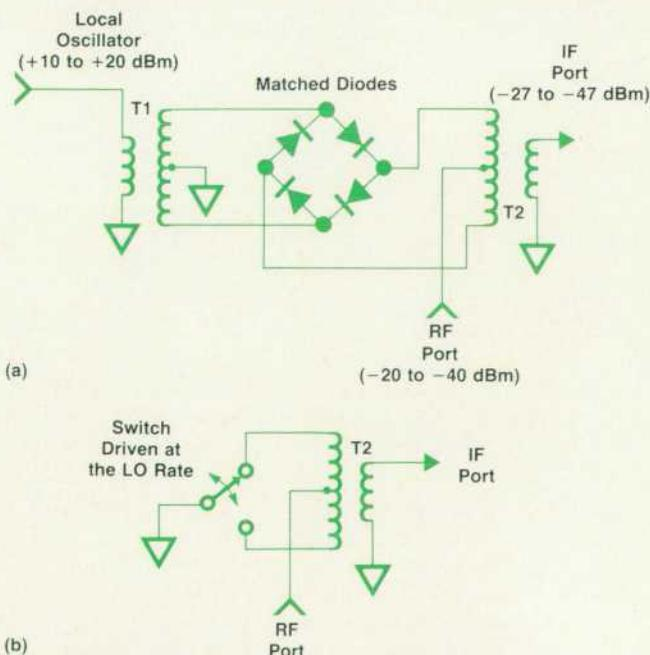
Fig. 2. The classic diode ring mixer (a) and its equivalent circuit (b).
