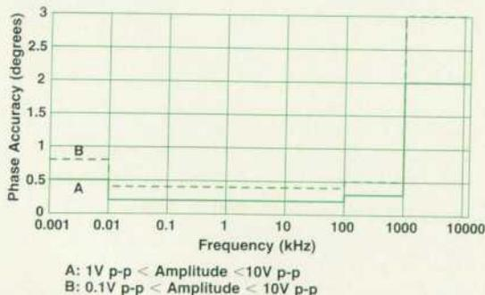
Fig. 1. HP 3326A Two-Channel Synthesizer phase accuracy specifications.
