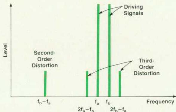
Fig. 1. Second-order and third-order intermodulation distortion products.
