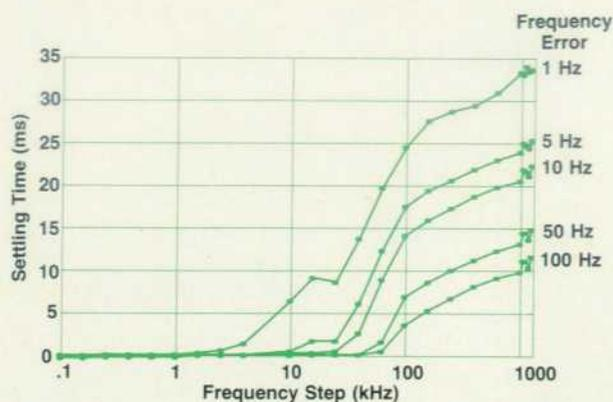
Fig. 2. Typical settling time as a function of the size of the frequency change and allowable frequency error.
