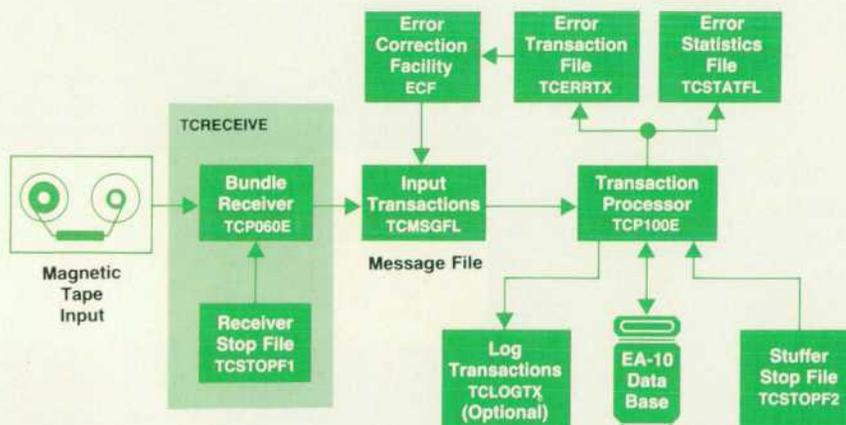
Fig. 6. TC-10 data base stuffer processing flow.
