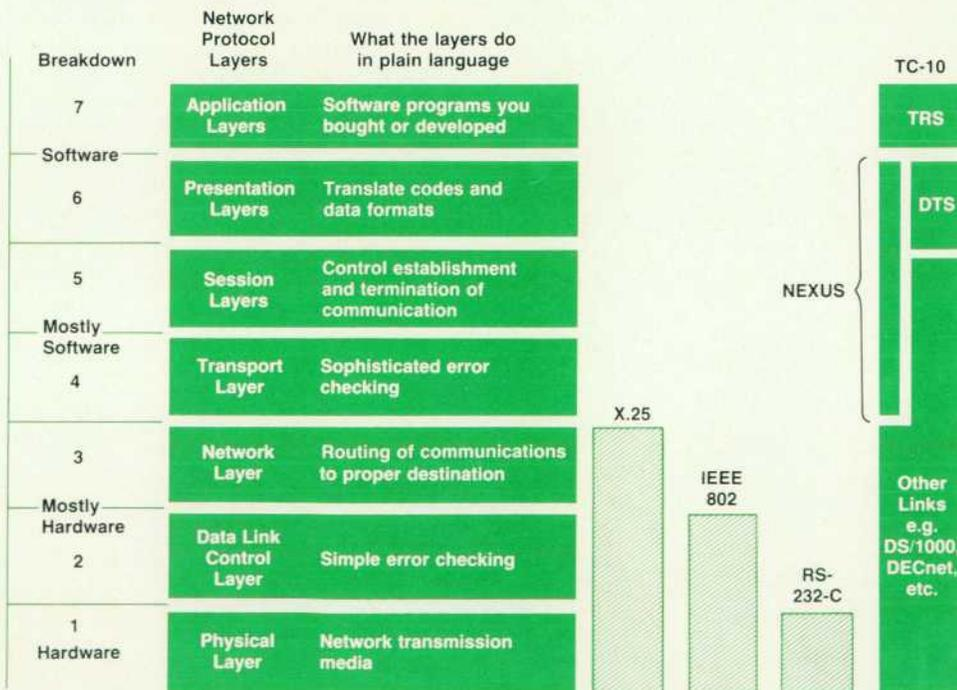
Fig. 3. ISO Open System Interconnect (OSI) model and coverage of TC-10 compared with other network standards.
