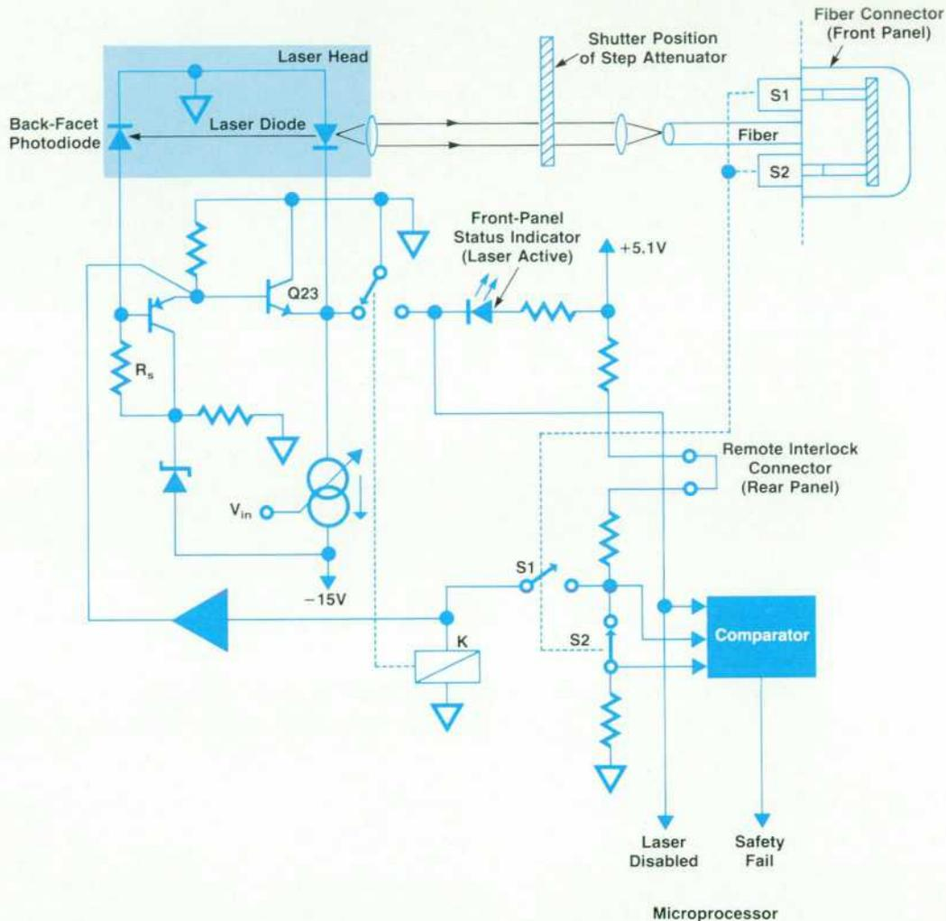
Fig. 15. This laser safety and protection circuit prevents laser damage caused by overdriving the laser. It also shuts off the light output when no optical fiber is connected.
