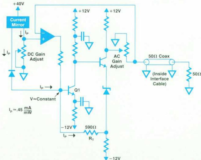
**Fig. 4.** The wideband transimpedance amplifier in the optical head is fast, offset compensated, and dc coupled.
