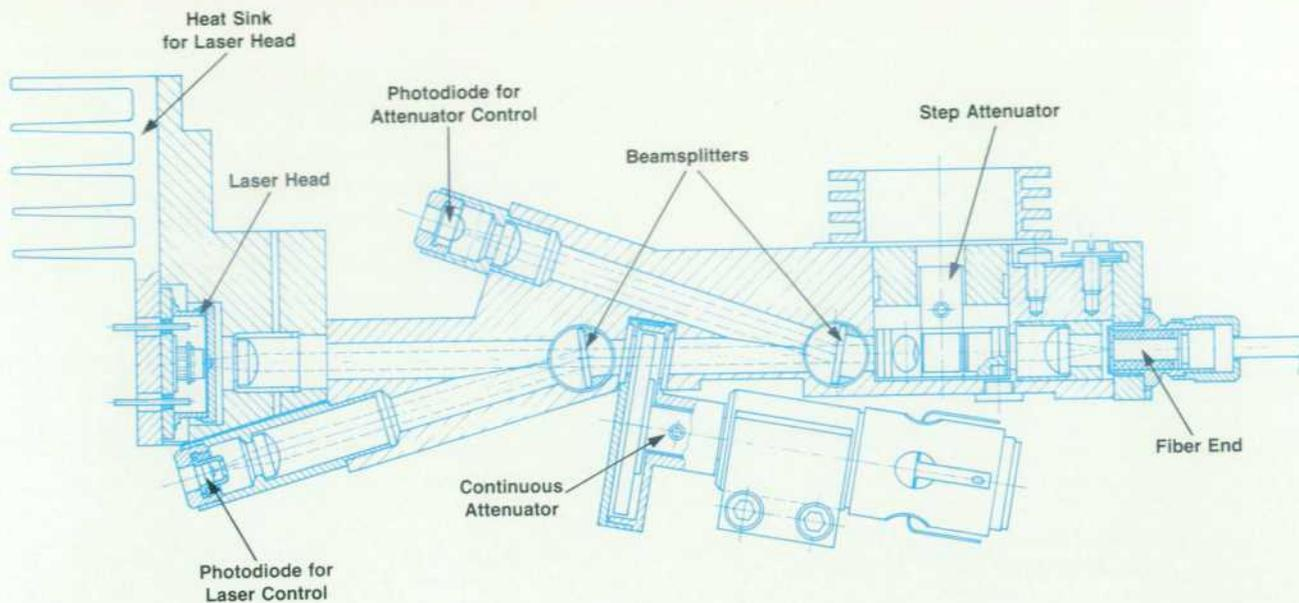
Fig. 16. Cross section of the optical bench.
