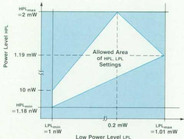
Fig. 12. Range of possible high and low power level settings. Automatic adjustments occur internally to keep the HP 8150A's operation in the allowed range.
