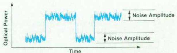
Fig. 14. Optical input signal disturbed by noise.
