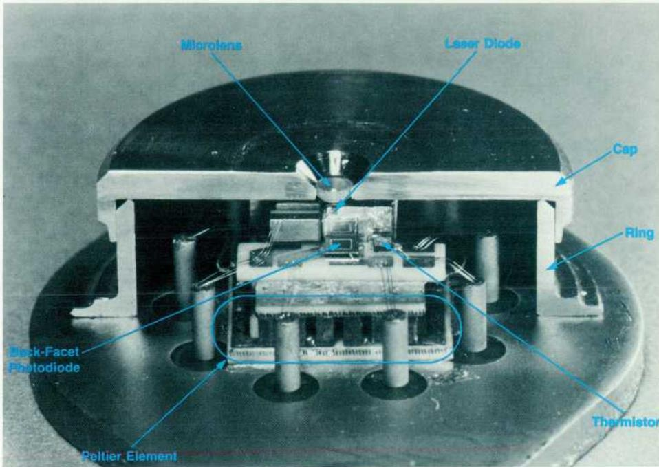
**Fig. 8.** The laser diode is mounted on a thermoelectric cooler and its temperature is controlled by a regulator circuit. This cutaway view of the laser head shows the Pelier cooler, the photodiode for monitoring the laser's back-facet emission, the thermistor, and the GaAlAs laser diode.
