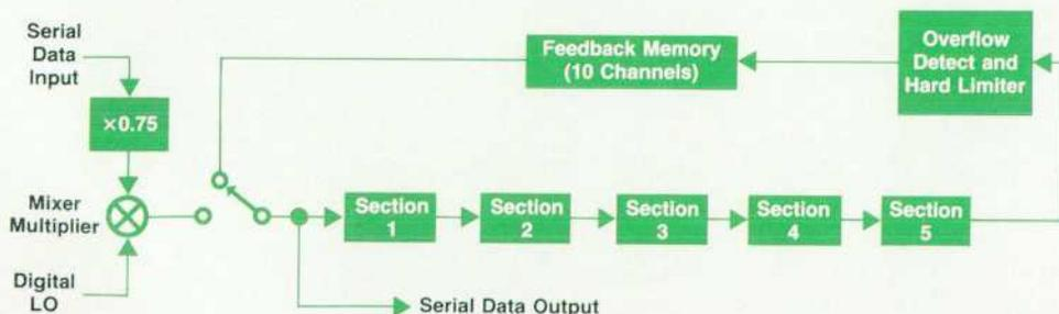
Fig. 7. Simplified block diagram of complete digital filter.
