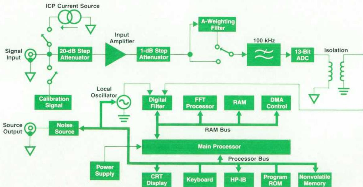
Fig. 1. Hardware block diagram of the HP 3561A.
