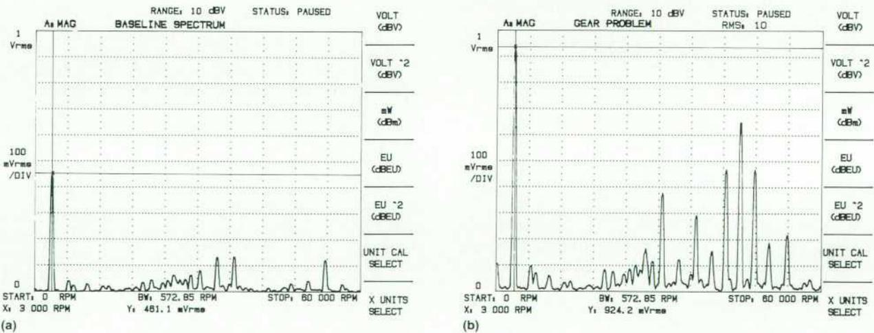
Fig. 2. (a) Baseline spectrum for a machine. (b) Later spectrum for machine of (a) showing the excessive response at the gear-mesh frequencies caused by a damaged gear.
