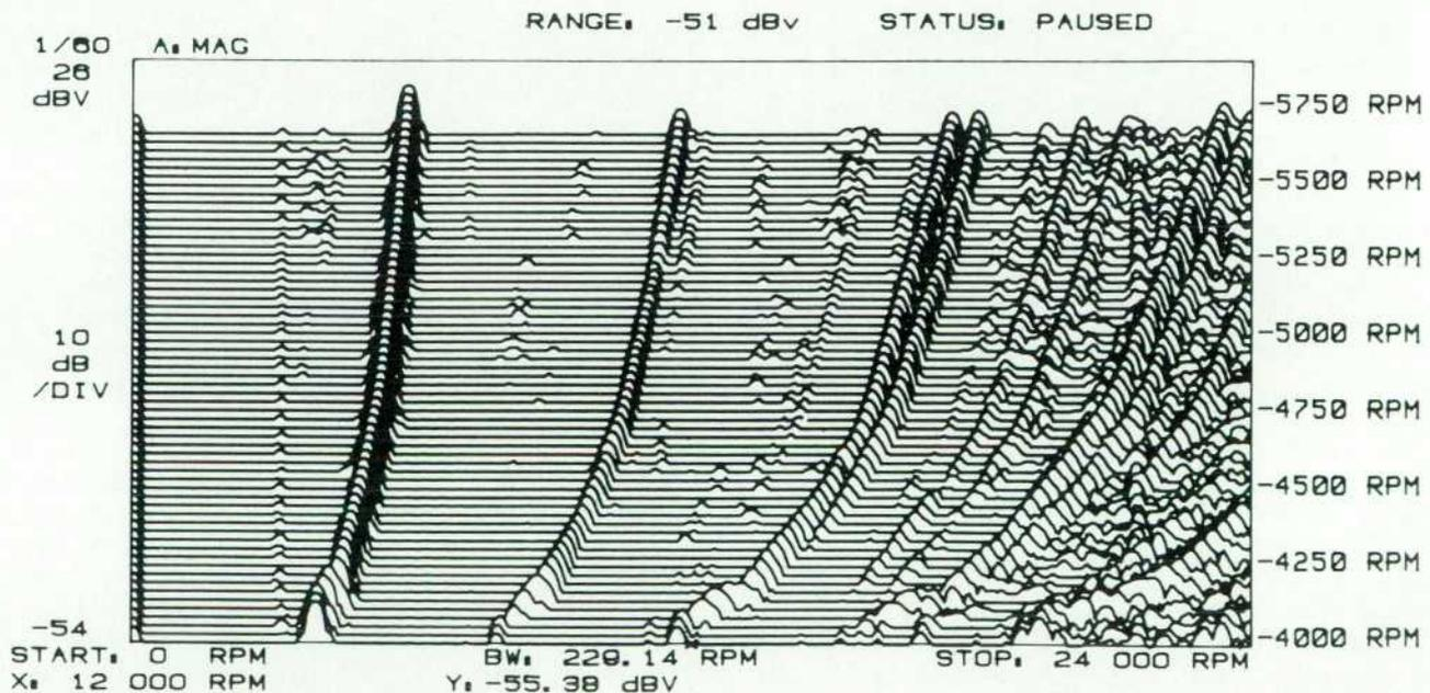
Fig. 5. Spectral map display. Up to 60 magnitude traces can be displayed simultaneously for studies of changes in the spectrum as a function of time, rpm, etc. These maps can be saved and recalled later from the optional nonvolatile bubble memory.
