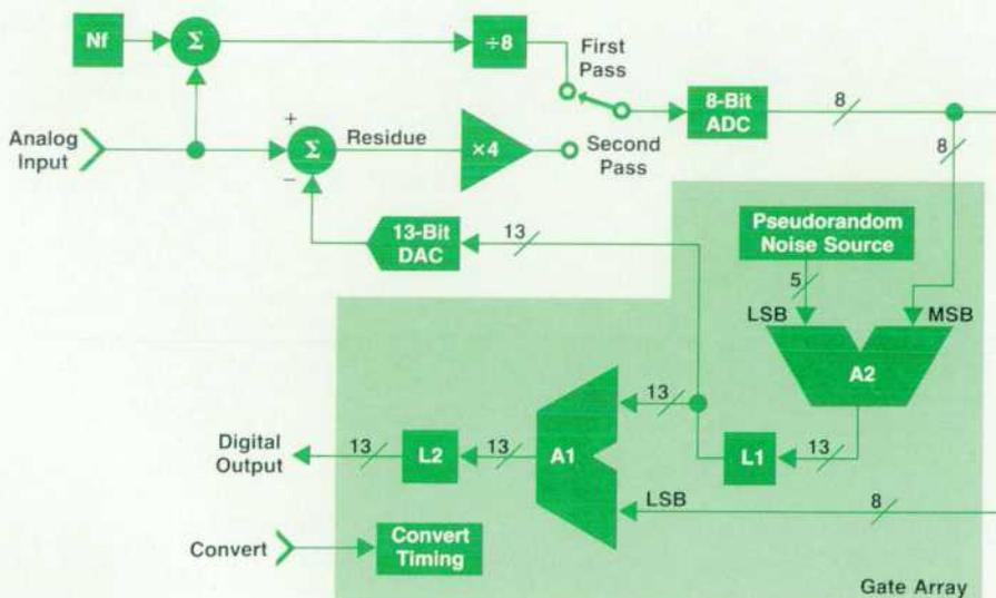
Fig. 4. ADC of Fig. 3 with dithering circuitry added. This circuitry is incorporated as a gate array design to keep the added cost low.
