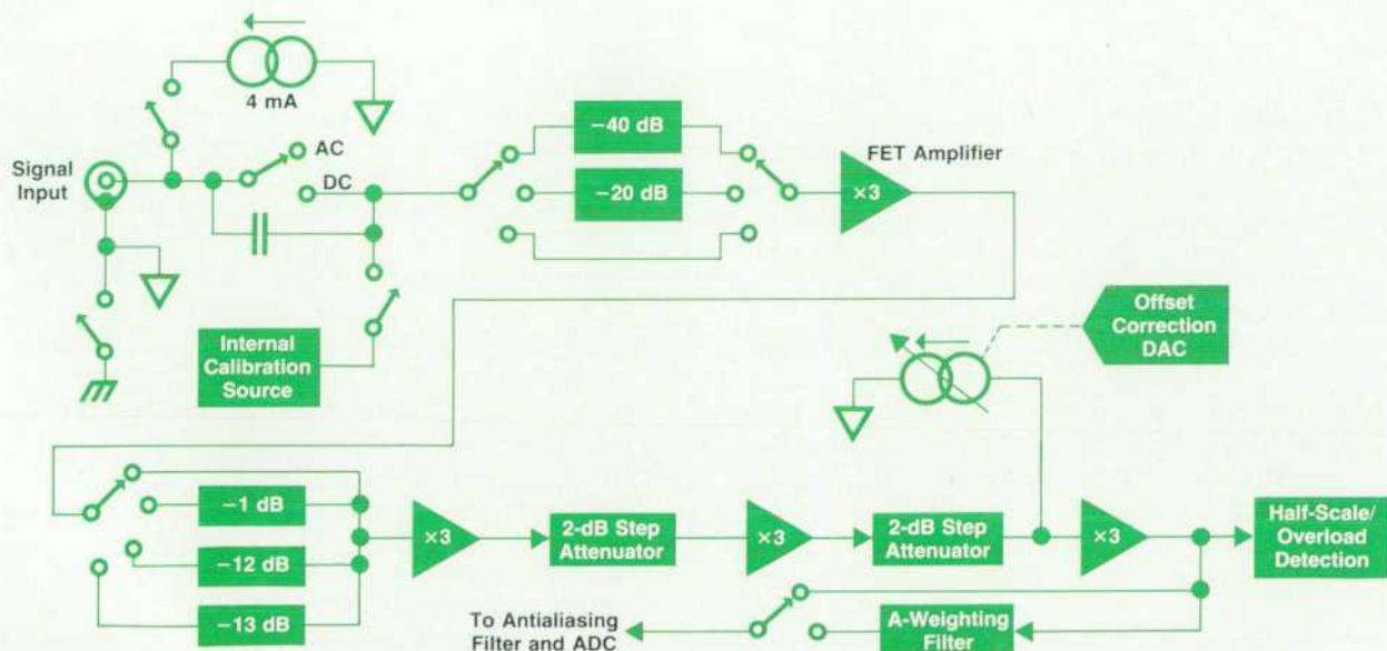
Fig. 2. Input circuitry of the HP 3561A.
