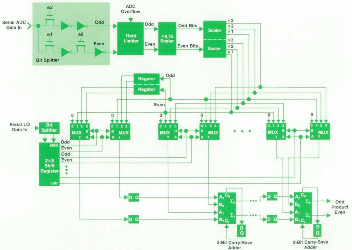
Fig. 4. Two's-complement paired-bit mixer multiplier.
