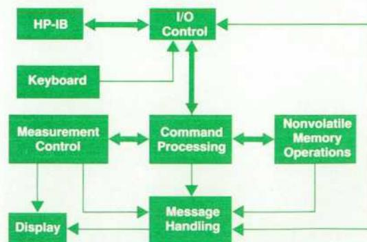
Fig. 1. Operating tasks for the HP 3561A's software.
