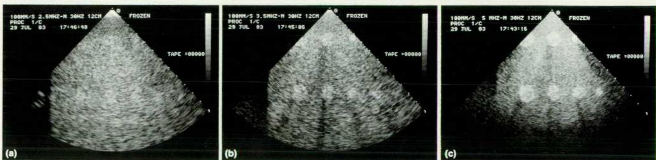
**Fig. 8.** Images made of a region of 20- $\mu\text{m}$  diameter scatterers surrounded by 7- $\mu\text{m}$  diameter scatterers using the 77020A System's (a) 2.5-MHz, (b) 3.5-MHz, and (c) 5.0-MHz transducers.
