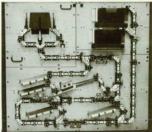
**Fig. 1.** To record the timing tracks and programs on the magnetic cards for the HP-75 Portable Computer, this production system was designed and built. It accepts blank cards in any possible orientation, rejects bad cards, and can record 2500 cards per hour.
