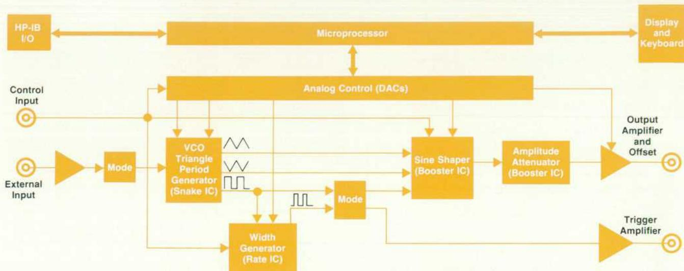
Fig. 8. Block diagram of the 8116A Pulse/Function Generator.
