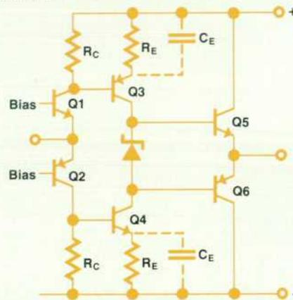
Fig. 3. Simplified schematic of the high-frequency amplifier.
