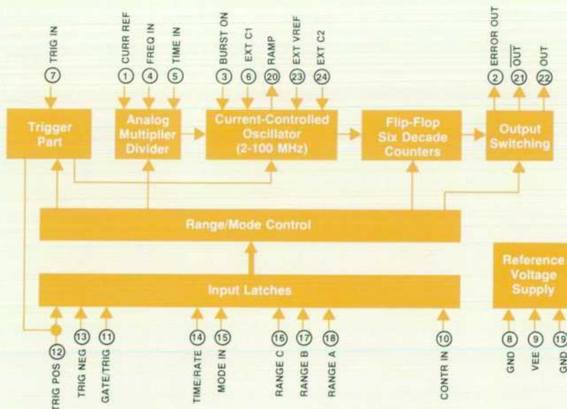
Fig. 1. Block diagram of the Rate IC, a monolithic timing circuit.
