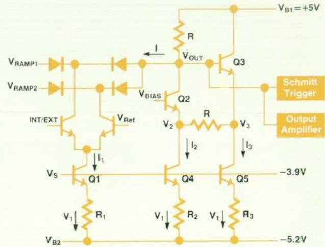
Fig. 9. This circuit on the Snake IC selects one of two possible ramp voltages to feed the Schmitt trigger and output amplifier. The current source  $I$  is usually realized with a single pnp transistor, but since the IC process used does not have adequate pnp transistors, this electronic pnp implementation was devised.
