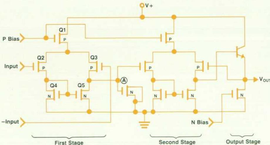
Fig. 1. CMOS operational amplifier circuit.
