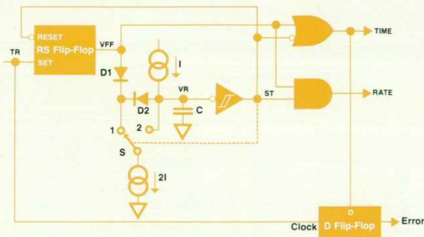
Fig. 3. Schematic of the 100% retriggerable pulse width generator and error detector of the Rate IC. The circuit can be restarted immediately after being stopped.
