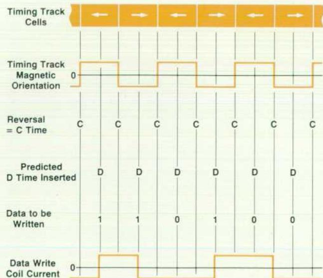
Fig. 7. Write operation timing for HP-75 card recorder.
