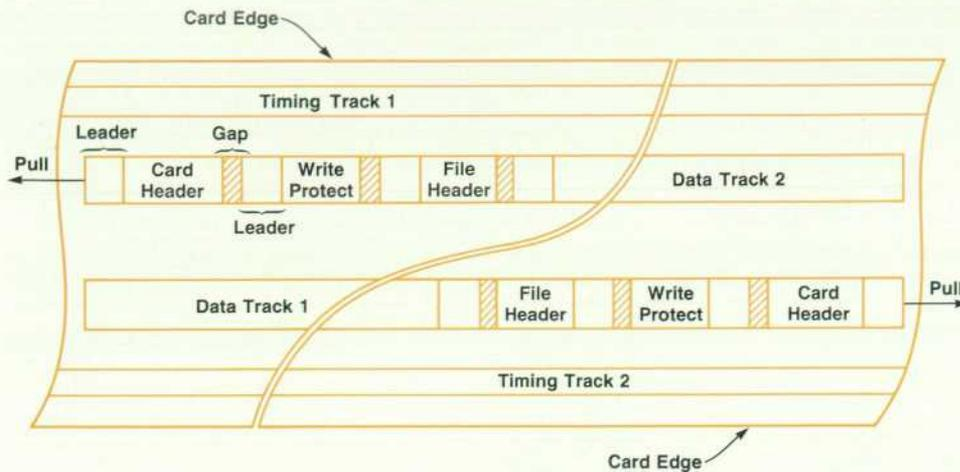
Fig. 2. Magnetic card track and data field format.
