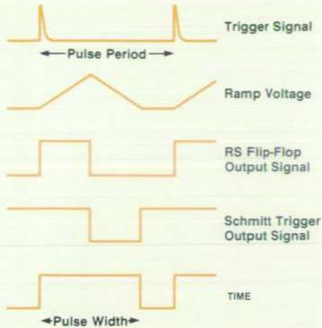
Fig. 4. Timing diagram for Fig. 3 in trigger mode.
