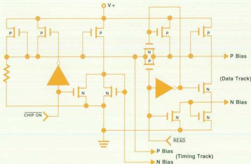
Fig. 3. Bias generation circuitry of CMOS card reader IC.
