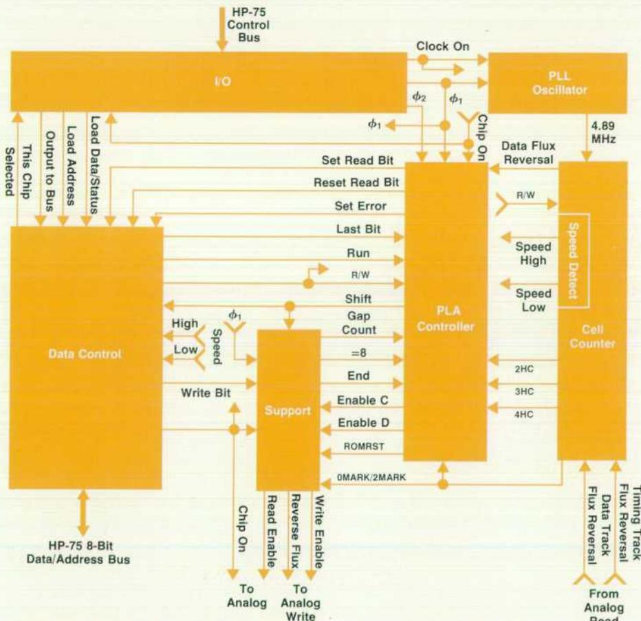
Fig. 8. HP-75 card reader digital block diagram.
