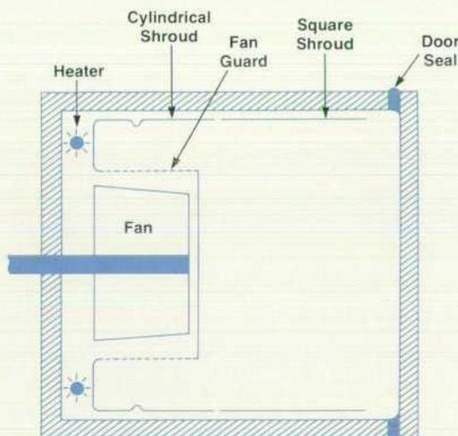
**Fig. 3.** 5790A oven design. Capillary columns mount in the annular space between the fan guard and the cylindrical shroud. Packed columns mount forward of the fan and inside the square shroud. The shrouds prevent mixing of controlled air with return air within the column area. The fan is a flat blade turning at high speed.
