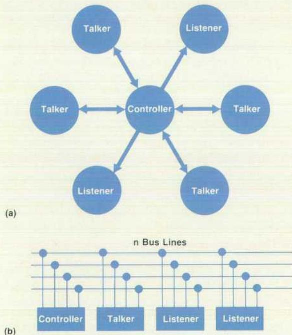
**Fig. 1.** (a) Star network architecture. The controller located at the center must have an I/O port for each of the other devices on this interface system. (b) Parallel bus network architecture. Each device on the bus must be able to drive the combined load presented by the other devices on the bus.
