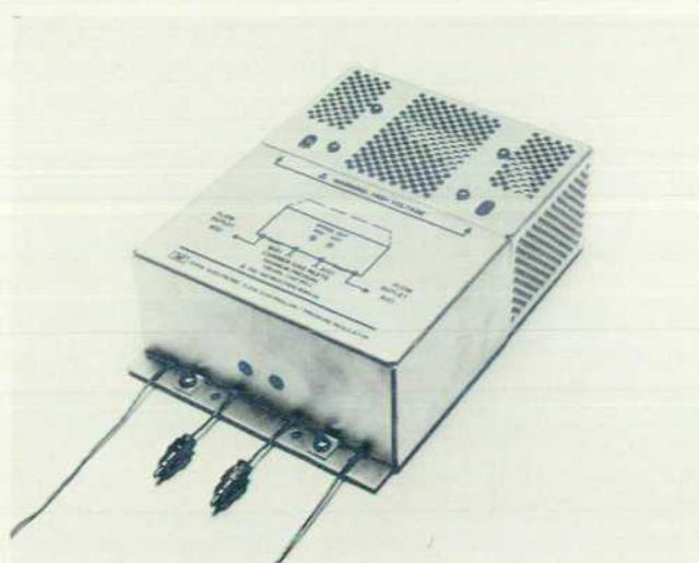
Fig. 10. Electronic flow controller module.
