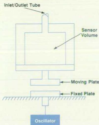
Fig. 4. Basic elements of the capacitive pressure transducer.
