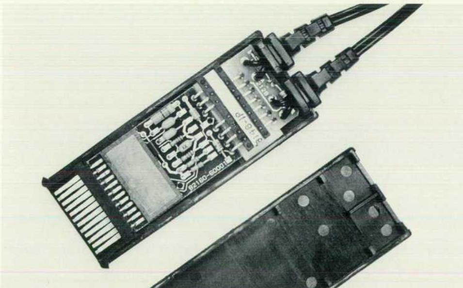
**Fig. 1.** Opened HP 82160A HP-IL Interface Module showing internal electronic components.
