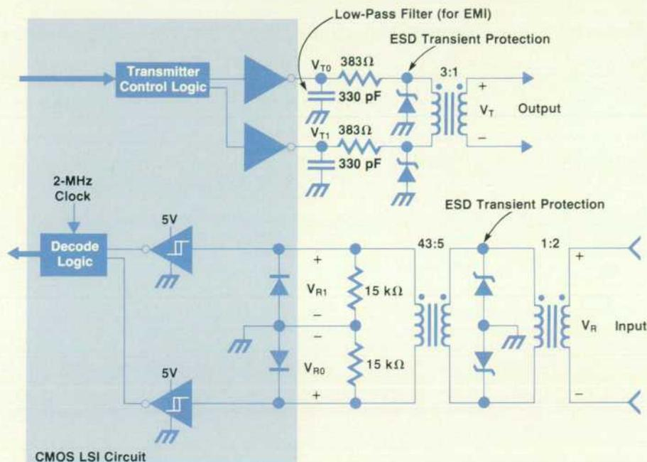
Fig. 7. Schematic of one implementation of the HP-IL electronics.
