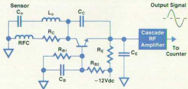
Fig. 7. Oscillator used in the capacitive pressure sensor.
