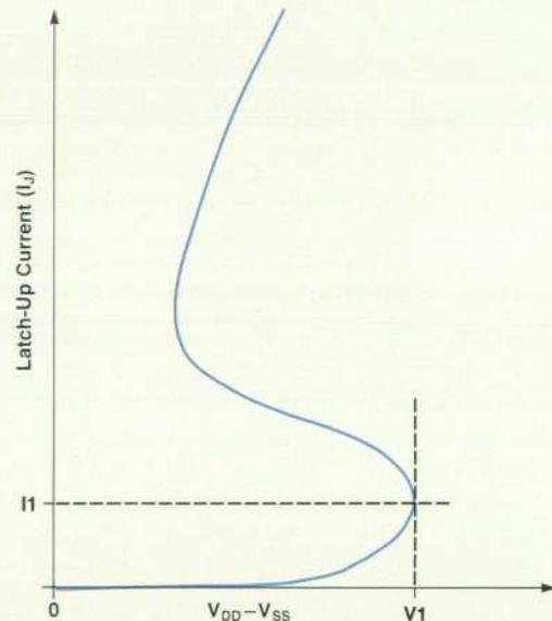
Fig. 3. I-V characteristic for circuit in Fig. 2.
