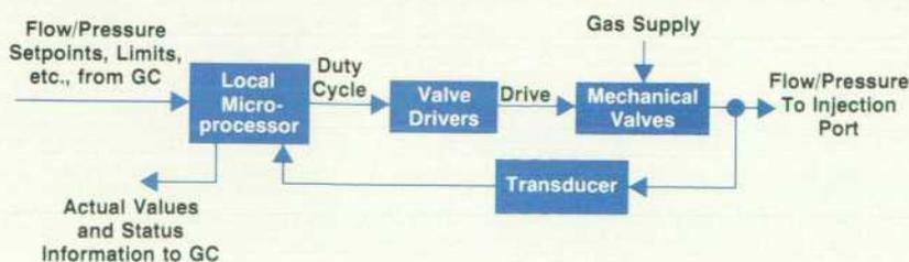
**Fig. 3.** Block diagram of the electronic flow controller.
