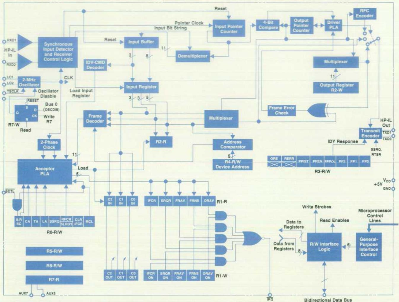
Fig. 1. Block diagram of HP-IL interface CMOS integrated circuit. This IC has an eight-bit bidirectional data bus for easy connection to most common microprocessors.
