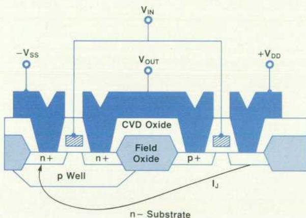
Fig. 1. Cross section of CMOS inverter structure.
