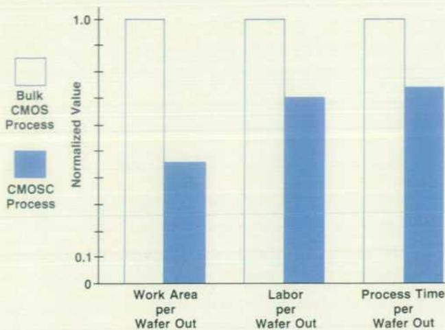
**Fig. 6.** Efficiency of CMOS clean-room use compared to previous bulk CMOS process. Data is based on a mature process in a facility running at full capacity. A wafer out means one wafer of devices fully processed into integrated circuits.
