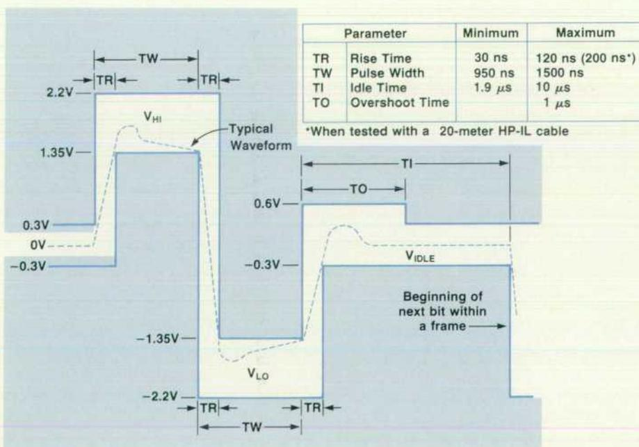
Fig. 6. HP-IL transmitter waveform specification (open circuit). While only a logical-one bit is shown, all logical bits must conform to the same basic specifications with polarity changes made where appropriate.
