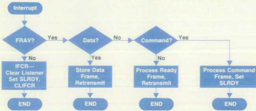
Fig. 4. Simplified flowchart of the response of a listener on the HP-IL.
