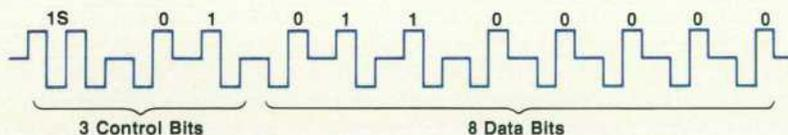
Fig. 3. The HP-IL uses an eleven-bit message frame consisting of three control bits and eight data bits. The first control bit also serves as a sync bit.
