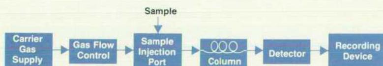
**Fig. 1.** Schematic representation of a gas chromatographic system. A carrier gas under pressure moves a vapor sample from the injection port through the column where the sample is separated into its components. The detector converts the amount of sample reaching it to an electrical signal, which is recorded as a function of time. Different components of the sample reach the detector at different times and are seen as peaks in the record.
