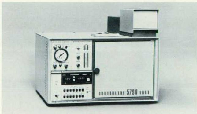
**Fig. 1.** The HP 5790A Gas Chromatograph is designed for operational simplicity and high retention time reproducibility. Its features include an advanced oven design, a large digital display, easy setpoint control, storage of setpoint methods, memory protection, stopwatch, valve control, and built-in diagnostics.
