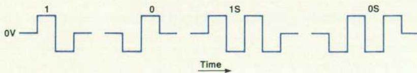
Fig. 2. HP-IL definitions for logical bits 1, 0, 1S, and 0S.
