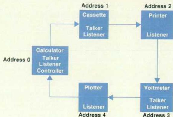
**Fig. 2.** Typical Hewlett-Packard Interface Loop system. Messages are circulated around a loop. Only controllers and talkers can originate a message but all devices can retransmit a received message. Each device receives the message, acts upon it if required, and retransmits it to the next device until the message returns to its originator. Thus, each HP-IL device only has to drive one other device, regardless of the number of devices on the loop.
