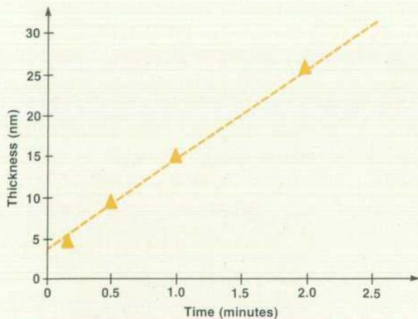
**Fig. 3.** The deposited thickness of a very thin silicon-nitride film on a polycrystalline silicon surface versus deposition time. The y-intercept is caused by the very rapid formation of a 3-nm-thick native oxide layer before the deposition cycle.
