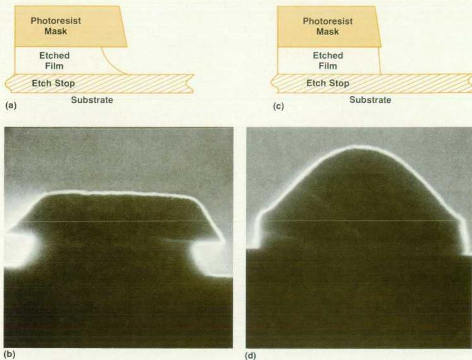
**Fig. 2.** Comparison of the etch profiles for isotropic and anisotropic etching. (a) Diagram of isotropic etch profile. (b) SEM photograph of actual isotropic profile. (c) Diagram of anisotropic etch profile. (d) SEM photograph of actual anisotropic profile.
