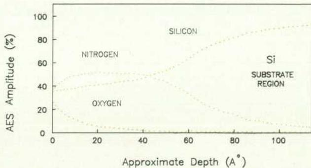
**Fig. 1.** Profile of oxynitride film composition versus depth obtained by Auger analysis. Film was grown by plasma-enhanced nitridation at  $400^\circ\text{C}$  using  $NH_3$  gas at 0.5 torr and a power level of 400 W for 2 hours.
