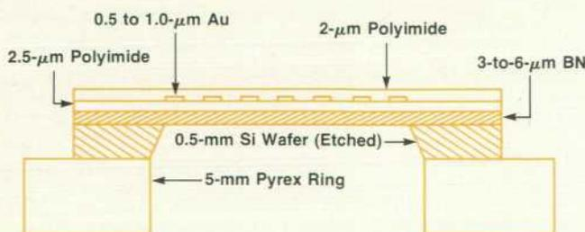
Fig. 3. Cross section of typical X-ray mask structure.
