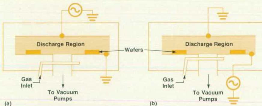
Fig. 4. Diagram of side view of parallel plate reactors in (a) the plasma mode and (b) the reactive-ion-etch mode. The gas flows radially inward over the wafers that are in intimate contact with the plasma.
