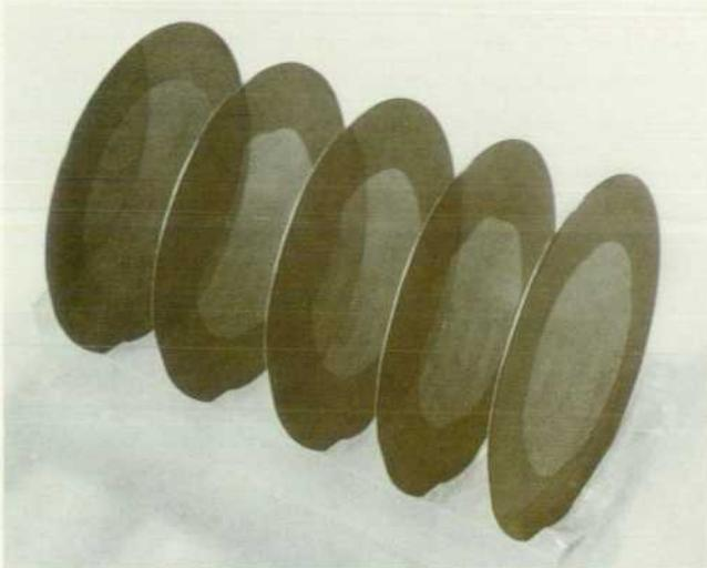
Fig. 5. Photo of boron-nitride pellicles.
