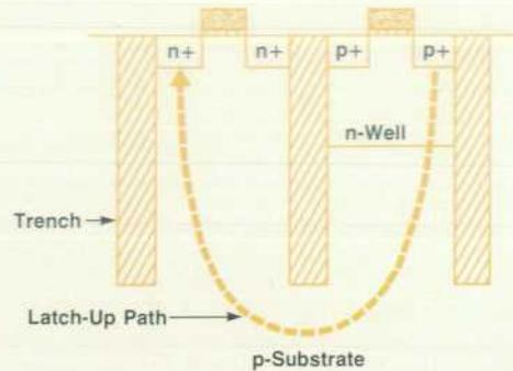
**Fig. 2.** By etching a deep trench between the two transistors in Fig. 1 and refilling the trench with a dielectric material, the transistors can be spaced closer together, but the path for regenerative feedback will still remain long enough to prevent latch-up.
