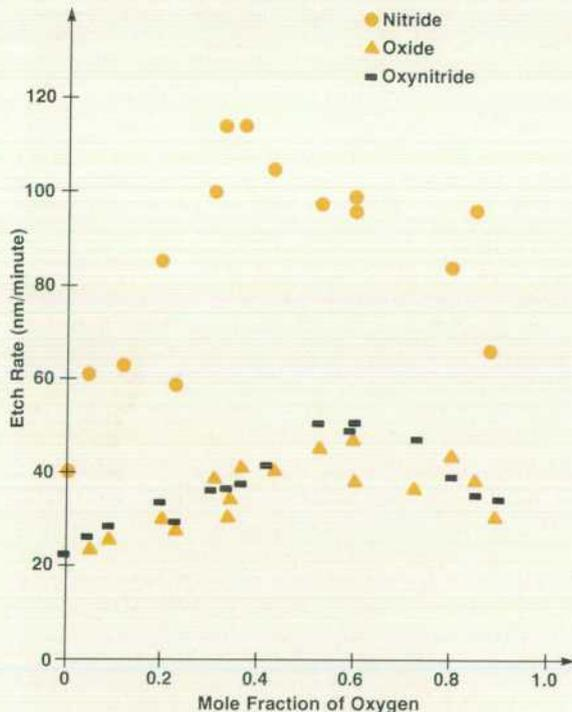
Fig. 2. The etch rate of standard silicon-nitride, silicon-oxynitride, and silicon-dioxide films in C<sub>2</sub>F<sub>6</sub>/O<sub>2</sub> plasma.
