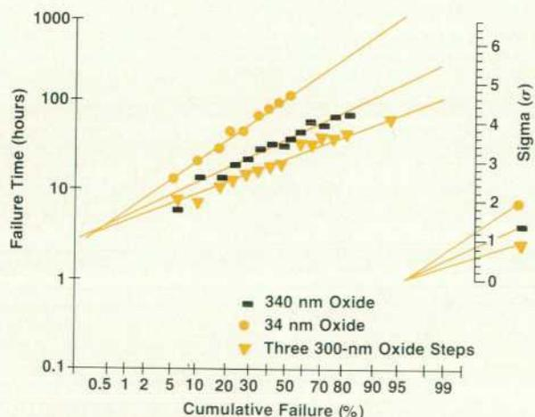
**Fig. 4.** Accelerated electromigration life-test plots of sputtered Al-Si (2%)  $2\text{-}\mu\text{m}^2$  conductors,  $100\ \mu\text{m}$  long. The stress conditions are a current density of  $1 \times 10^6$  A/cm<sup>2</sup> and a temperature of 220°C. The different underlying substrate surfaces are (●) 34-nm-thick planar SiO<sub>2</sub>, (■) 340-nm-thick planar SiO<sub>2</sub> and (▼) the same surface as (■) with three vertical-walled, 300-nm-high SiO<sub>2</sub> steps.
