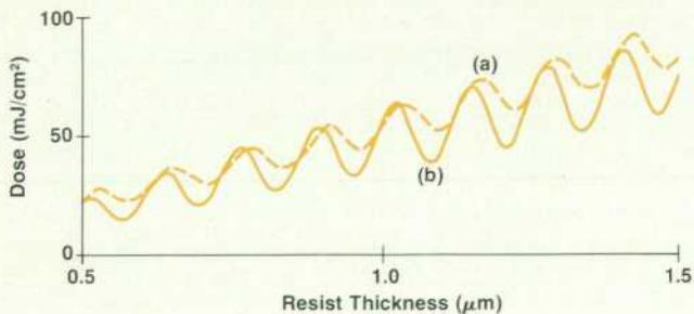
**Fig. 2.** The exposure energy density (dose) required at a wavelength of 436 nm to achieve 1- $\mu\text{m}$ -wide lines and spaces in HPR 204 positive resist on (a) silicon and (b) aluminum surfaces for numerical aperture  $NA=0.28$ , perfect focus, and partial coherence factor  $\sigma=0.7$ .
