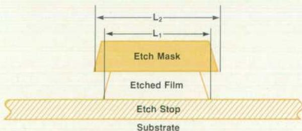
Fig. 1. A typical cross section of an integrated circuit feature. For an anisotropic etch  $L_1 = L_2$  and  $L_2$  is not altered by the etch process. In most processes the ratio of the film etch rate to the etch-stop-material etch rate varies from 5:1 to 10:1. The ratio of the film etch rate to the mask etch rate is similar.
