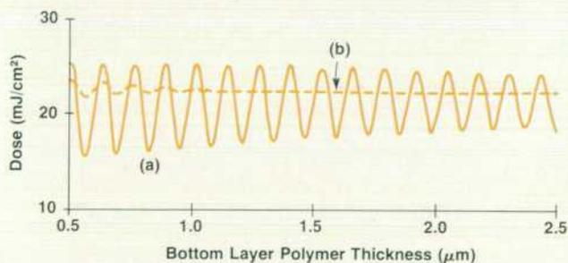
**Fig. 5.** Nominal dose versus bottom polymer thickness for the trilayer system of Fig. 4 on an aluminum substrate using (a) HPR 204 positive resist and (b) HPR 204 containing 1.5% dye for the bottom polymer. Simulations are for 1- $\mu\text{m}$ -wide lines and spaces under perfect focus conditions.
