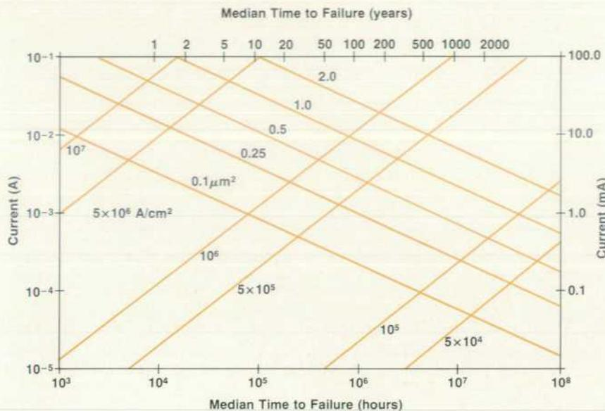
**Fig. 2.** Design rules for sputtered Al-Si(2%)-Cu(4%) metallization alloyed at 450°C and operating at 90°C. The axes give median time to failure  $t_{50}$  and current. Constant-current-density and conductor cross-sectional-area contours allow easy selection of desired conductor size or current density.
