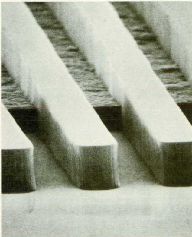
**Fig. 8.** Edge profile of trilayer process using spin-on glass for the intermediate layer covering 1.0- $\mu\text{m}$ -high aluminum steps. Profile is shown after reactive ion etching of bottom polymer layer.
