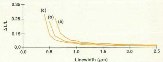
**Fig. 10.** The fractional linewidth variation ( $\Delta L/L$ ) as a function of linewidth in micrometers for a  $\pm 5\%$  variation in exposure energy for the curves of Fig. 9. Each optical system was degraded by  $\lambda/[4(NA)^2]$  of focus error.
