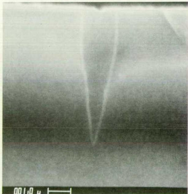
**Fig. 3.** Cross-sectional microphotograph of a refilled trench.
