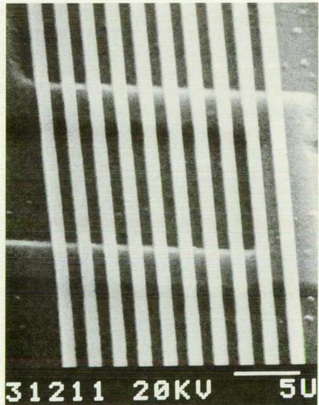
**Fig. 7.** 1- $\mu\text{m}$ -wide lines and spaces in trilayer resist over 0.5- $\mu\text{m}$ -high aluminum steps after reactive ion etch. 2.0- $\mu\text{m}$ -thick HPR 204 positive resist containing 1.5% dye is used for the bottom polymer layer.
