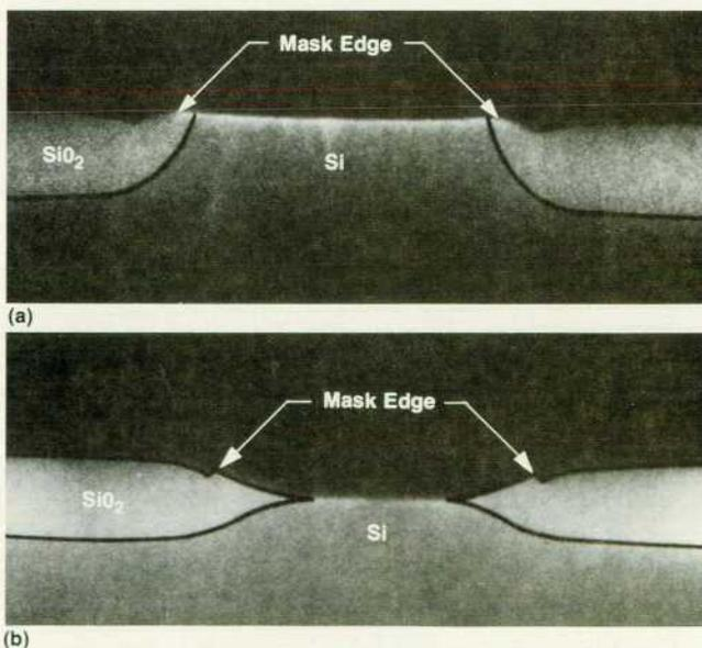
**Fig. 2.** Microphotograph of (a) SWAMI structure compared to (b) LOCOS structure before gate oxidation.
