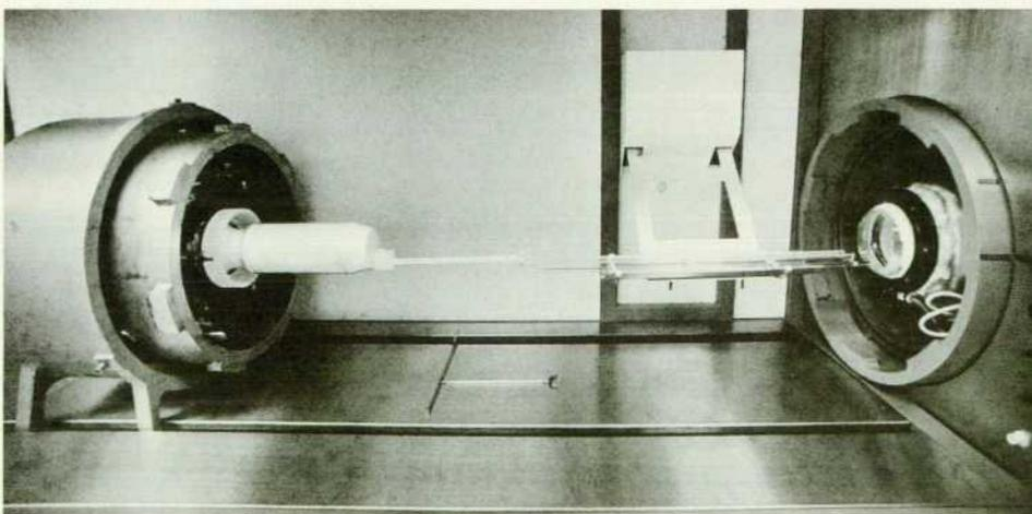
**Fig. 1.** Operator's view of HP's high-pressure oxidation system. After the quartz carrier (center) is loaded with wafers to be oxidized, it is inserted into the chamber on the right and the chamber is sealed with the end cap shown on the left.
