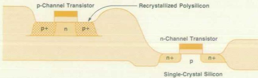
Fig. 5. Schematic cross section of a CMOS transistor pair used in an integrated circuit. Any possibility of latch-up is avoided by completely surrounding one type of transistor by insulating silicon dioxide.
