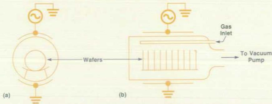
Fig. 3. Diagram of barrel plasma reactor. (a) End view. (b) Side view.
