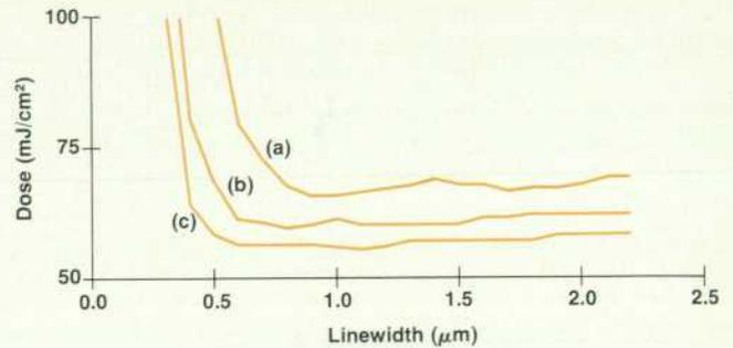
**Fig. 9.** The nominal exposure dose as a function of linewidth in micrometers for (a)  $\lambda=436 \text{ nm}$ ,  $NA=0.28$ ; (b)  $\lambda=405 \text{ nm}$ ,  $NA=0.35$ ; and (c)  $\lambda=240 \text{ nm}$ ,  $NA=0.25$  ( $\sigma=0.7$ , all cases). Simulation parameters (see reference 11):  $A=0.57 \mu\text{m}^{-1}$ ,  $B=0.08 \mu\text{m}^{-1}$ ,  $C=0.01 \text{ cm}^2/\text{mJ}$ ,  $F_1=0.179$ ,  $F_2=-0.346$ ,  $F_3=0.168$ .
