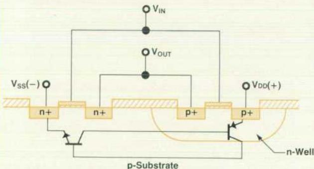
**Fig. 1.** Cross section of CMOS inverter structure with the two-transistor equivalent circuit superimposed. This transistor combination can act as a lateral SCR structure that will turn on when large currents are passed, if the spacing between the transistors is small enough to permit regenerative feedback.
