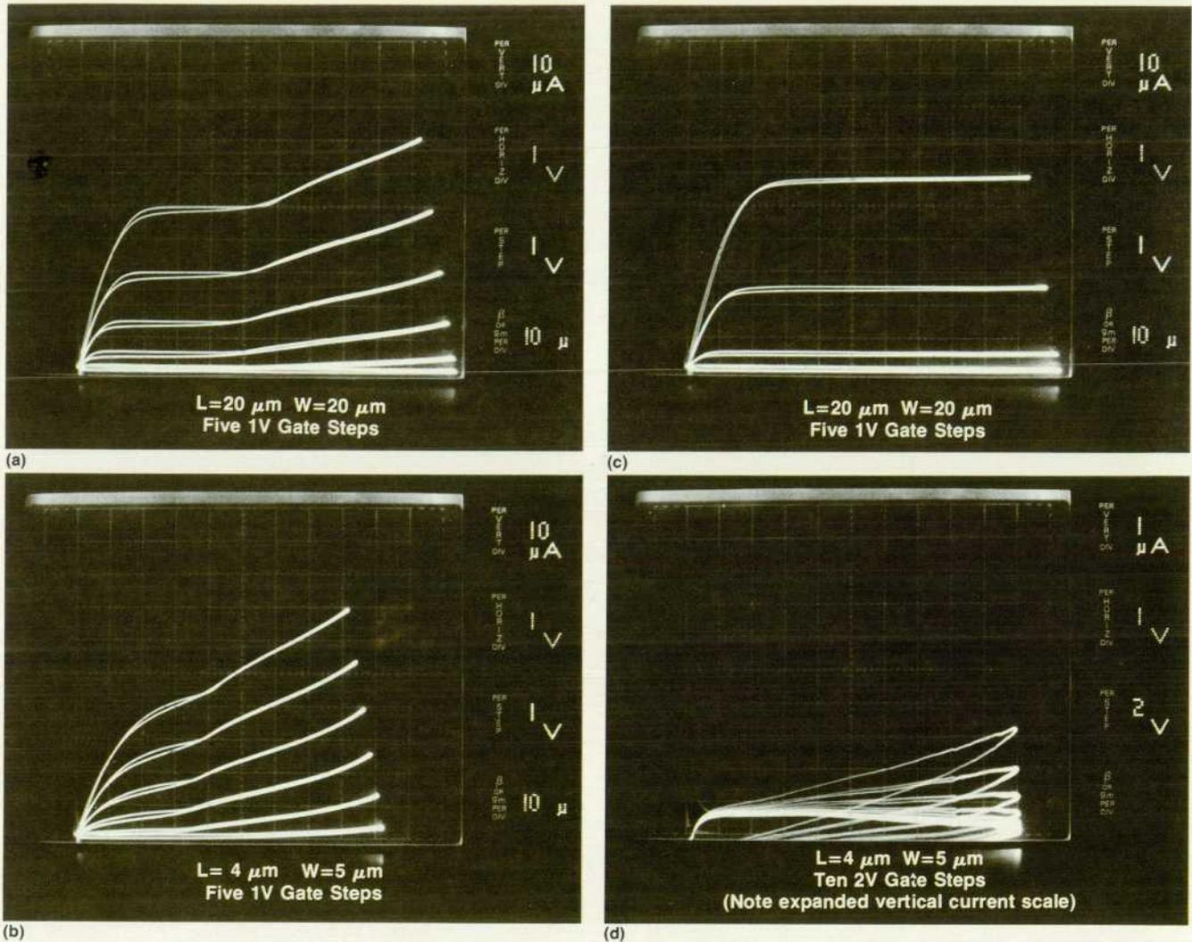
**Fig. 4.** Source-drain characteristics of (a) large-geometry and (b) small-geometry transistors fabricated in recrystallized polysilicon, along with the characteristics of (c) single-crystal-silicon and (d) fine-grain-polysilicon transistors (see reference 2).
