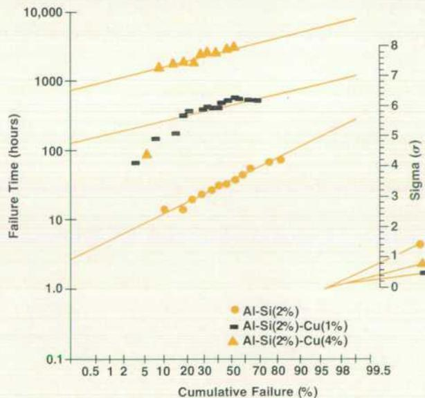
**Fig. 3.** Accelerated electromigration life-test plots (log-normal paper) of Al-Si(2%) alloys for different copper concentrations; (●) 0%, (■) 1%, and (▲) 4% Cu. Test done at 220°C and a current density of  $10^6 \text{ A/cm}^2$ .  $t_{50}$  is found from the intersection of the 50% cumulative failure line and the straight-line fit of the data points.
