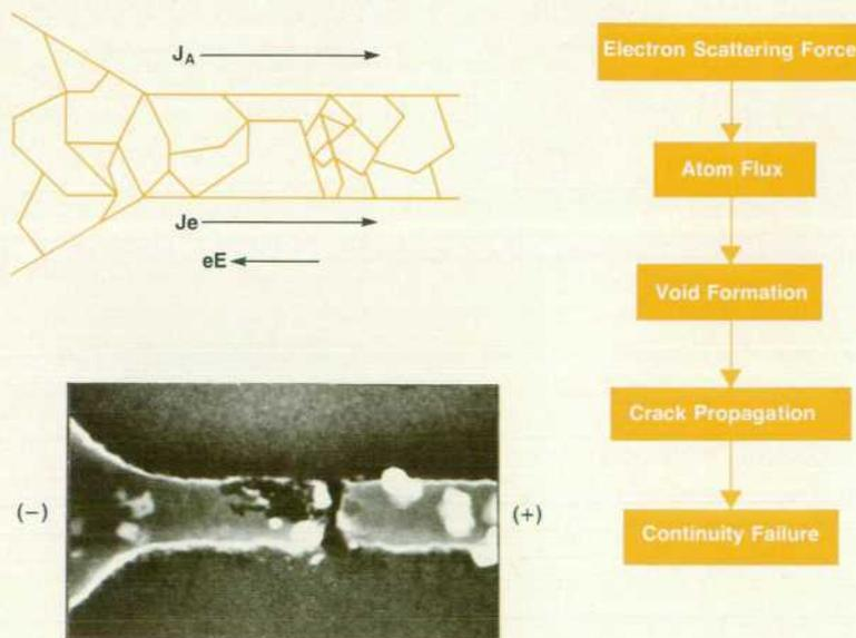
**Fig. 1.** Electromigration mechanism showing an idealized conductor (upper left) with directions of electron flux  $J_e$ , electrostatic force  $eE$  and resultant atomic flux  $J_A$ . Scanning electron microscope photograph (lower left) of void formation to the left of the break and accumulation of material in the form of hillocks to the right. The right half of this figure outlines the failure process.
