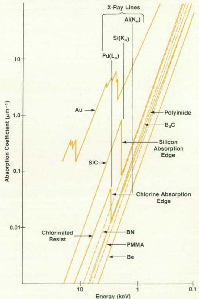
Fig. 4. Absorption coefficient versus X-ray wavelength for several materials.
