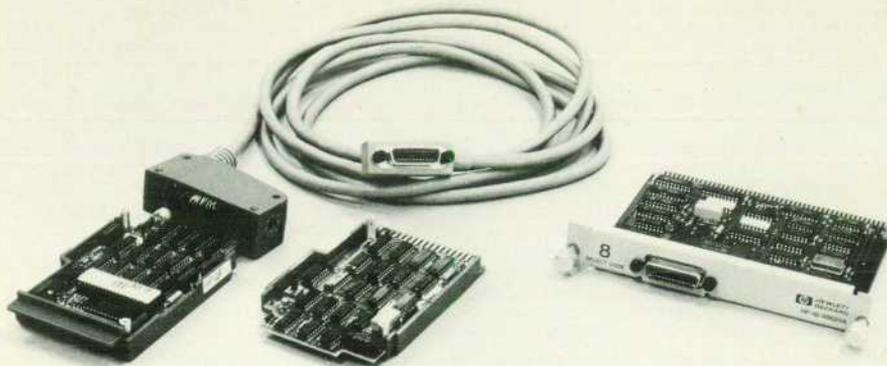
Fig. 1. Physical comparison of the older 980xx series I/O card (on the left) and the new I/O card (on the right) developed for the 9826A and 9836A.
