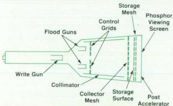
Fig. 1. Simplified variable persistence CRT construction.
