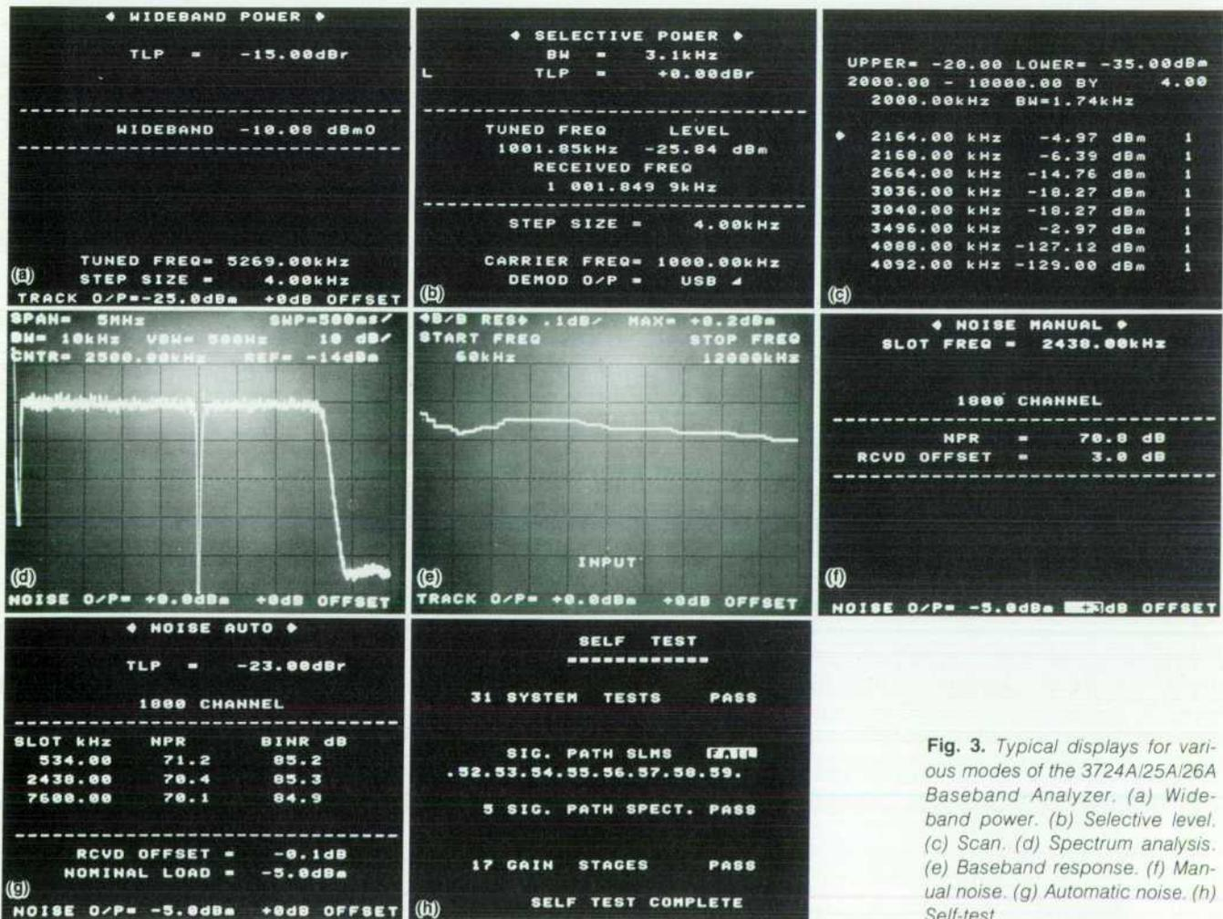
Fig. 3. Typical displays for various modes of the 3724A/25A/26A Baseband Analyzer. (a) Wideband power. (b) Selective level. (c) Scan. (d) Spectrum analysis. (e) Baseband response. (f) Manual noise. (g) Automatic noise. (h) Self-test.
