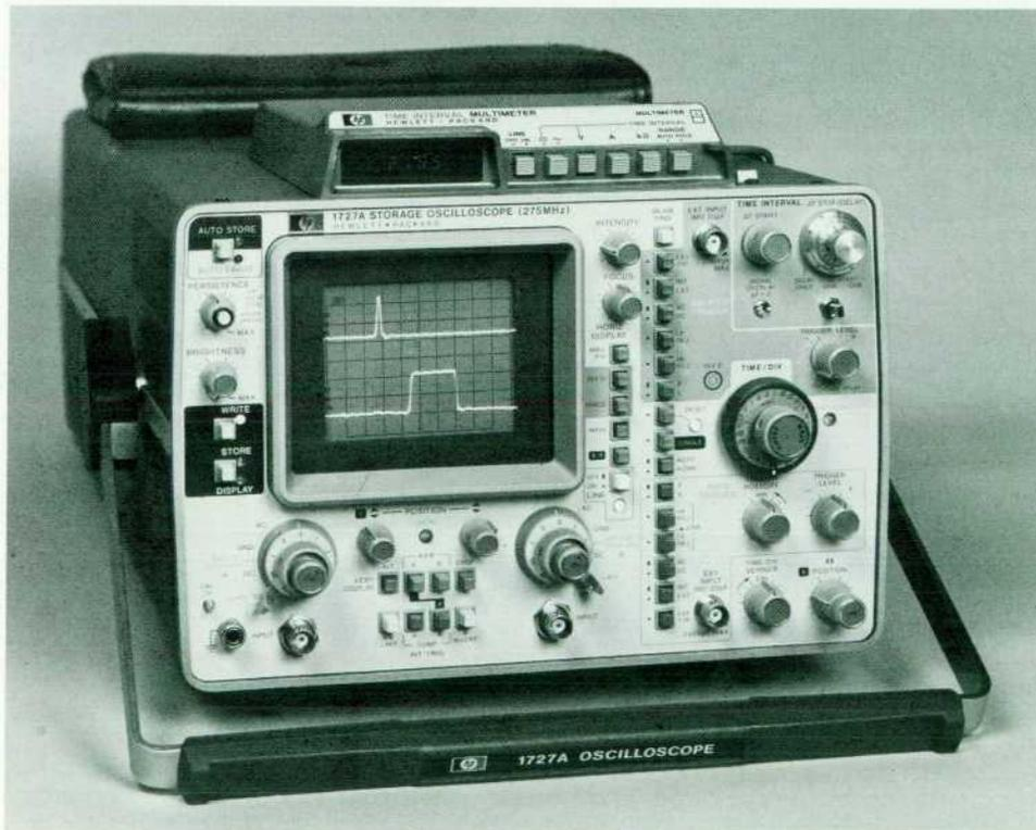
**Fig. 1.** With its 275-MHz bandwidth, variable persistence, and high 2000-cm/ $\mu$ s writing capability, Model 1727A Oscilloscope can capture single-shot or low-repetition-rate signals that would be difficult to observe otherwise.
