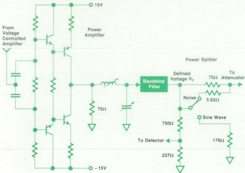
Fig. 5. Power amplifier and power splitter circuit.
