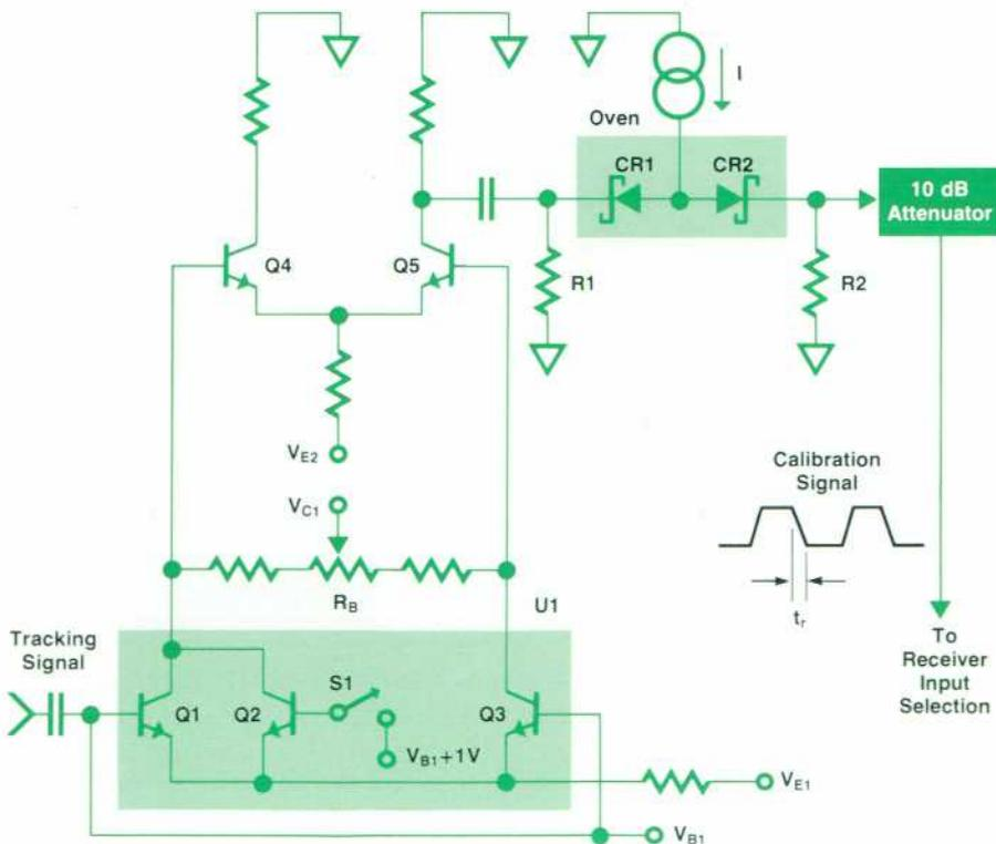
**Fig. 11.** Simplified schematic of calibration amplifier.
