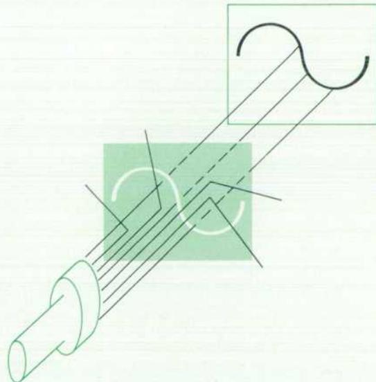
Fig. 2. Once a trace is written on the storage mesh of a variable persistence CRT, flood gun electrons can penetrate the storage mesh in the written areas and continue on to the phosphor. Flood gun electrons are repelled by unwritten areas of the storage mesh.
