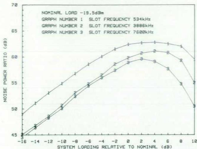
Fig. 4. White-noise V-curves. Using the HP-IB interface and a plotter, one can directly record many measurements in a convenient format.
