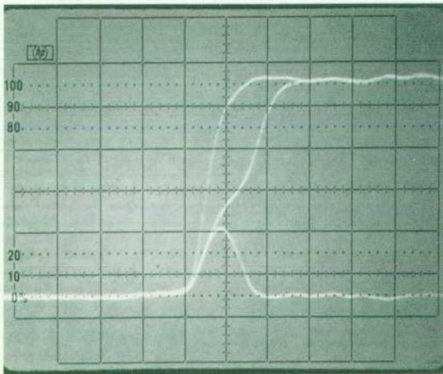
**Fig. 3.** D flip-flop setup violation showing a metastable state. (Sweep speed = 5 ns/div.)
