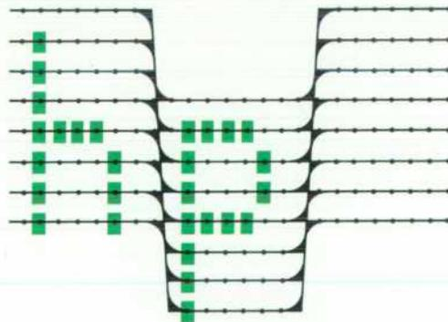
**Fig. 3.** A spare row bit in the character ROM is used to shift the vertical raster to generate a lowercase p as shown above.
