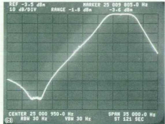
Fig. 8. (a) One section of the two-stage first-IF crystal filter in the selective circuit path. T1 is both a component of the lattice structure of the filter and a matching transformer for the low-noise amplifier that follows. (b) Filter response.
