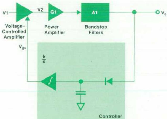
Fig. 2. Leveling-loop block diagram.
