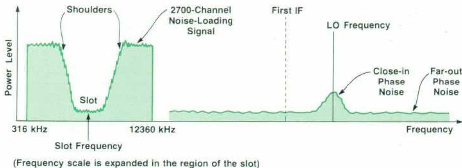
Fig. 7. The LO mixes the slot frequency into the first IF. The shoulders of the slot mix with the close-in phase noise of the LO to appear in the IF and the rest of the noise-loading signal mixes with the far-out noise sidebands of the LO and also appears in the IF.
