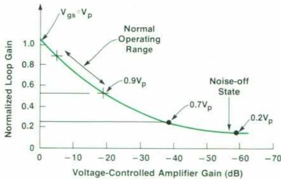
Fig. 4. Loop-gain variation with voltage-controlled amplifier gain.
