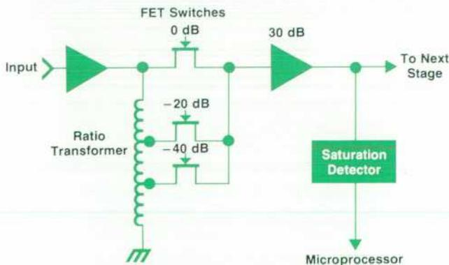
Fig. 9. One section of the programmable-gain amplifier.
