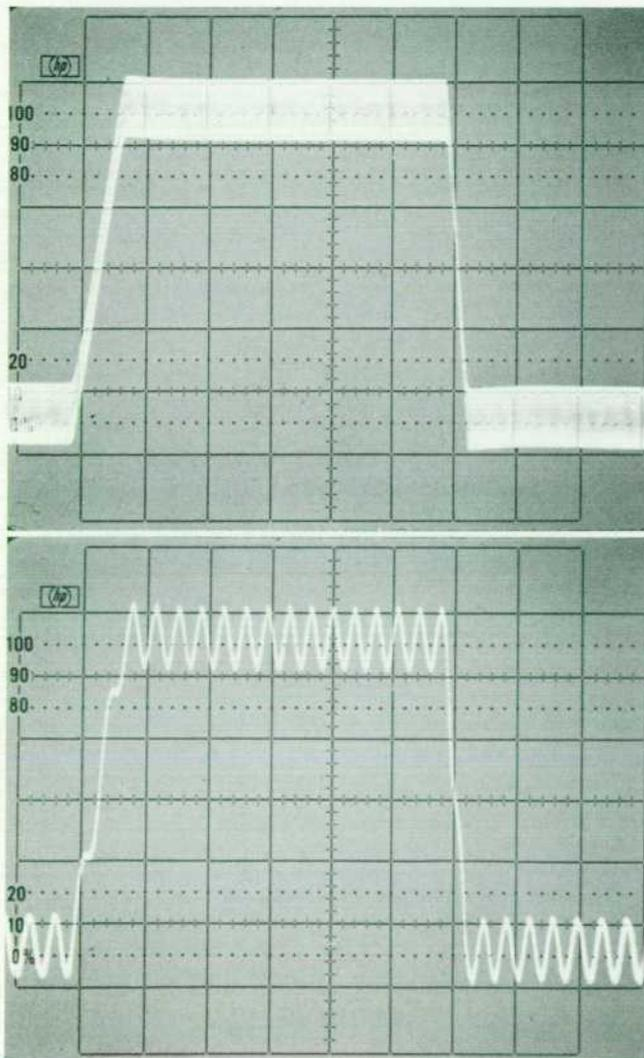
**Fig. 8.** Auto-erase mode is a repetitive single-shot mode that provides a continuous sequence of updated displays. Here it helps in the observation of noise on a pulse train. Top: conventional display. Bottom: auto-erase display.
