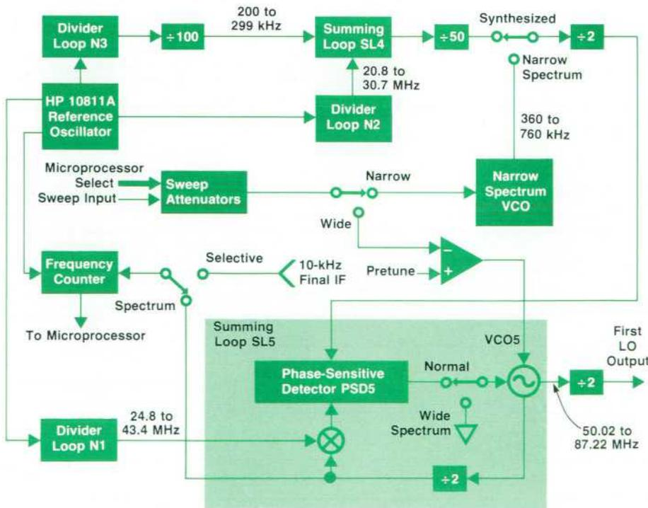
Fig. 5. Block diagram of first-LO section.
