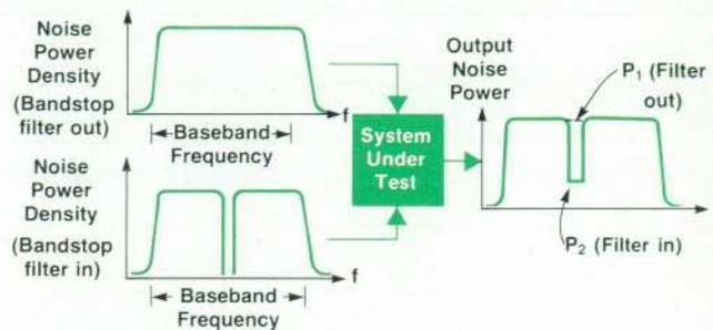
**Fig. 1.** By measuring the noise power output from a system under test with a white noise input signal with ( $P_2$ ) and without ( $P_1$ ) a narrow bandstop filter switched in, the noise power ratio (NPR) can be determined from the equation  $NPR = 10 \log (P_1/P_2)$  dB.
