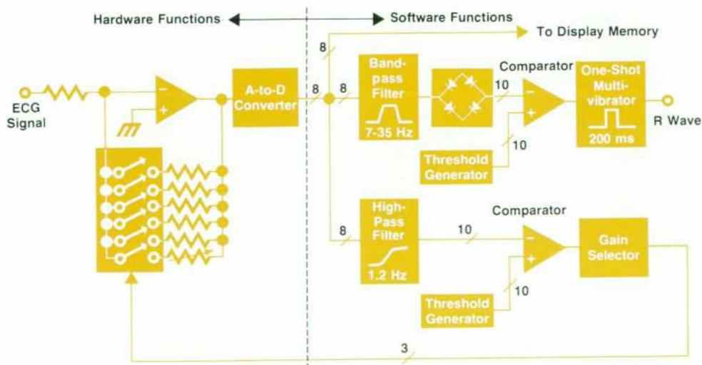
Fig. 9. Block diagram of heartbeat detection circuitry.
