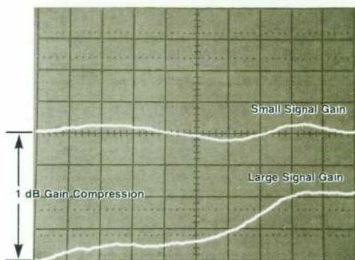
**Fig. 6.** The alternate sweep function causes the 8350A to switch, on successive sweeps, between the current front-panel settings and any of nine front-panel states stored in memory. This makes it possible to observe a device's responses to two different stimulus conditions on the same display.
