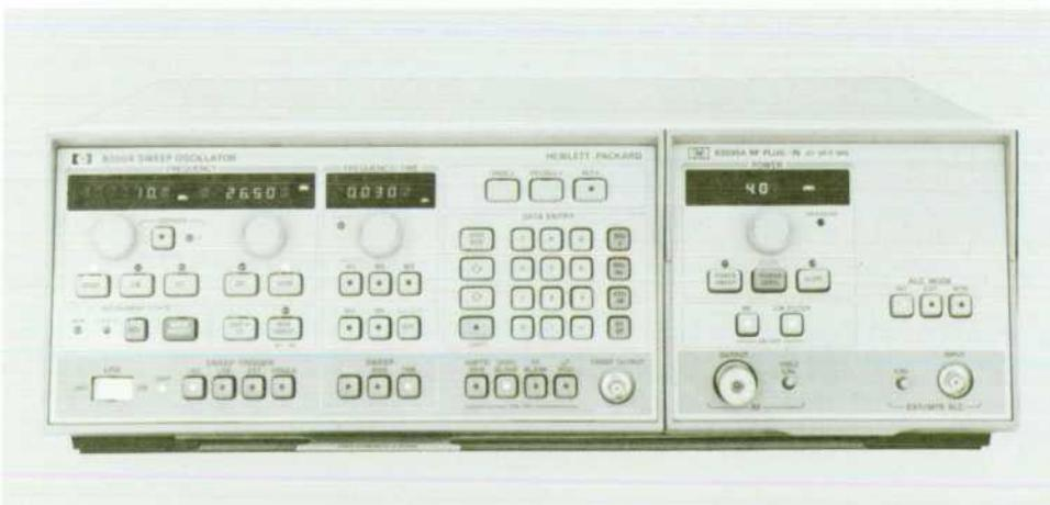
**Fig. 1.** Model 8350A Sweep Oscillator is a fully programmable instrument that can accept various RF and microwave plug-in modules to provide broadband frequency sweeps (0.01 to 26.5 GHz with the 83595A RF Plug-in shown), calibrated output power, and high frequency accuracy ( $\pm 10$  MHz at 20 GHz).
