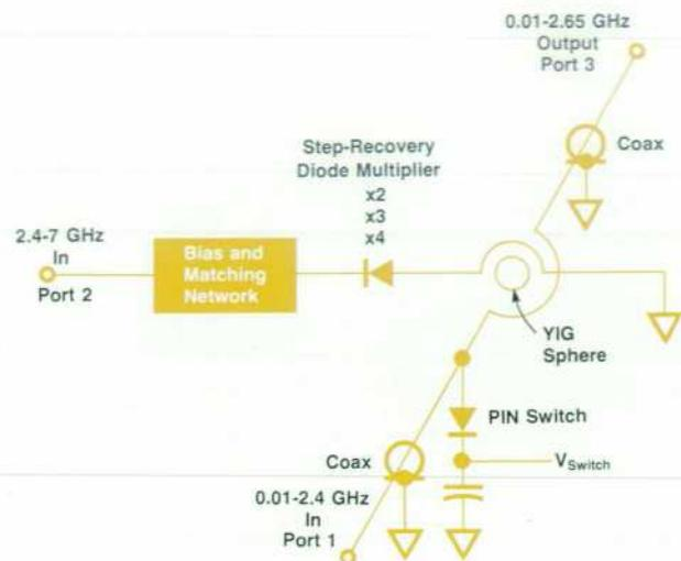
**Fig. 2.** Equivalent circuit of the SYTM.
