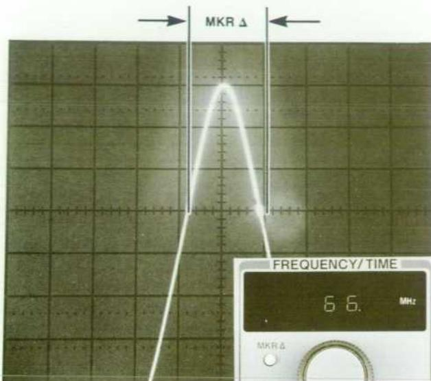
**Fig. 4.** Five independent, continuously variable markers identify significant frequencies. The marker difference function simplifies frequency bandwidth measurements as shown here. The frequency difference between any two of the five markers is displayed.
