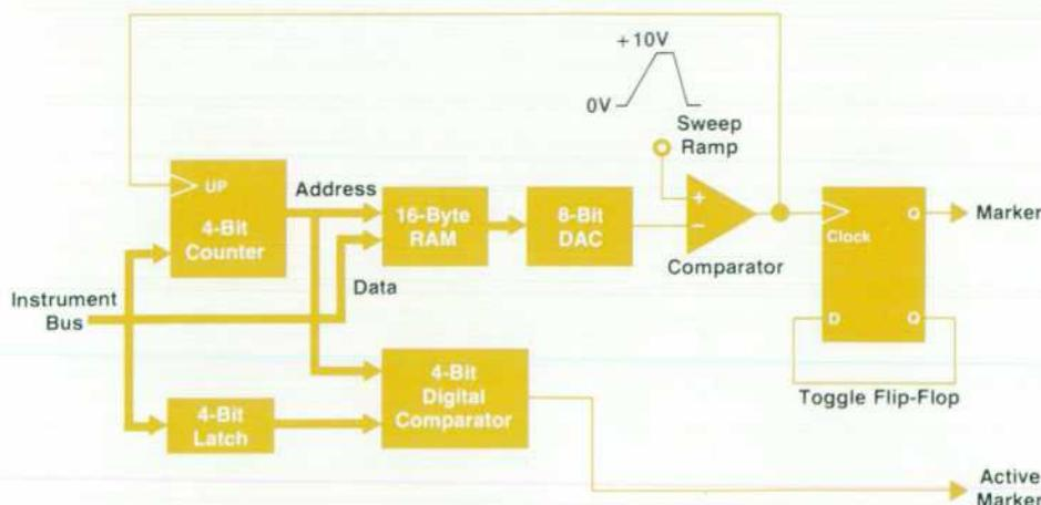
Fig. 11. Markers are generated by comparing the sweep ramp to the output of a DAC that has been loaded with the next marker frequency from a 16-byte RAM.
