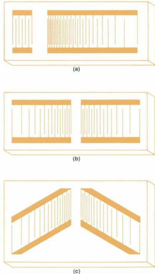
**Fig. 5.** Three SAW transducer configurations used to make dispersive (chirp) filters. (a) Broadband, nondispersive transducer on the right, dispersive transducer on the left. (b) Both transducers are dispersive and shorter than the long one in (a). (c) Slanted arrangement of transducers used in (b). This minimizes distortion caused by propagation under transducer electrodes.
