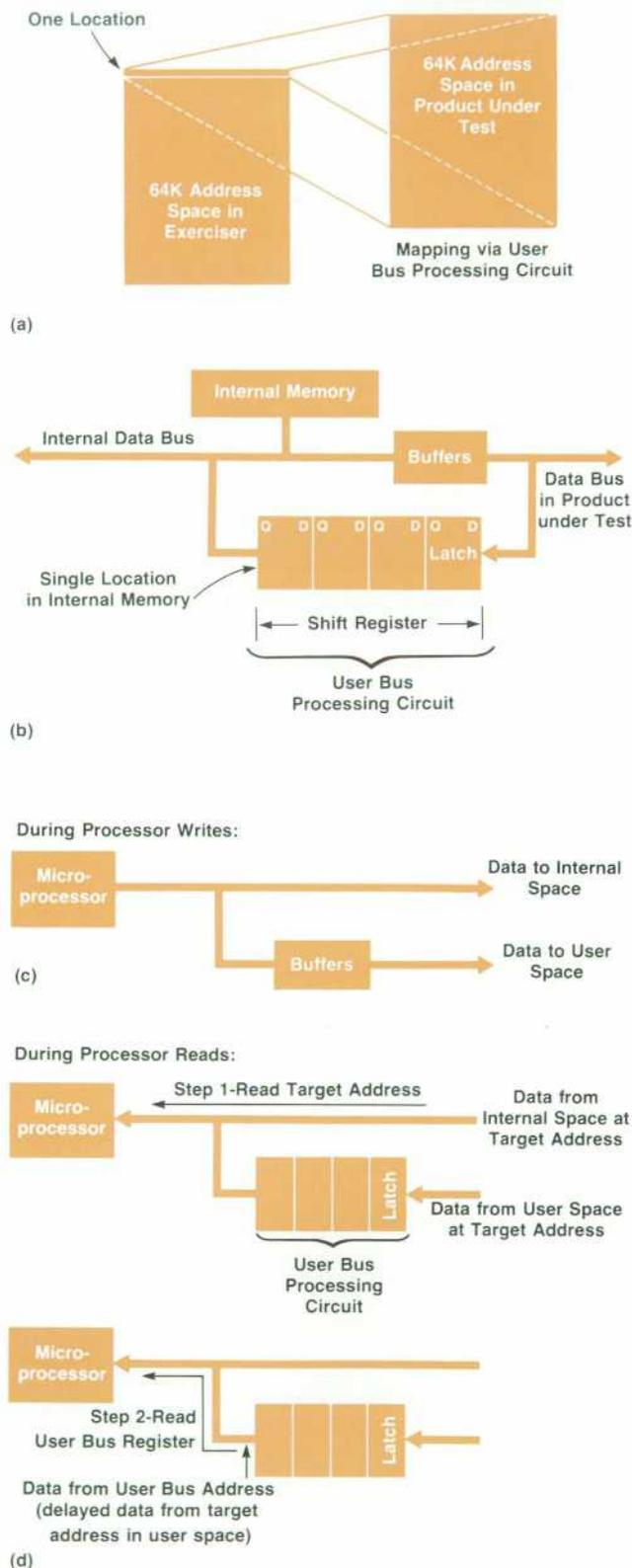
**Fig. 4.** The 5001A maintains a dual 64K address space by mapping the user space in the product under test into a single location in its internal memory. The user bus processing circuit delays responses from the user memory and the microprocessor reads the delayed data by reading the single internal memory location.
