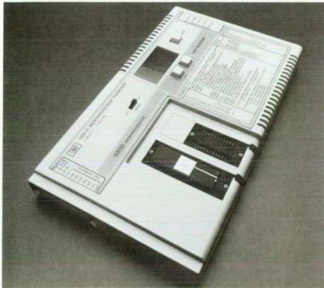
**Fig. 1.** Model 5001A Microprocessor Exerciser makes it possible to apply signature analysis troubleshooting techniques to 6800-microprocessor-based products not originally designed for signature analysis methods. Other versions (5001B,C,D) test products based on the 6802/6808, 8085A, and Z80A microprocessors.
