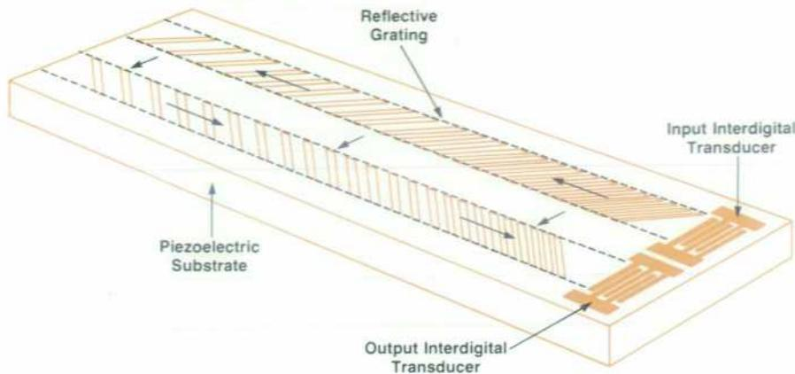
**Fig. 6.** Reflective array compressor. Here two broadband transducers are used for the input and output and dispersion is obtained from the variation in path length for different frequencies. The wave is reflected when the spacing in the direction of propagation is a wavelength  $\lambda$  (the period for adjacent grooves in the grating is about  $\lambda/\sqrt{2}$ ).
