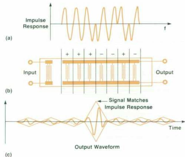
**Fig. 7.** SAW implementation of a seven-bit biphase-code correlator. An incoming signal is converted into a surface acoustic wave by the input transducer in (b) and propagates toward the output transducer. When the shape of the surface wave under the output transducer matches the impulse response of the transducer (a), a correlation pulse occurs at that time in the output waveform (c).
