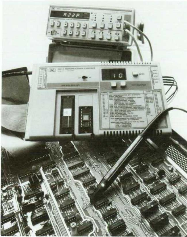
**Fig. 2.** To use the 5001A, the microprocessor in the product under test is removed from its socket and placed in the socket on the exerciser. The flat cable from the exerciser is connected to the vacant socket in the product. Four wires connect the exerciser to the signature analyzer, in this case the 5005A Signature Multimeter.
