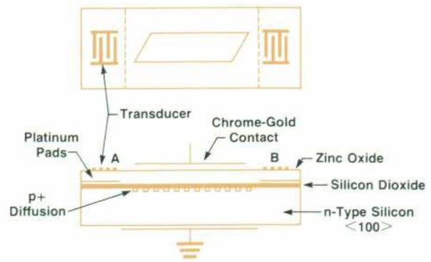
Fig. 9. Configuration of a monolithic diode storage correlator.
