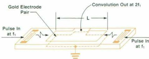
Fig. 8. Basic configuration for SAW elastic convolver.
