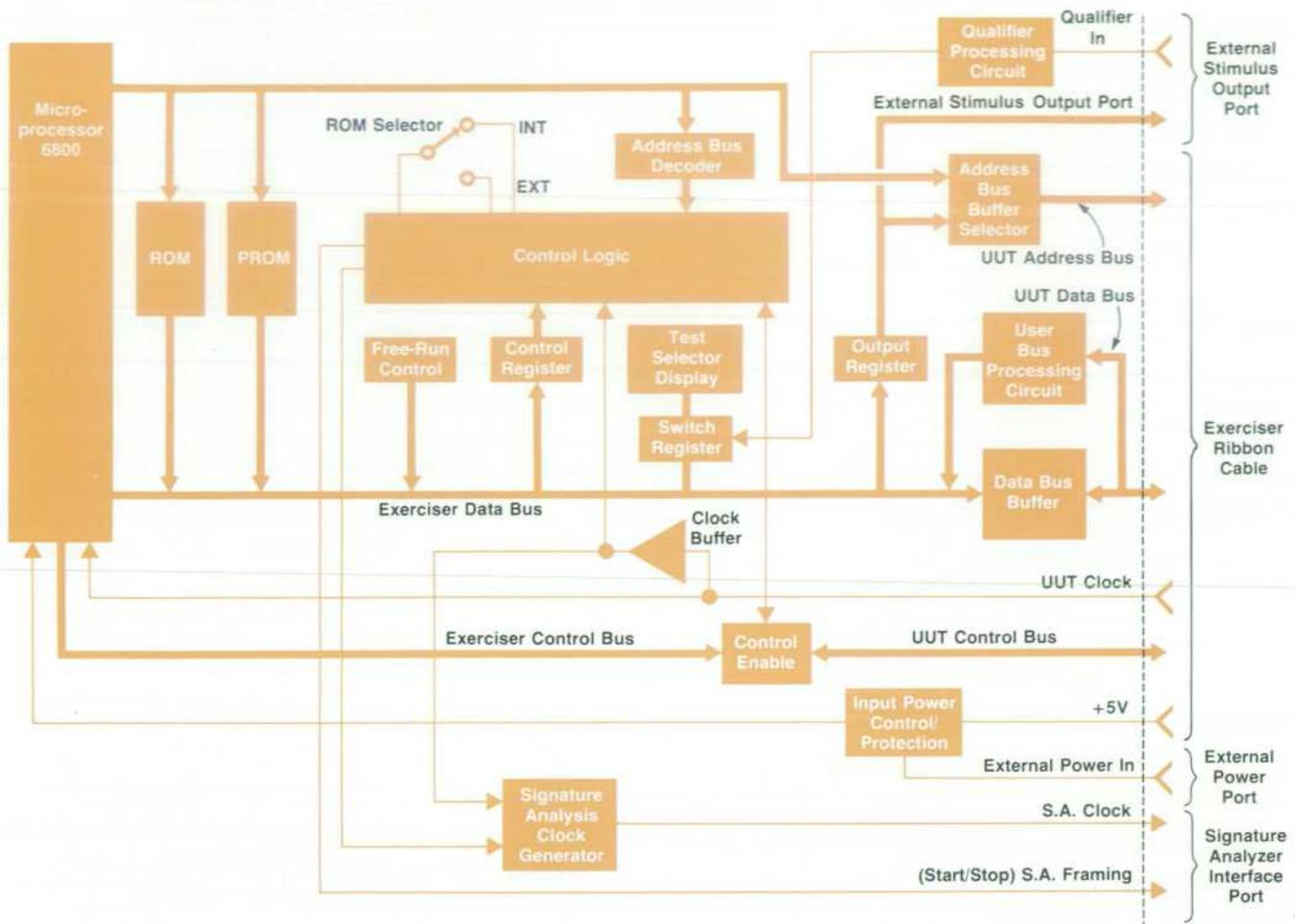
Fig. 3. Block diagram of 5001A Microprocessor Exerciser (UUT = unit under test).
