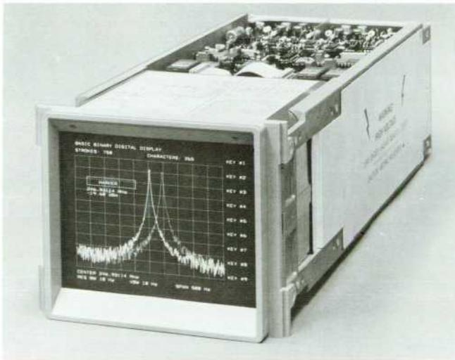
**Fig. 1.** Model 1345A Digital Display Module is a 16-cm (diagonal) electrostatic CRT display component for instrumentation and measurement systems. It has high resolution (2048 × 2048 points), internal character generation, and programmable intensity and line type.
