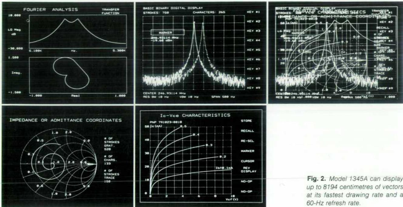
Fig. 2. Model 1345A can display up to 8194 centimetres of vectors at its fastest drawing rate and a 60-Hz refresh rate.
