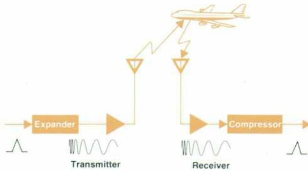
**Fig. 2.** SAW devices can be used in chirp radar systems by expanding a pulse before it is transmitted and compressing the received signal back into a narrow pulse so that distance accuracy is maintained. Expanding a pulse reduces the peak transmitter power required and pulse compression improves the signal-to-noise ratio in the receiver.
