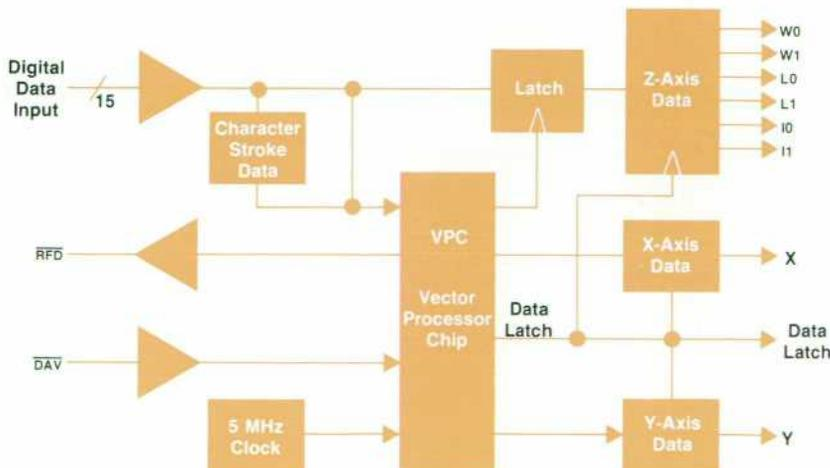
**Fig. 11.** The vector processor accepts input data and processes it for the stroke generator. The VPC is a special NMOS/CMOS integrated circuit chip.
