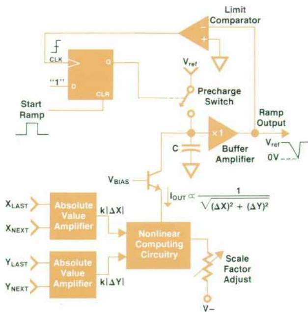
**Fig. 10.** The ramp generator keeps the writing beam velocity constant regardless of the length of the line being drawn. Thus all lines have the same intensity unless different intensities have been programmed.
