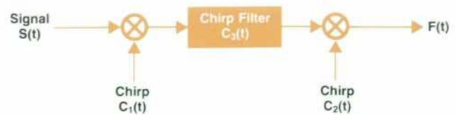
**Fig. 4.** Chirp filter implementation of analog Fourier transform. Chirps  $C_1(t)$  and  $C_2(t)$  can be generated by pulsing SAW chirp filters. The output  $F(t)$  is the Fourier transform of the signal  $S(t)$ .
