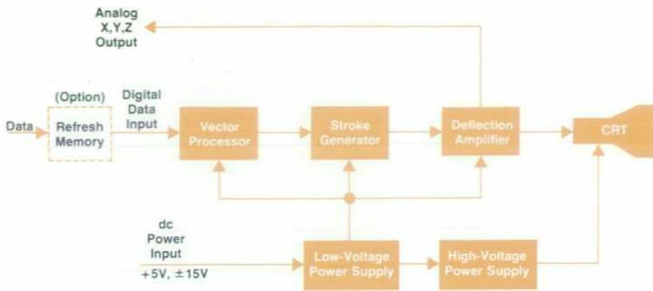
Fig. 8. 1345A block diagram.
