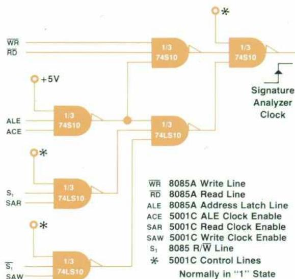
Fig. 3. 5001C signature analyzer clock generation.
