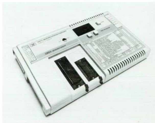
Fig. 5. 5001D Microprocessor Exerciser for Z80A-microprocessor-based products.
