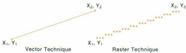
Fig. 4. Comparing vector and raster line-generation techniques.
