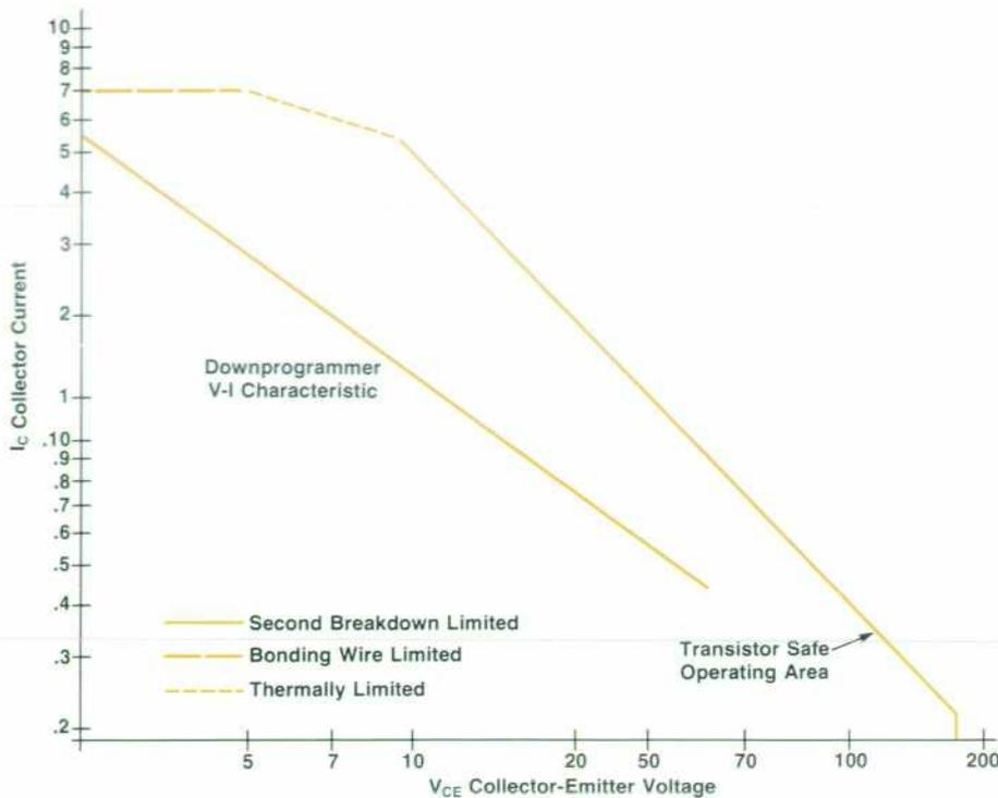
Fig. 6. A downprogrammer with this negative resistance characteristic makes it possible to decrease the output voltage rapidly in automatic test and industrial process control applications.
