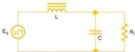
**Fig. 2** This simplified circuit illustrates the voltage regulation technique used in the 65000A Series Power Supplies. The tank circuit converts the square wave to sine waves as an integral part of the technique. See Fig. 3.
