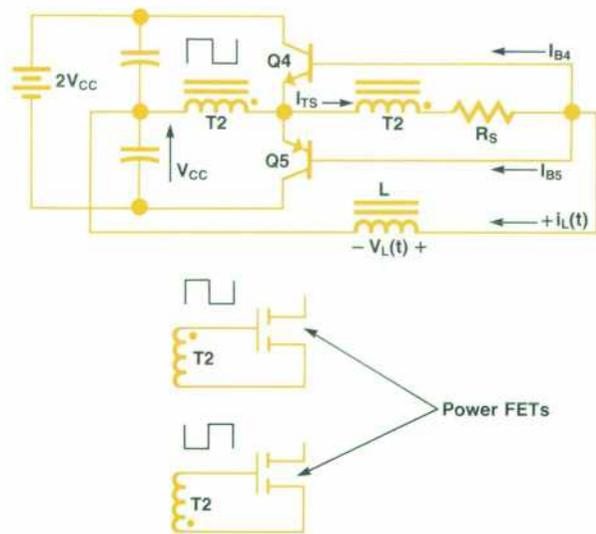
Fig. 5. High-current voltage-controlled oscillator (VCO) provides more than one ampere to drive the power MOSFETs, using only eight components.  $L$  is a variable control inductor; the oscillator frequency is controlled by varying the inductance of  $L$ .
