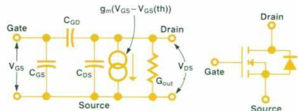
Fig. 8. Small-signal equivalent circuit for the power MOSFET.
