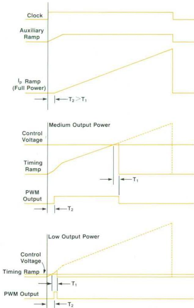
**Fig. 5.** An auxiliary timing ramp added to the primary timing ramp takes effect at low output power so that very narrow, yet controlled pulse widths are produced by the pulse-width modulator (PWM) that switches the MOSFETs on and off. This allows efficient operation at combinations of low output voltage and current.
