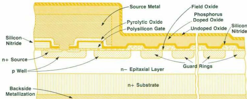
**Fig. 6.** Cross section of the HP vertical power MOSFET showing the guard-ring structure on the right. This structure distributes the electric fields at and near the top surface to maintain a high voltage breakdown capability.
