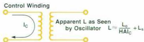
Fig. 7. Simplified schematic of the variable control inductor shown in Fig. 5.
