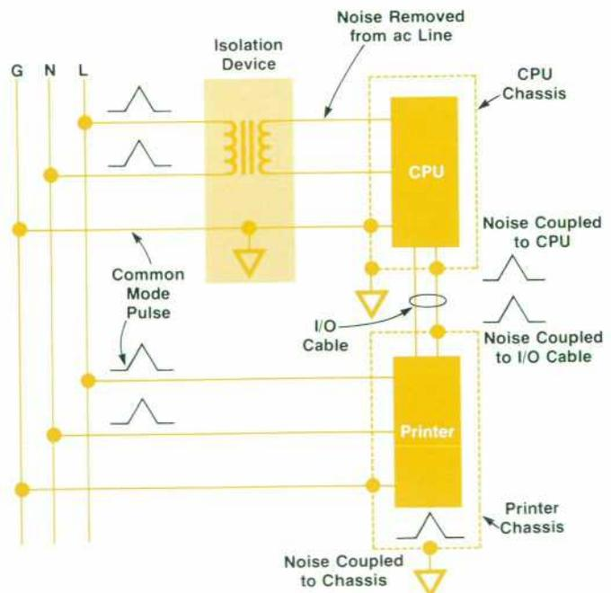
Fig. 3. All units in a computer system must be isolated from the ac power line. Otherwise, an unisolated unit, the printer shown here, can couple noise to an isolated unit, the CPU here, via the I/O interconnections.
