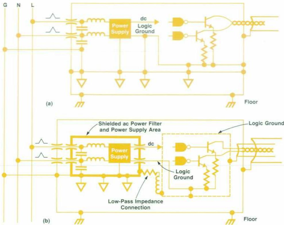
**Fig. 5.** Two grounding approaches can be used to increase immunity to line transients. (a) Common safety and logic grounds. Transient energy is uniformly distributed throughout the chassis so that no noise potentials exist between the internal circuits. (b) Isolated safety and logic grounds. Transient energy is tightly coupled to the chassis, but the internal circuits are isolated with respect to the chassis by a low-pass filter.
