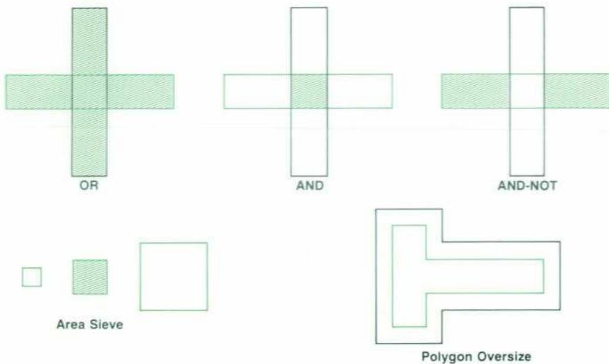
Fig. 3. Design rule checking (DRC) operations.
