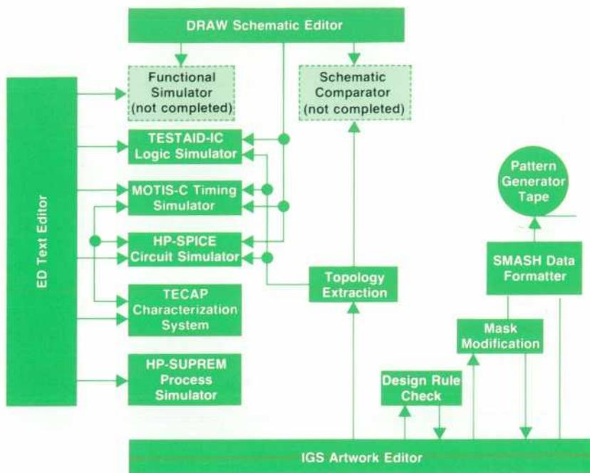
Fig. 1. Hewlett-Packard design aids for integrated circuit design.
