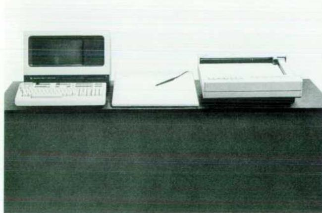
**Fig. 1.** DRAW circuit design station consists of an interactive graphics terminal, a digitizing tablet, and a four-color plotter, all tied to a timeshared computer. DRAW is a graphics editor designed for editing schematics.
