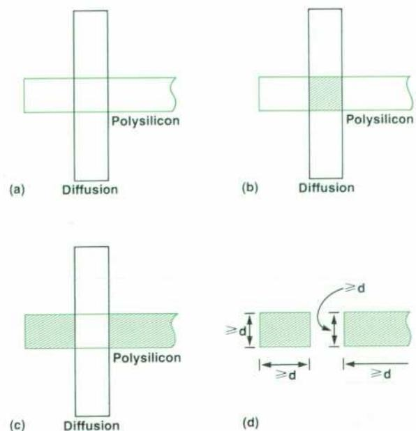
Fig. 5. An example of rule isolation and test. One design rule for an NMOS transistor gate is that polysilicon must overlap diffusion by a distance  $d$ . (a) Original artwork. (b) Polysilicon is ANDed with diffusion to create the active area. (c) Polysilicon is AND-NOTed with the active area to create the nonactive polysilicon. (d) The internal width of the nonactive polysilicon is tested to be sure that it exceeds the minimum  $d$ .
