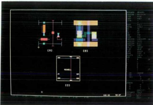
Fig. 6. Stick, detailed, and block symbolic views of a shift register cell, produced using the SYMBOL and DETAIL macrocommands.
