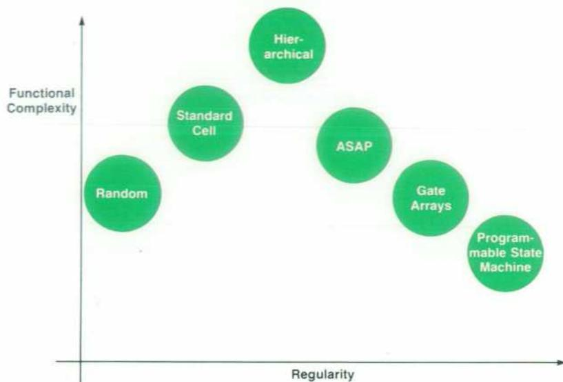
Fig. 2. Six different IC design methodologies (circled areas) are used at Hewlett-Packard, depending on the functional complexity and regularity of the circuit being designed.
