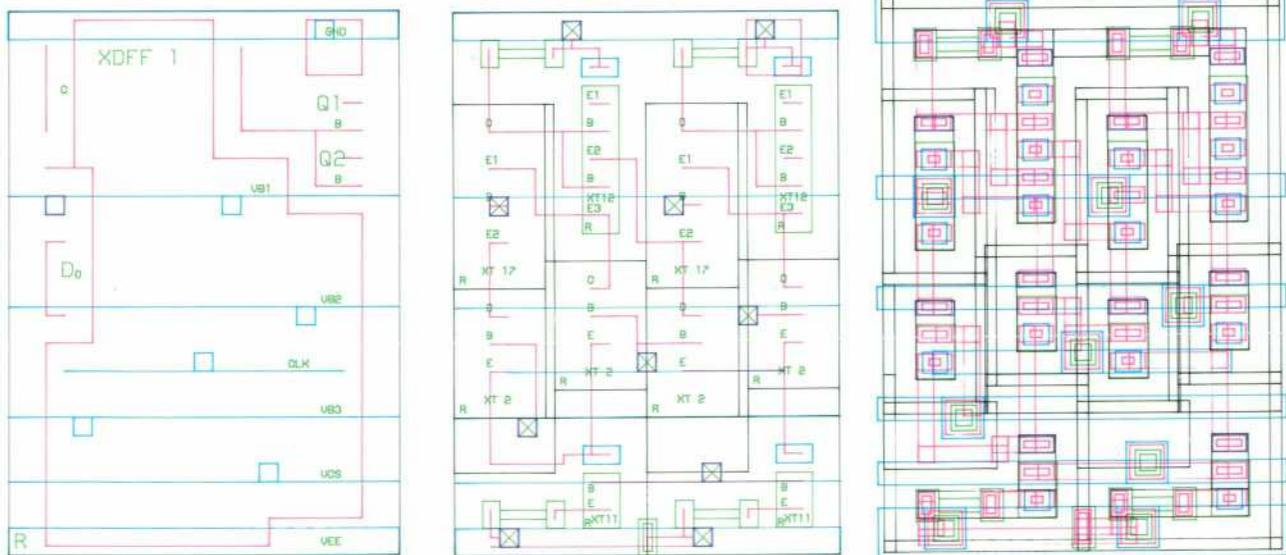
Fig. 2. The ASAP design starts with the simple symbols on the far left and progresses to a more detailed symbolic representation which is translated into the geometrical layout used to fabricate the circuit shown on the far right.
