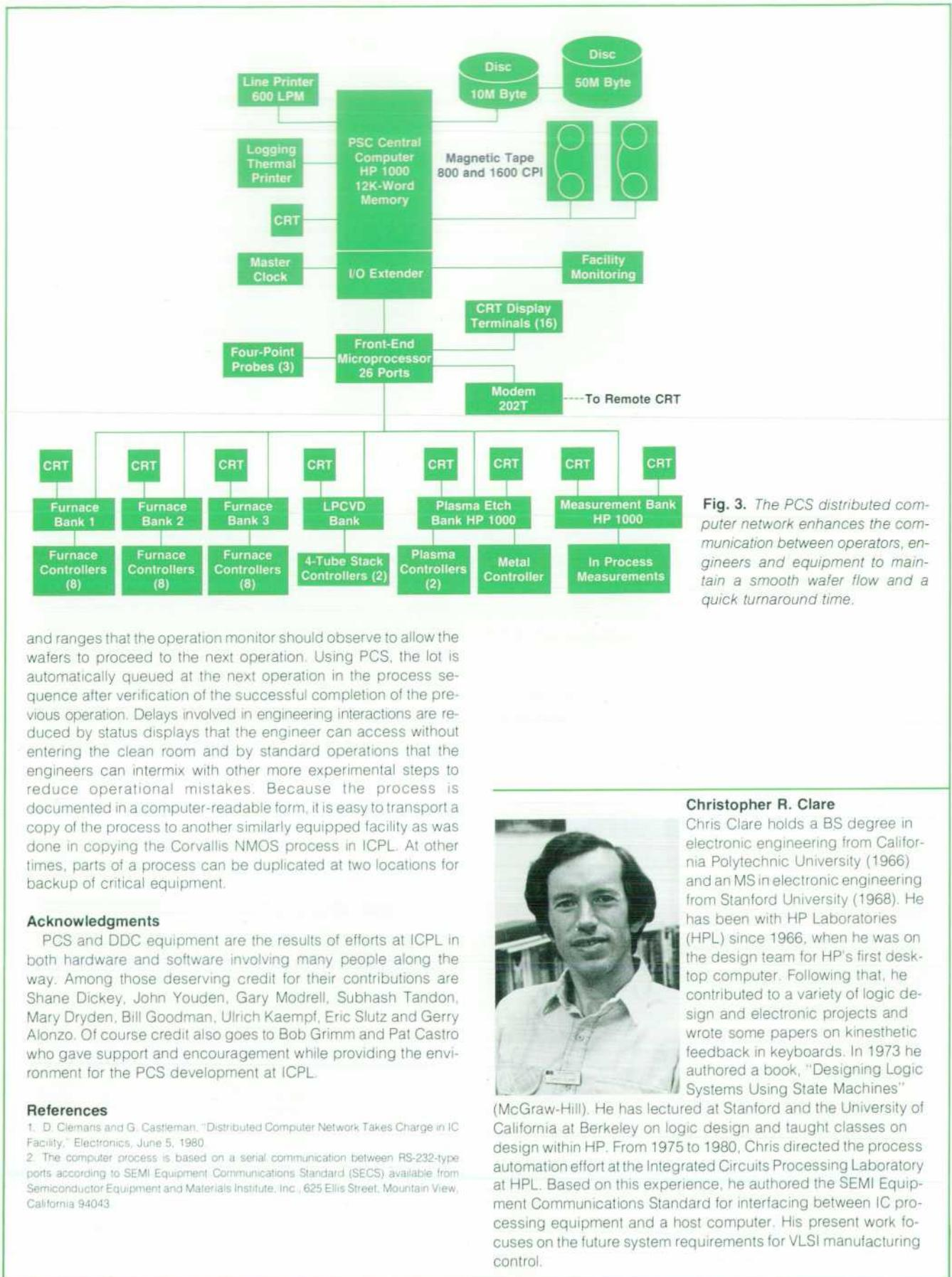
**Fig. 3.** The PCS distributed computer network enhances the communication between operators, engineers and equipment to maintain a smooth wafer flow and a quick turnaround time.
