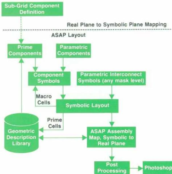
Fig. 1. Flow diagram of the symbolic layout process.
