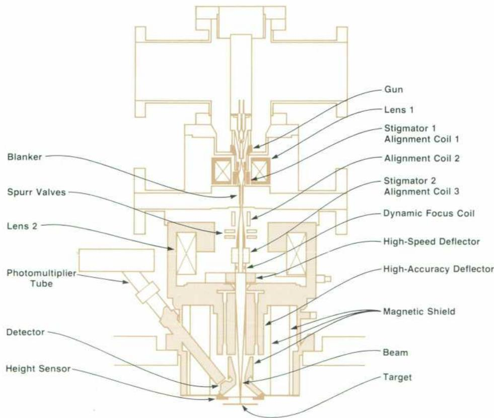
**Fig. 1.** Column design for the HP electron beam lithography system uses two magnetic lenses, electrostatic beam blanking, and a field-emission cathode. The electron gun assembly can be removed from the system for servicing without exposing the lower deflection system to the atmosphere.
