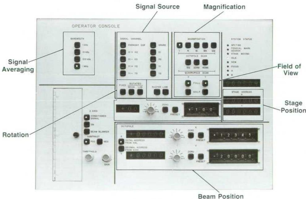
Fig. 1. The operator panel of the HP electron beam lithography system.
