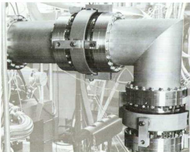
**Fig. 3.** Several of these assemblies are used in the vacuum line from the main cryogenic vacuum pump and the electron beam system to isolate the vibration caused by the pump. The U-joint design protects the bellows inside from distortion and collapse caused by atmospheric pressure and mechanical misalignment.
