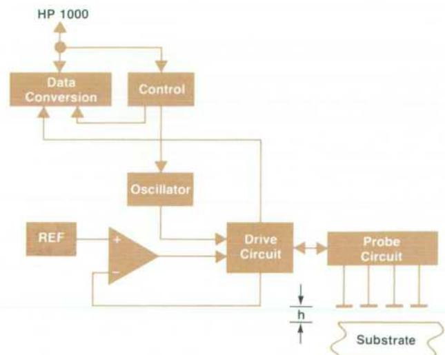
**Fig. 8.** The height sensor system measures the height of the substrate within a few tenths of a micrometre.
