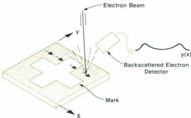
**Fig. 1.** The signal for detecting the fiducial mark is generated by scanning the electron beam through the vicinity of the mark and detecting the number of electrons backscattered from the mark and its substrate.
