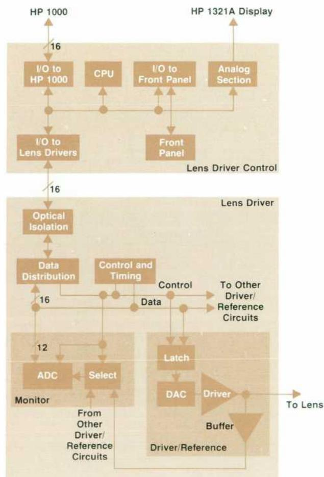
Fig. 6. The lens driver and control subsystem provides a focusing system for the electron beam.
