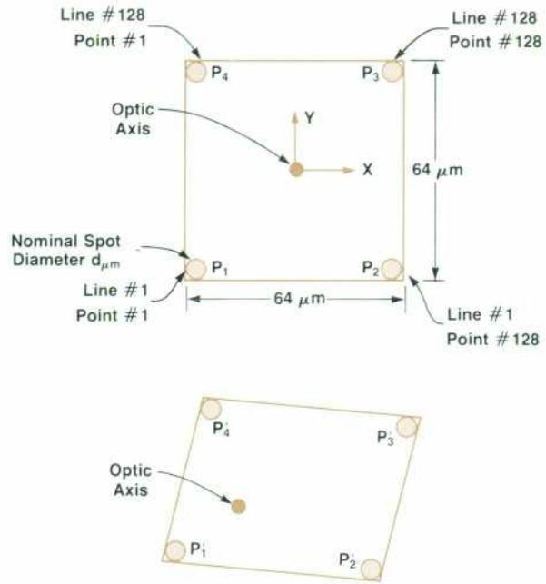
**Fig. 5.** If the quadrupole is calibrated, four points, one in each corner of the raster scan, will define a square centered about the optic axis as shown in (a). However, if the quadrupole is uncalibrated, the same four points will define a parallelogram whose center is offset from the optic axis as shown in (b).
