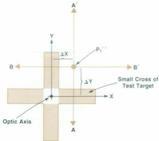
**Fig. 6.** When the beam is deflected from  $P_1$  in Fig. 5 to a position near the optic axis (center of the fiducial mark), the error ( $\Delta x$ ,  $\Delta y$ ) between its actual position  $P_1''$  and the optic axis can be measured by scanning the beam across the mark along A-A' and B-B'.
