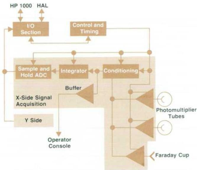
**Fig. 7.** The fiducial mark system conditions signals from photomultiplier tubes or a Faraday cup within the column. The system computers use the conditioned signals to detect fiducial marks on the substrates so that the substrates can be precisely located.
