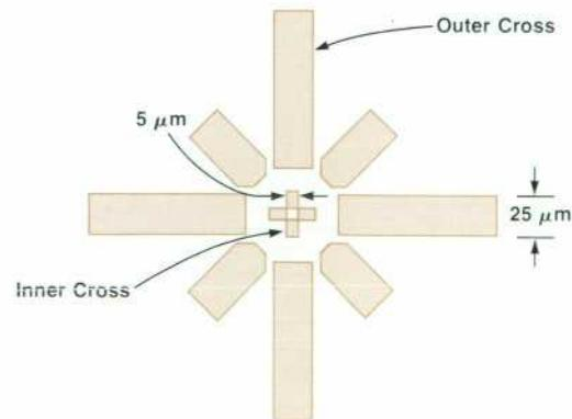
**Fig. 2.** Individual pattern on calibration plate. The outer cross is used for coarse beam position measurements and the small inner cross is used for X-Y stage calibration and for fine beam position measurements. The octagonal arrangement is used for measuring the beam shape.
