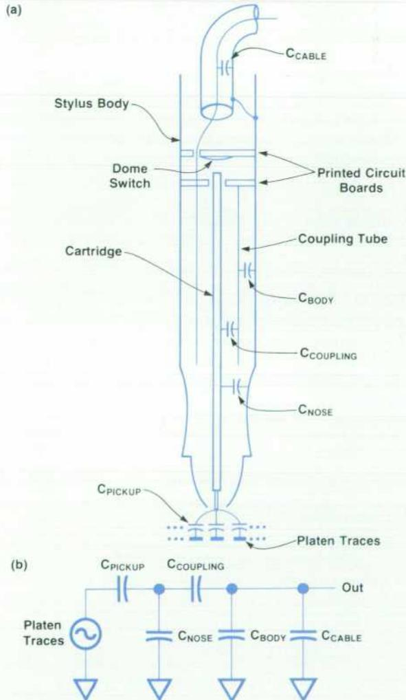
**Fig. 1.** Design of capacitively coupled stylus for the 9111A. (a) Cross-sectional view showing the conductors and capacitive components. The stylus cartridge can be replaced by an ink-filled cartridge for users drawing images instead of tracing them. (b) Equivalent circuit for the stylus signal path from the platen traces to the instrument.
