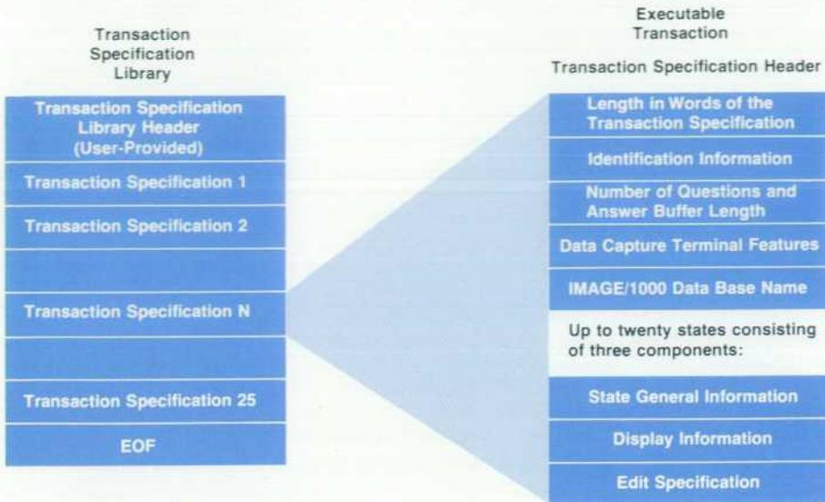
**Fig. 9.** Each transaction specification in the TS library consists of a transaction header followed by up to 20 states consisting of three components each.
