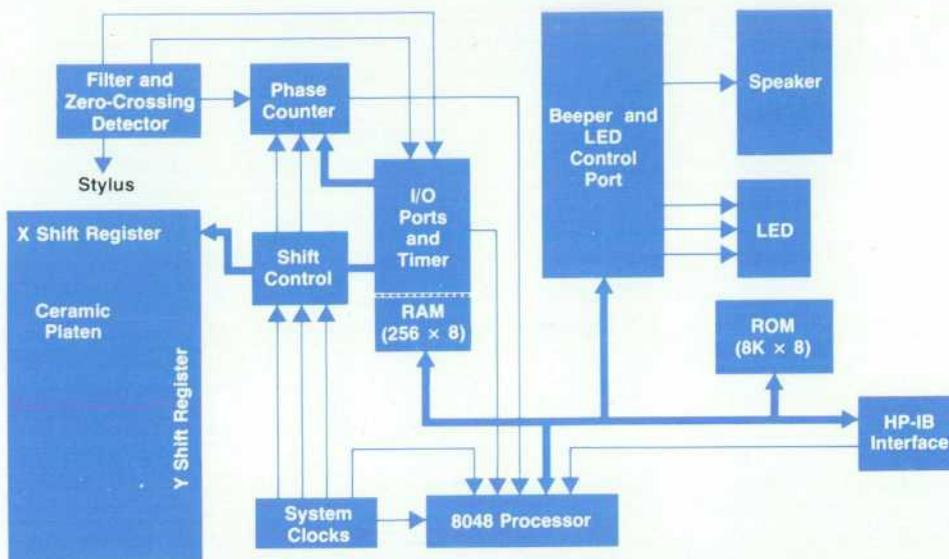
**Fig. 2.** 9111A system block diagram. The microprocessor in the system controls the interface functions, selects measurement modes, tests the system, and communicates with the host computer in addition to computing the position of the stylus.
