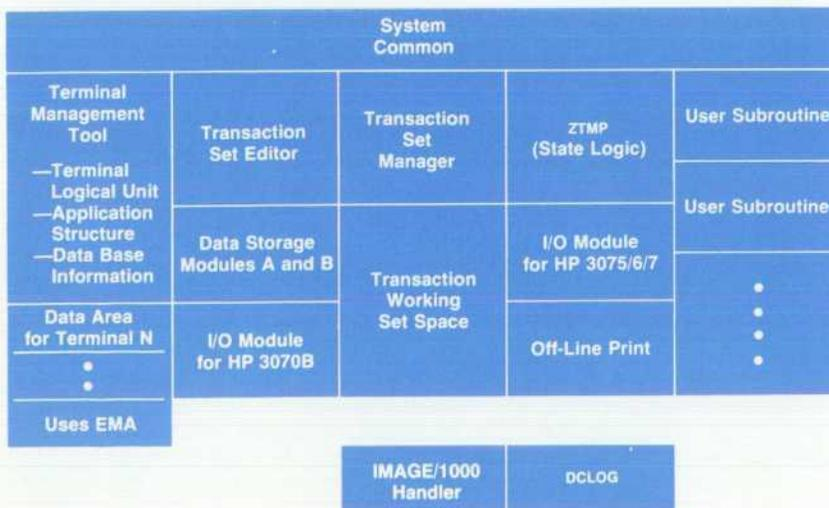
**Fig. 10.** Once it has all of the answers it needs, the transaction monitor program generator generates the relocatable members of DATACAP/1000 and calls the RTE-IVB loader to relocate them into the memory structure shown here.
