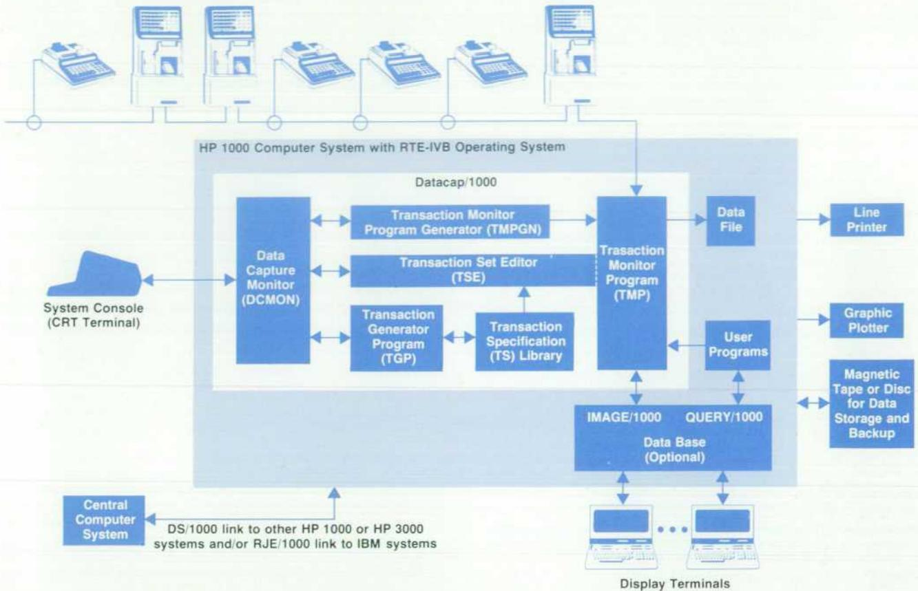
**Fig. 3.** Major components of DATACAP/1000. The transaction generator program (TGP) and transaction monitor program generator (TMPGN) interactively lead the user through the process of building transaction specifications and the transaction monitor program (TMP). The TMP then manages the collection of factory data and creates data files or enters the data into the IMAGE/1000 data base, if present.
