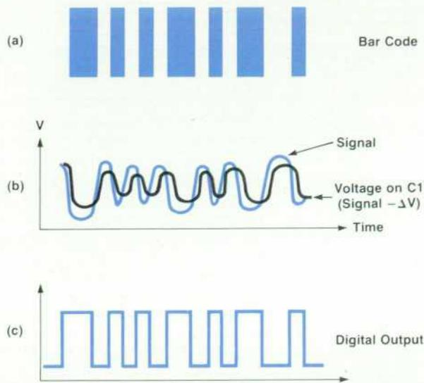
**Fig. 7.** Operation of the processing circuit in the HEDS-3000. When the bar code in (a) is scanned, peak detection converts the resulting voltage across C1 (b) into a logic-compatible signal (c). Note:  $\Delta V$  = diode forward voltage drop.
