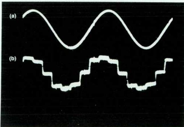
**Fig. 3.** Stylus signals after (a) and before (b) bandpass filtering. The lower trace shows the stairstep waveform resulting from the summation of the signals from each of the platen traces.
