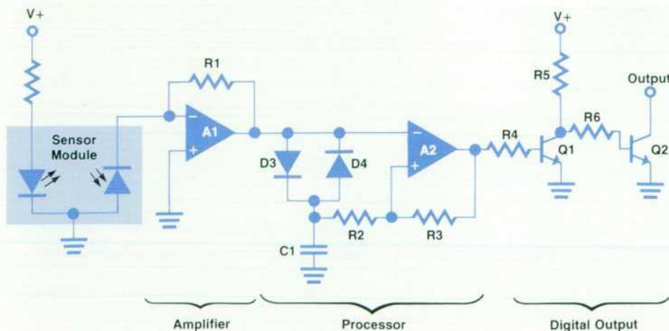
Fig. 6. Circuit schematic for the HEDS-3000.
