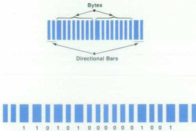
Fig. 3. Basic format for bar codes read by the 82153A Wand in the HP-41C Calculator system.
