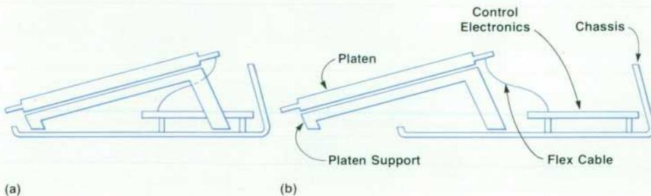
**Fig. 6.** The 9111A hardware design allows service personnel to easily open the unit for servicing and still maintain normal operating functions. (a) Normal operating configuration. (b) Open for servicing.
