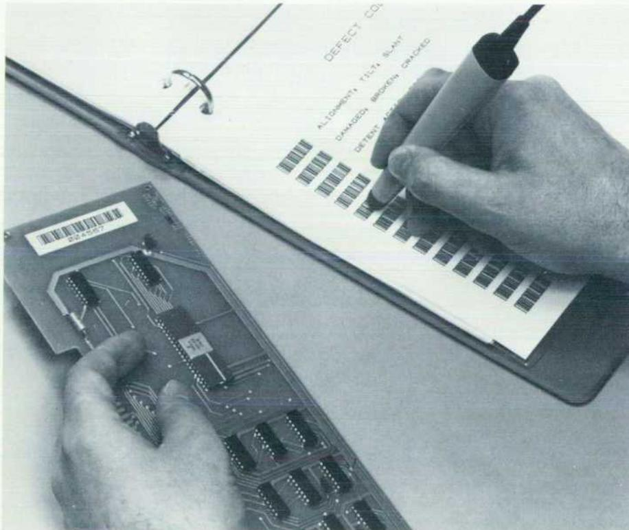
**Fig. 2.** In this industrial application each assembly is identified by bar code and the QA defect code is read directly by a bar code wand from a code index, eliminating copying errors.
