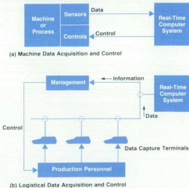
**Fig. 1.** DATACAP/1000 is a software package for HP1000 Computer systems. It collects factory data such as time and attendance, work in process, inventory, and test statistics, and presents it to management. It is a system for logistical data acquisition and control (b) rather than the more familiar form of factory automation shown in (a).
