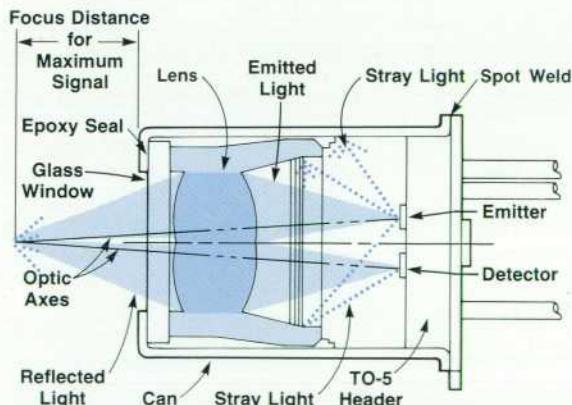
**Fig. 2.** The HEDS-1000 High-Resolution Reflectance Sensor used in the HEDS-3000 is also available as a separate product. This sensor contains both an emitter and detector in a single package. A bifurcated lens design focuses the light from the sensor's emitter onto the area to be sensed and focuses the reflected light back onto the detector area in the sensor.
