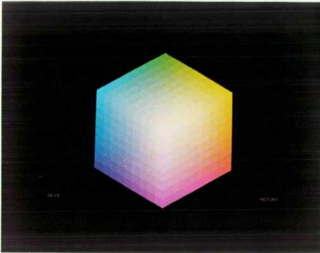
**Fig. 1.** Color cube model. Area-fill colors can be specified by selecting a point within this unit cube. The three coordinates for the point indicate the fractions of red, blue, and green required for the specified color.
