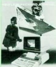
System 45 is Hewlett-Packard's most powerful desktop computer—the top of the line. Born in 1977 as System 45A, it gives engineers and scientists a single compact unit that contains all the elements needed to solve complex design and analytical problems. It has an interactive keyboard, a large memory, a graphic display, two fast processors, a line printer, and dual magnetic tape drives. Standard computer peripherals such as disc drives and plotters can be added if their capabilities are needed.
