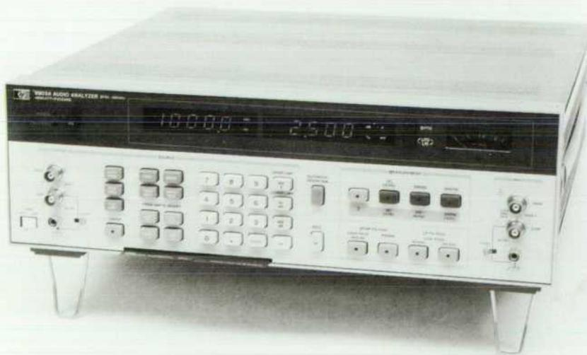
**Fig. 1.** Model 8903A Audio Analyzer makes the accurate measurements needed to characterize systems and signals in its frequency range of 20 Hz to 100 kHz. It has applications in general audio testing, transceiver testing, and automatic systems. Microprocessor control makes it automatic and easy to use.
