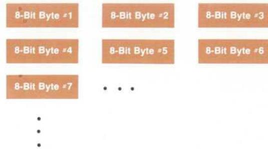
**Fig. 5.** Data display using triple probing. A threefold increase in frequency can be obtained in this way, at the expense of narrowing the effective analyzer word width.
