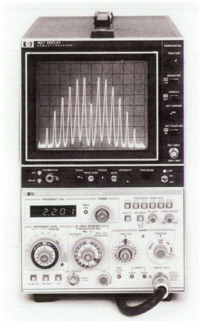
**Fig. 1.** The Model 8559A Spectrum Analyzer, shown here mounted in a Model 182T large-screen display, covers a frequency range of 0.01 to 21 GHz with accuracy and sensitivity characteristic of a lab-grade analyzer. Its size and weight make it suitable for field use.
