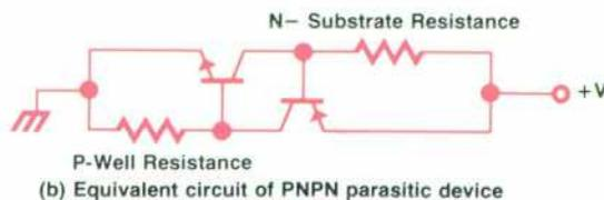
(b) Equivalent circuit of PNP parasitic device
