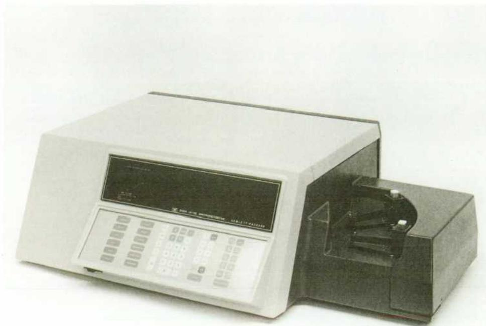
**Fig. 2.** Model 8450A UV/Visible Spectrophotometer is designed to overcome many of the limitations of traditional spectrophotometers and provide chemical information that formerly had to be ignored. A high degree of integration between its processor, optics, and keyboard helps maximize its speed, accuracy, sensitivity, and productivity.
