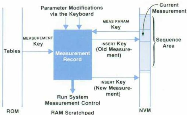
Fig. 3. The keyboard can be used to select, modify, and run measurements either from the sequence area or fresh from the tables. New measurements may be added to the sequence or existing ones modified.
