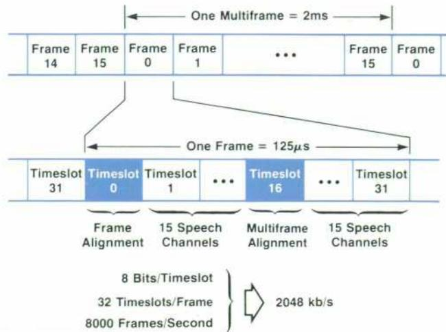
**Fig. 3.** The European 30-channel system uses a frame alignment signal in time slot 0 to identify each speech channel, and a multiframe alignment signal in time slot 16 to allow signaling information associated with each channel to be distributed throughout a 16-frame multiframe. The 3779A is designed to interface with this system.
