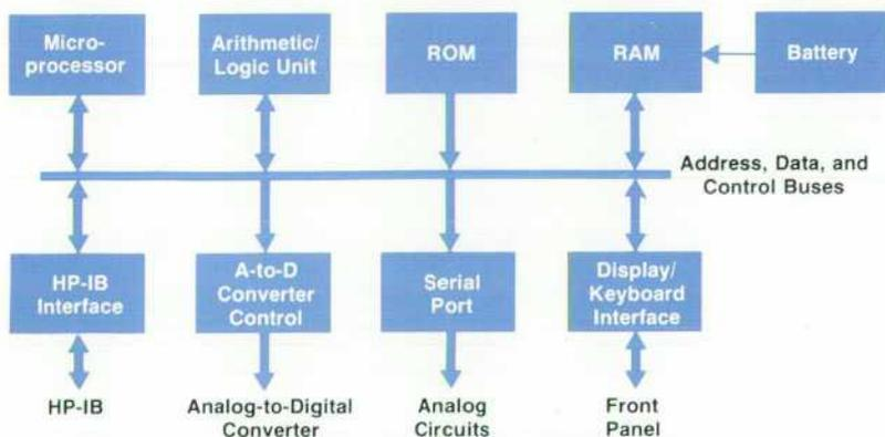
Fig. 9. 4191A digital section. An M6800 microprocessor manages all operations.
