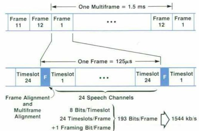
**Fig. 4.** In the North American 24-channel system, frame alignment and multiframe alignment information (more commonly referred to as terminal framing,  $F_T$ , and signaling framing,  $F_S$ ) are both carried in a one-bit-per-frame sequence. Signaling information can be accommodated by stealing one bit per channel every 6th frame. The 3779B has been developed for this system.
