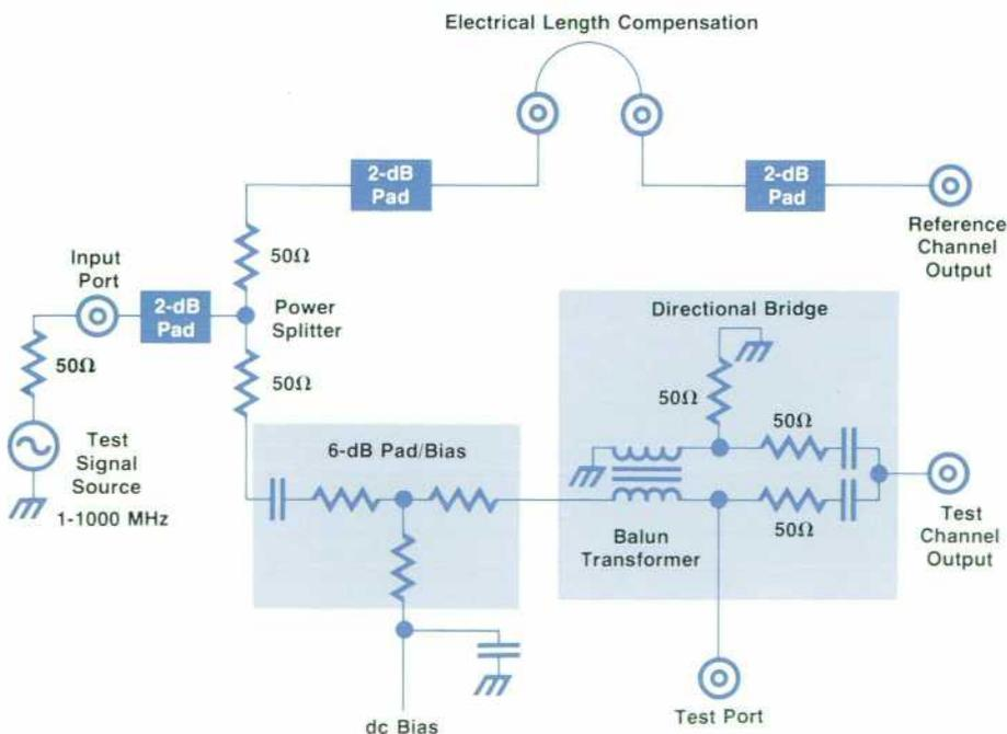
Fig. 5. RF bridge section of the 4191A Impedance Analyzer.
