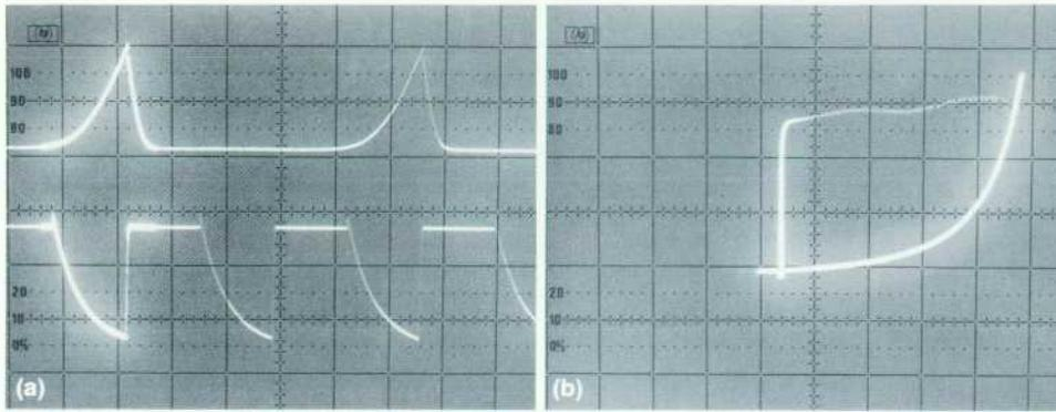
**Fig. 3.** Use of the delayed sweep intensity gate (brightened segments) while the oscilloscope is in the main intensified mode enables the operator to "window" the portion of the waveforms to be examined (a). Switching to the delayed sweep and A-vs-B mode causes an X-Y plot to be traced by the windowed portions while the remaining parts of the waveforms are blanked out (b).
