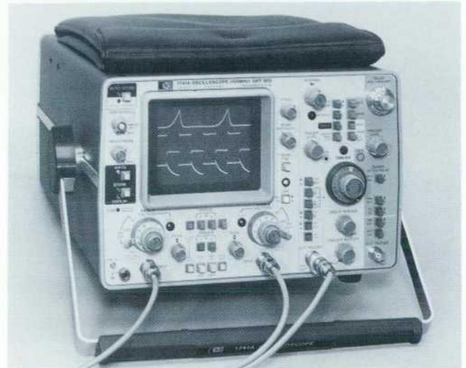
**Fig. 1.** Model 1741A is a portable, laboratory-grade, dual-trace 100-MHz oscilloscope that has variable-persistence and storage modes of operation with a writing rate of  $>100$  cm/ $\mu$ s. The most sensitive deflection factor is 5 mV/div, expandable to 1 mV/div on both channels simultaneously (with a reduction in bandwidth to 30 MHz). An external waveform used for triggering the sweep may be displayed on a third trace to assist the operator in selecting the trigger point.
