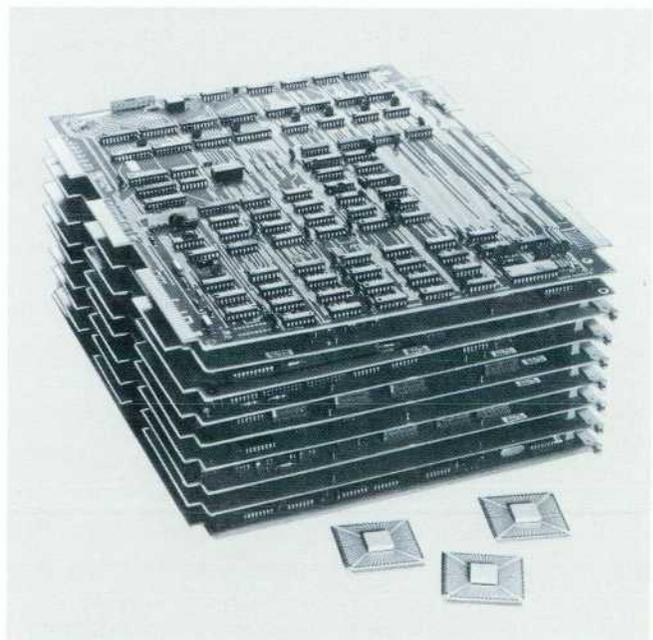
**Fig. 3.** Silicon-on-sapphire technology makes the Series 33 possible, reducing 4500 cm<sup>2</sup> of HP 3000 components on portions of nine circuit boards to the three SOS chips in the foreground.
