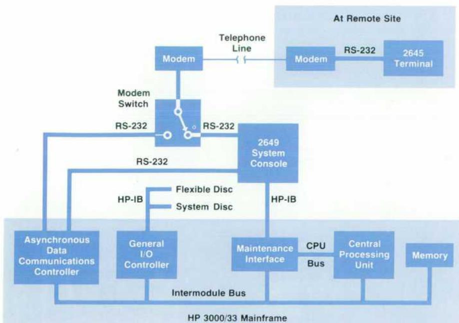
**Fig. 1.** HP 3000 Series 33 maintenance hardware includes the system console, a remote console, and the maintenance interface. The MI provides access to the CPU and the intermodule bus.
