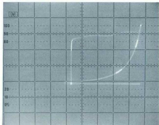
**Fig. 5.** Use of the delayed sweep intensity gate while making A-vs-B plots with the main sweep trigger enables the direction of time to be determined (see text), as illustrated by this triple-exposure photograph that shows the delayed sweep intensity gate in three different positions.
