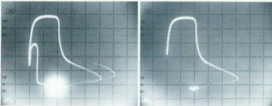
**Fig. 4.** The photo at left is a plot of collector current versus collector-emitter voltage in the switching transistor of a dc-to-dc inverter during the first 100  $\mu$ s of operation following turn on. In the photo at right, the delayed sweep is used in the A-vs-B mode to window a 2- $\mu$ s portion of the plot thereby showing that the high-power portion of the plot is of sufficiently short duration.
