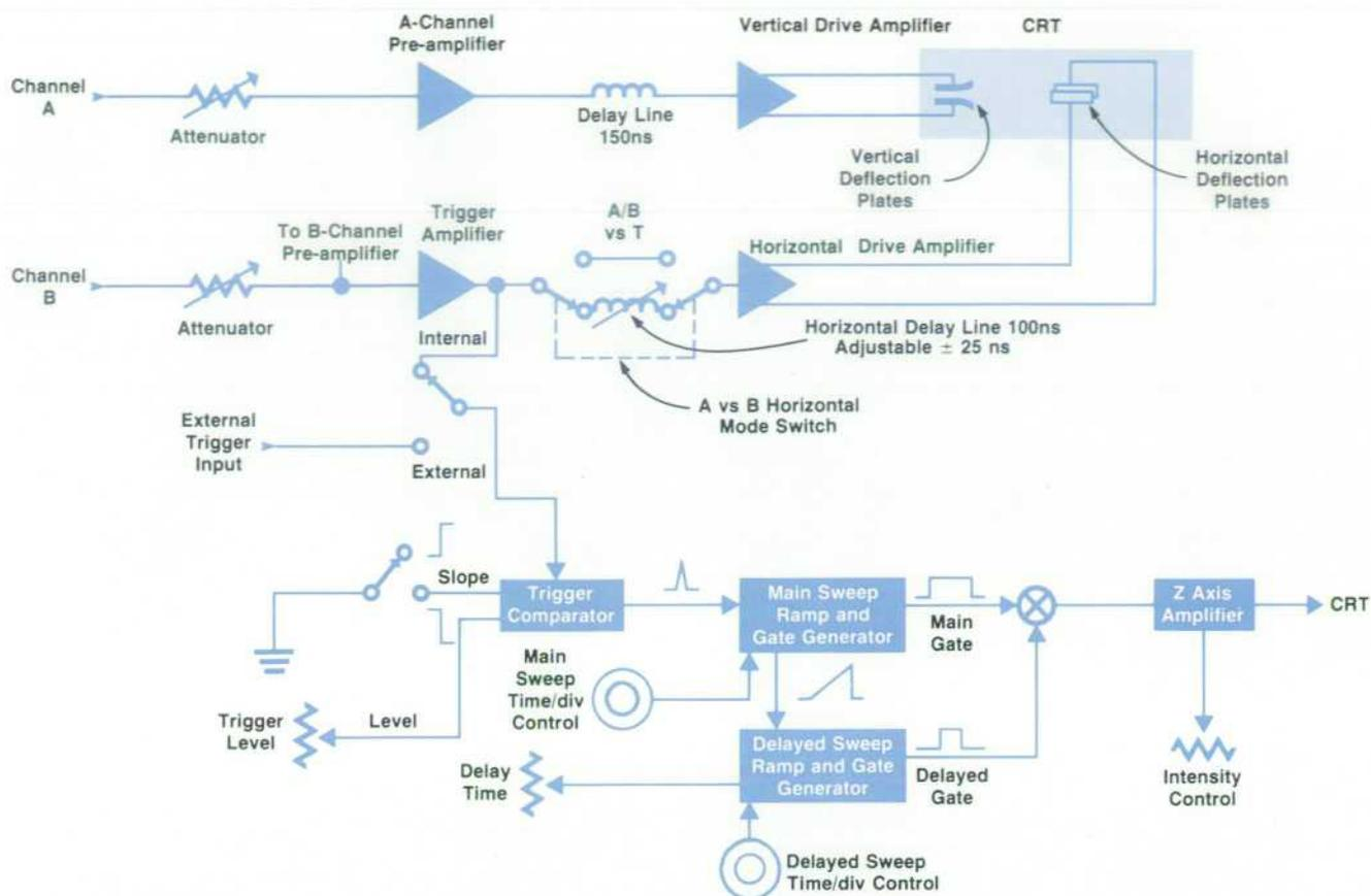
Fig. 6. Circuits pertinent to the triggered A-vs-B mode.
