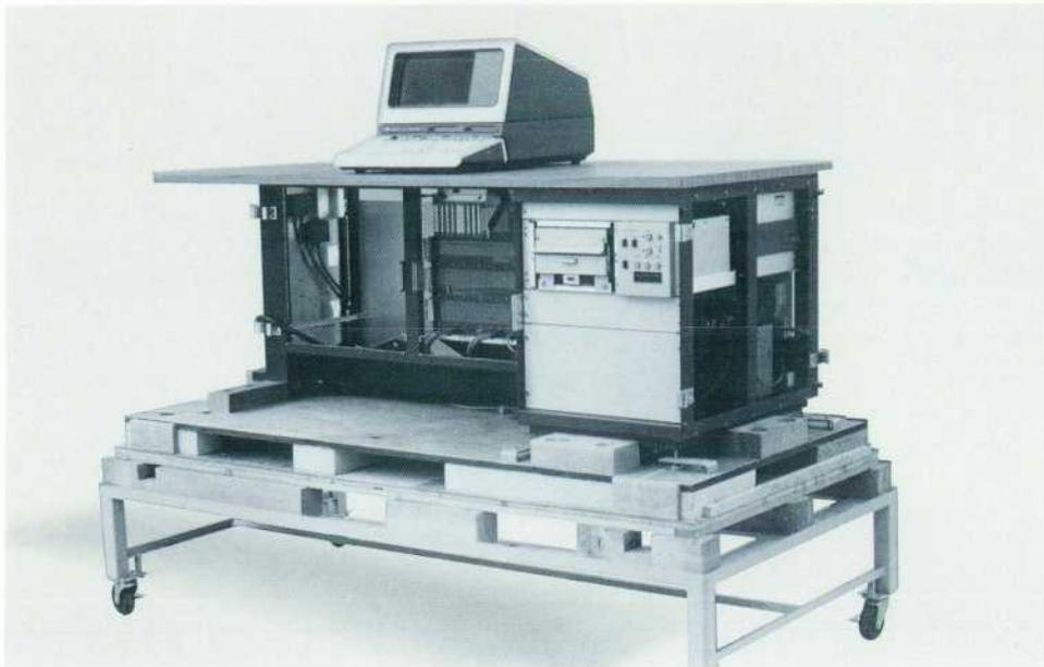
**Fig. 2.** Series 33 mainframe is mounted on a wooden pallet and placed on an elevated pedestal for ease of handling and assembly on the production floor. After final system assembly, the same pallet is used as the base for the shipping container.
